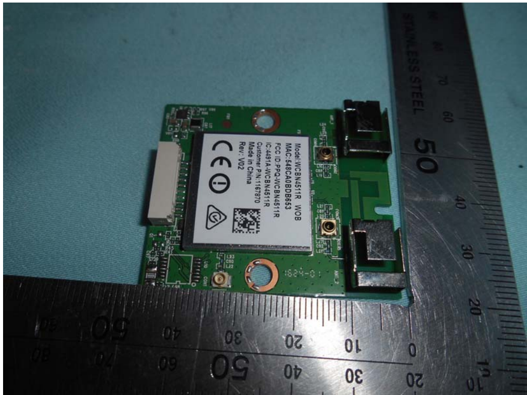
FIGURE 19 LED LCD TV (M/N: 43H7C) RF BOARD (COMPONENT SIDE)
