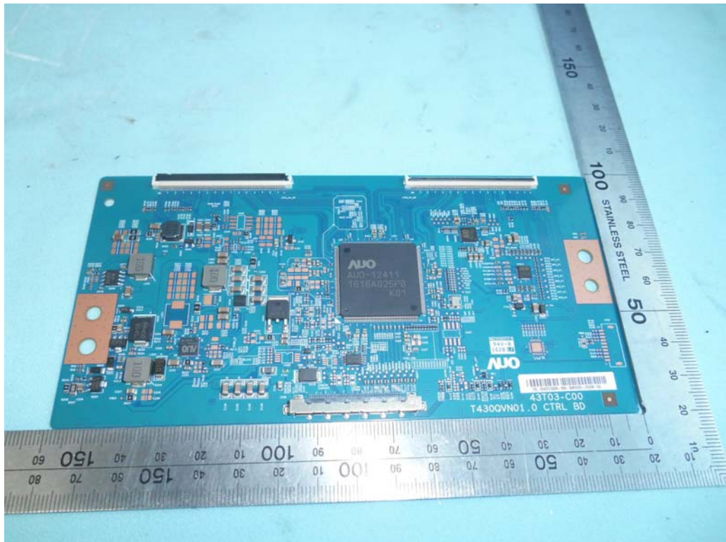
FIGURE 12 LED LCD TV (M/N: 43H7C) PANEL BOARD (COMPONENT SIDE)
