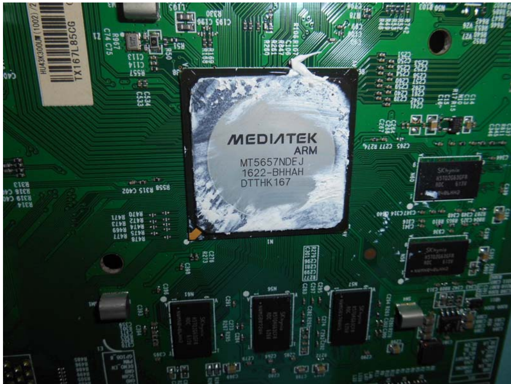
FIGURE 7 LED LCD TV (M/N: 43H7C) CHIP & CRYSTAL ON MAIN BOARD
