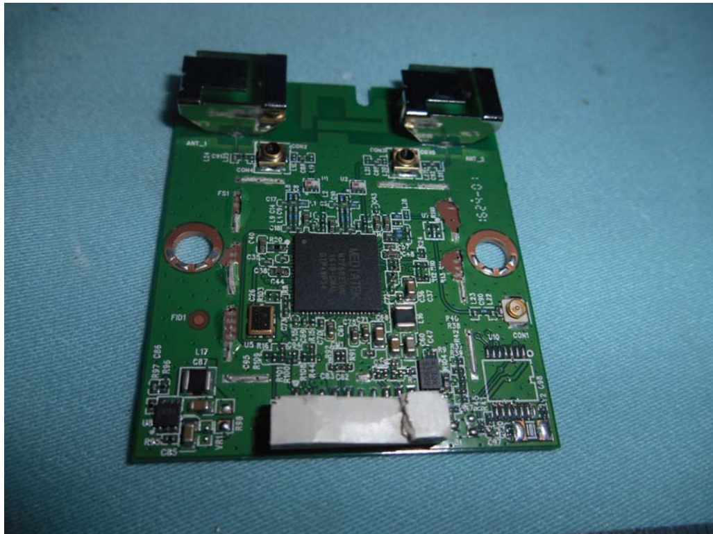
FIGURE 22 LED LCD TV (M/N: 43H7C) CHIP AND CRYSTAL ON RF BOARD
