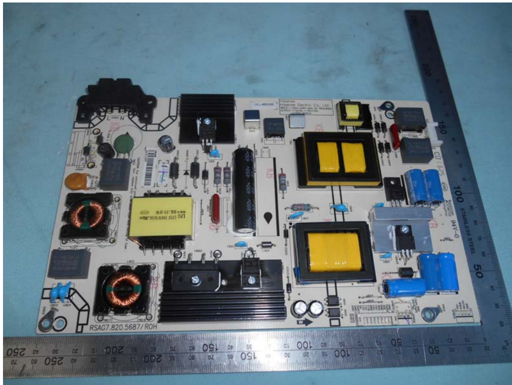
FIGURE 3 LED LCD TV (M/N: 43H7C) POWER BOARD (COMPONENT SIDE)
