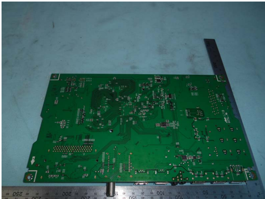
FIGURE 6 LED LCD TV (M/N: 43H7C) MAIN BOARD (SOLDERED SIDE)
