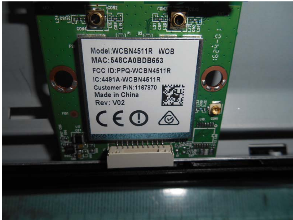
FIGURE 21 LED LCD TV (M/N: 43H7C) RF BOARD LABEL
