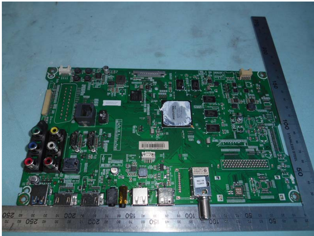
FIGURE 5 LED LCD TV (M/N: 43H7C) MAIN BOARD (COMPONENT SIDE)
