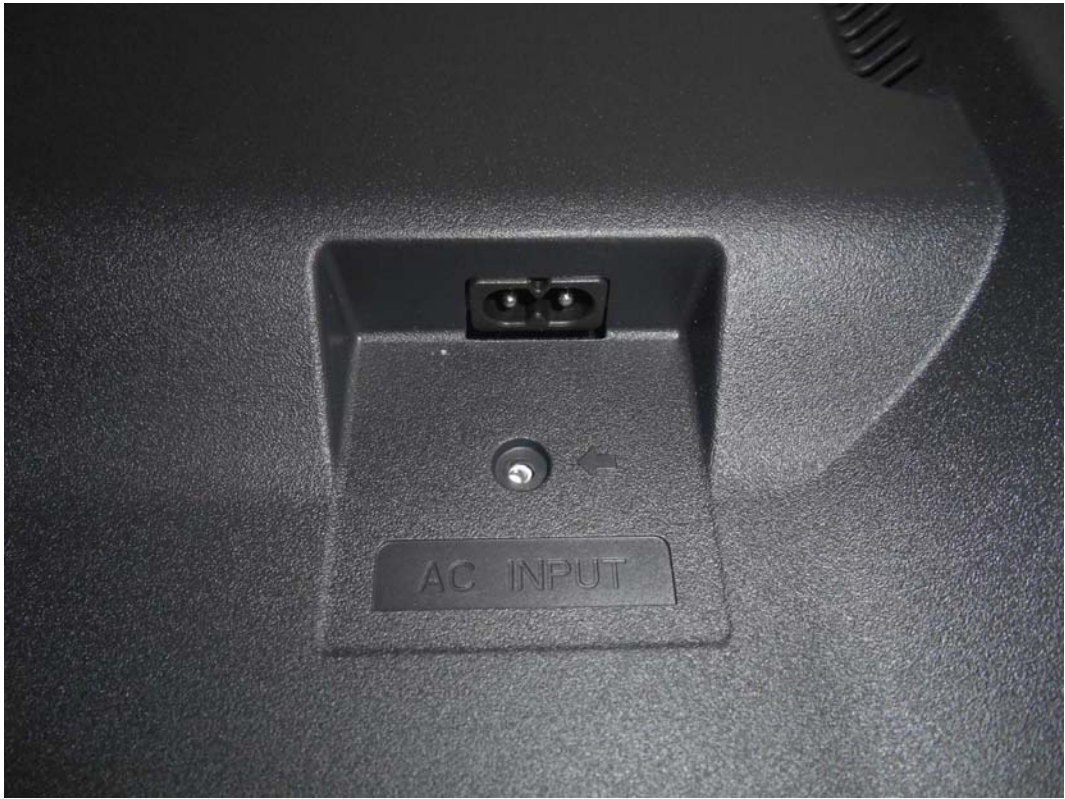
FIGURE 3 LED LCD TV (M/N: 43CU6100) AC PORT
