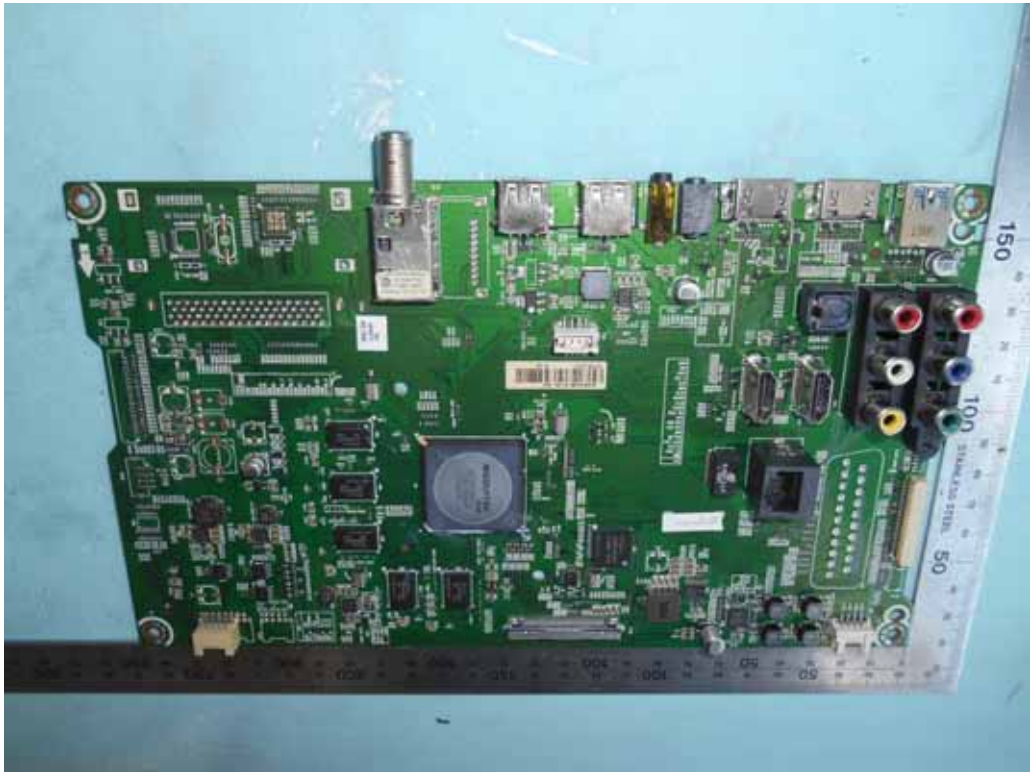
FIGURE 5 LED LCD TV (M/N: RLED4350-UHD-B-SM) MAIN BOARD (COMPONENT SIDE)
