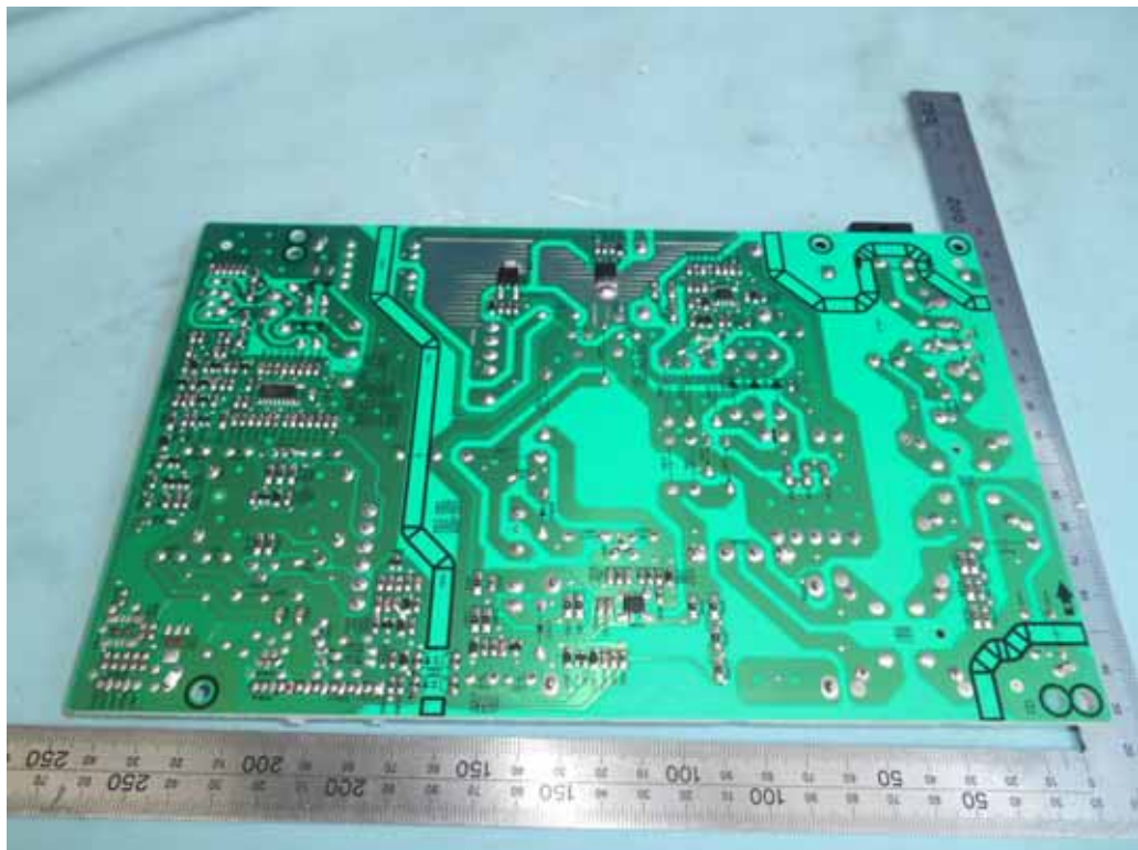
FIGURE 4 LED LCD TV (M/N: RLED4350-UHD-B-SM) POWER BOARD (SOLDERED SIDE)
