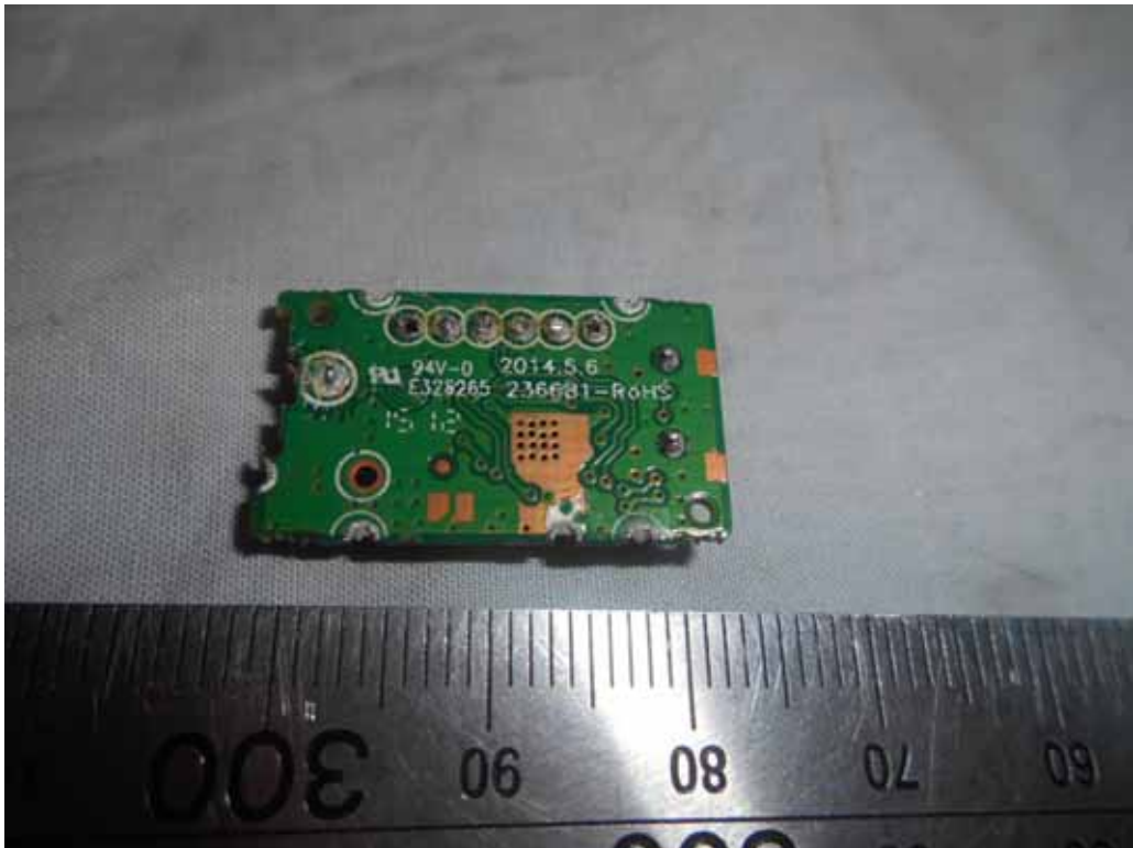
FIGURE 10 LED LCD TV (M/N: RLED4350-UHD-B-SM) TUNER BOARD (SOLDERED SIDE)
