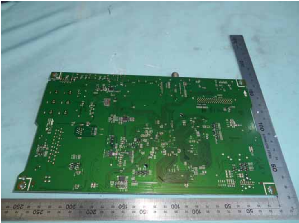
FIGURE 6 LED LCD TV (M/N: RLED4350-UHD-B-SM) MAIN BOARD (SOLDERED SIDE)
