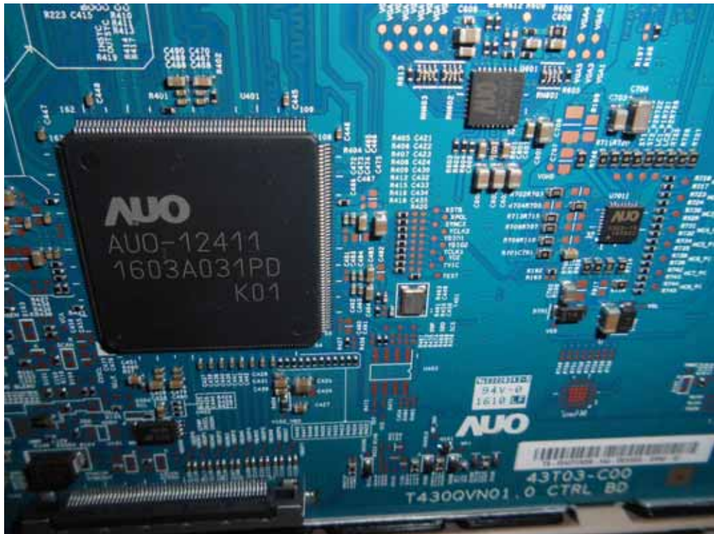
FIGURE 13 LED LCD TV (M/N: RLED4350-UHD-B-SM) CHIP & CRYSTAL ON PANEL BOARD
