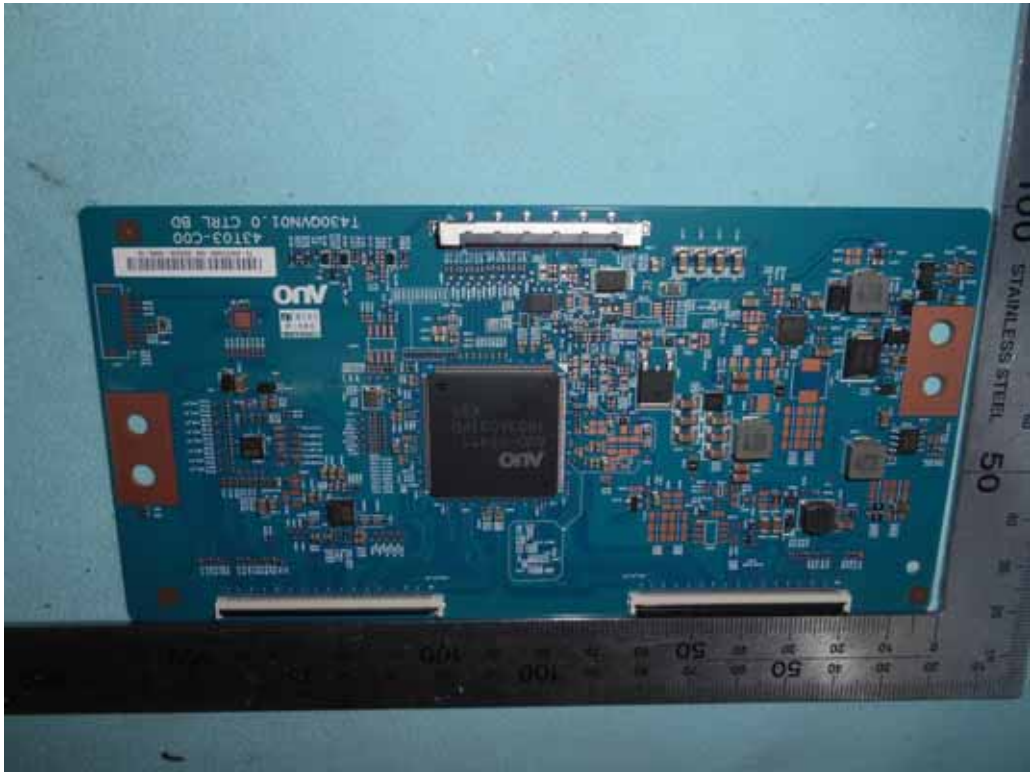
FIGURE 11 LED LCD TV (M/N: RLED4350-UHD-B-SM) PANEL BOARD (COMPONENT SIDE)
