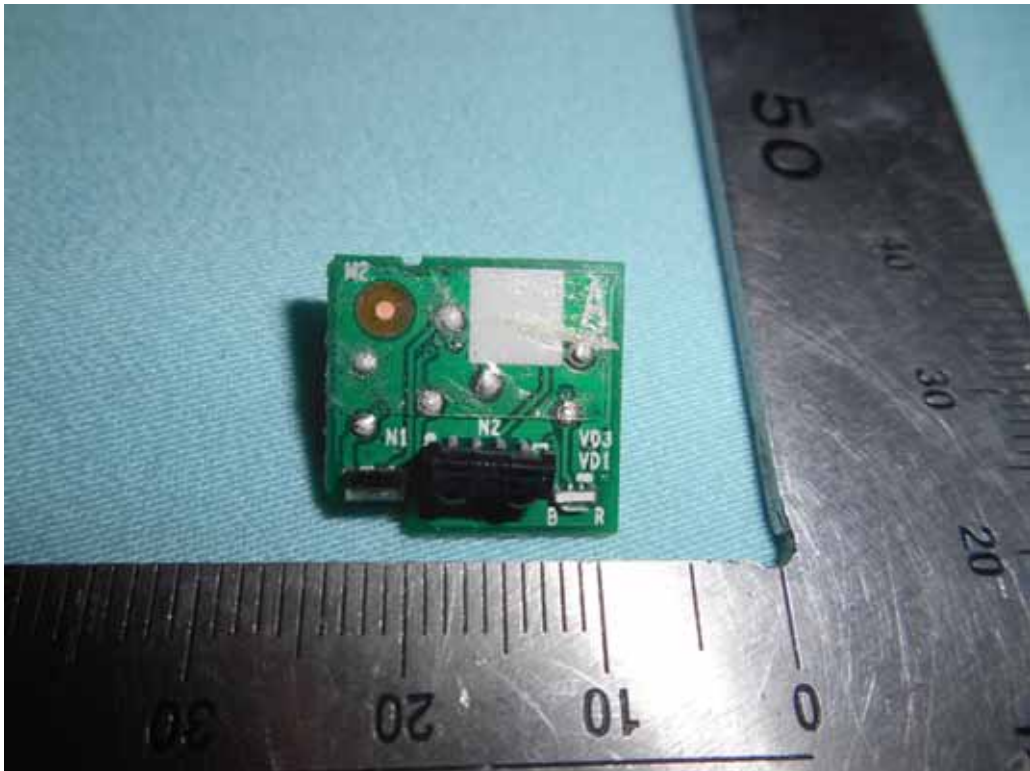
FIGURE 20 LED LCD TV (M/N: RLED4350-UHD-B-SM) IR BOARD (COMPONENT SIDE)
