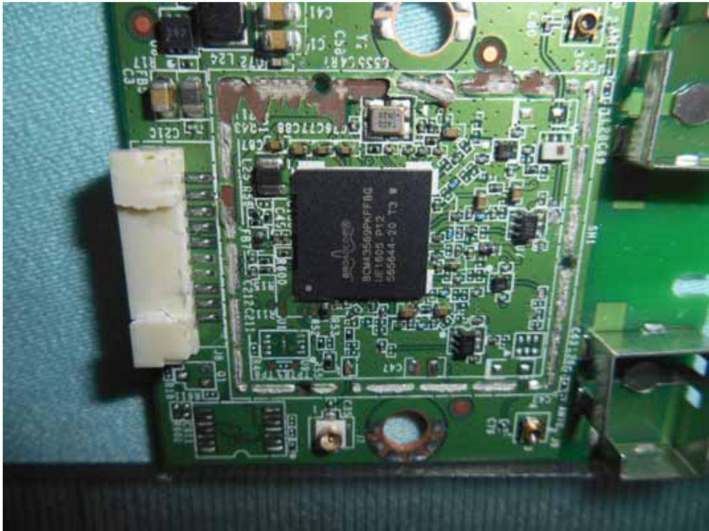
FIGURE 17 LED LCD TV (M/N: RLED4350-UHD-B-SM) RF BOARD COVER REMOVED
