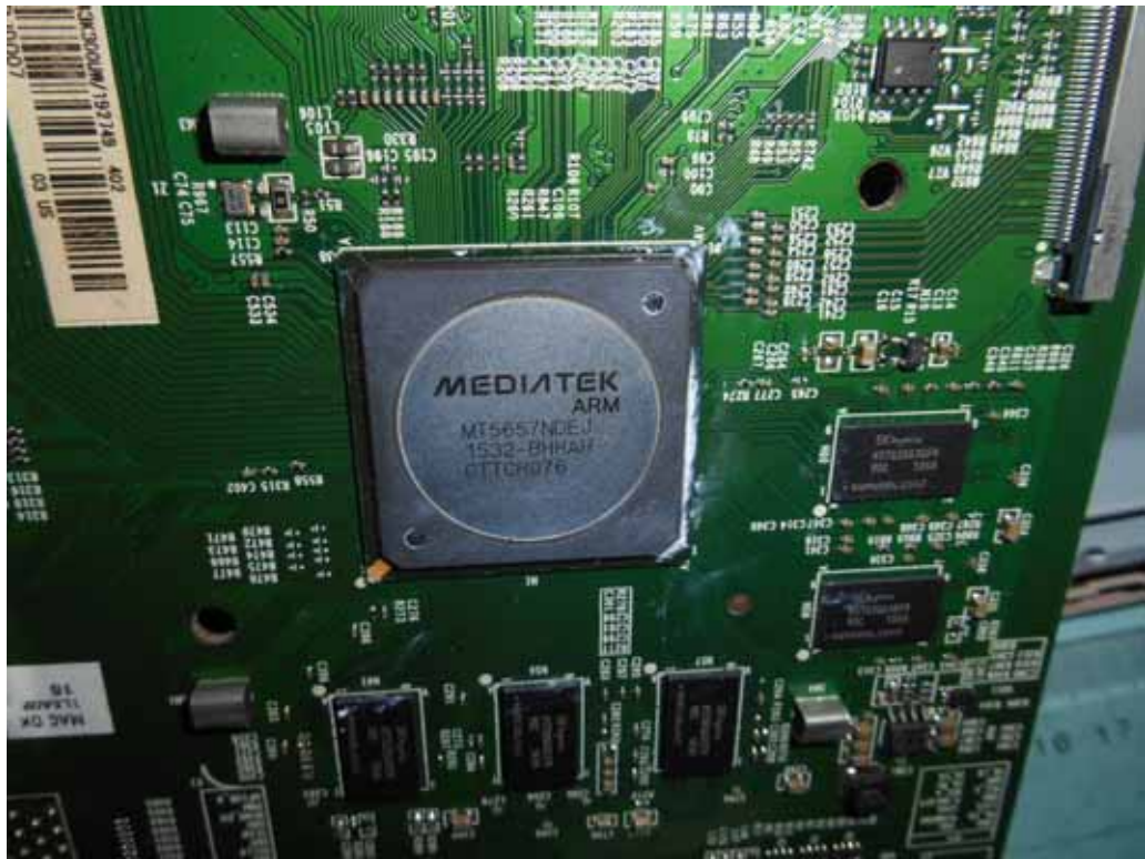
FIGURE 7 LED LCD TV (M/N: RLED4350-UHD-B-SM) CHIP & CRYSTAL ON MAIN BOARD
