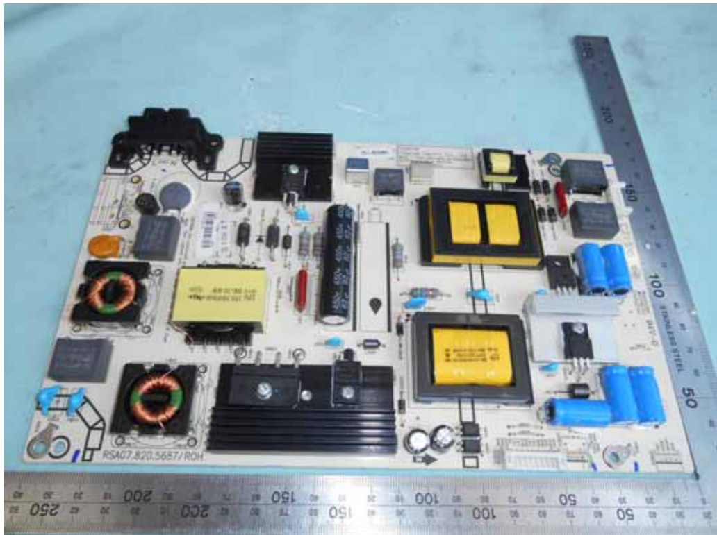
FIGURE 3 LED LCD TV (M/N: RLED4350-UHD-B-SM) POWER BOARD (COMPONENT SIDE)
