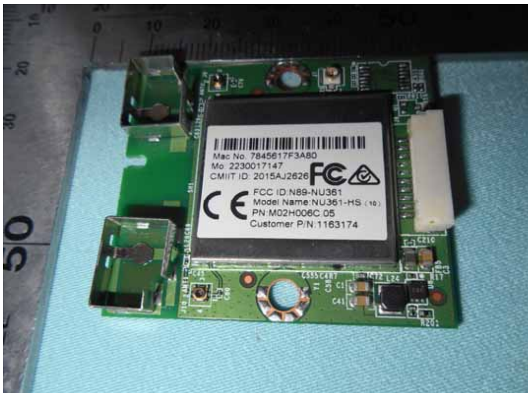
FIGURE 14 LED LCD TV (M/N: RLED4350-UHD-B-SM) RF BOARD (COMPONENT SIDE)
