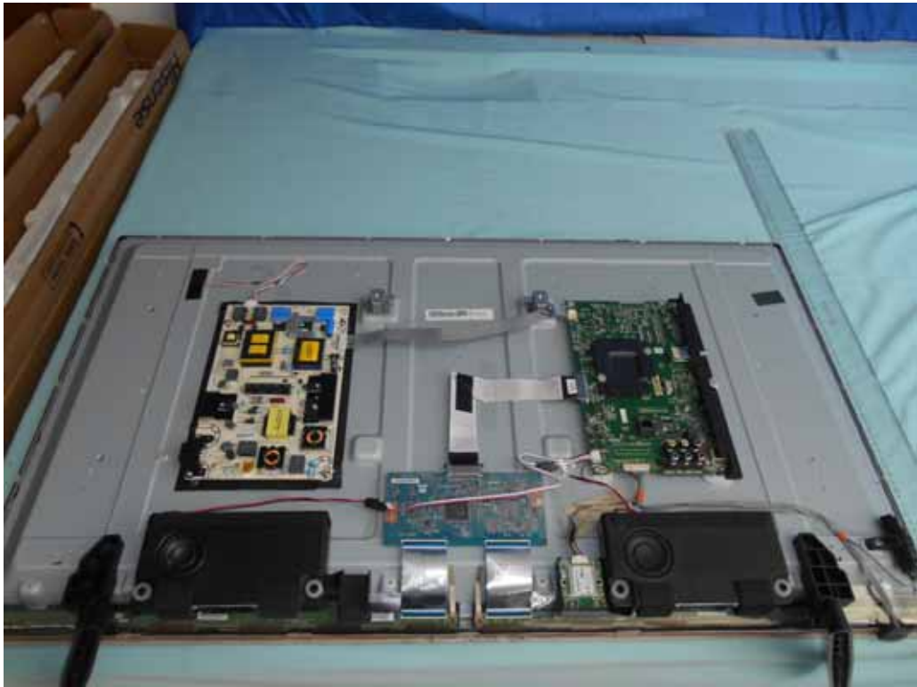
FIGURE 1 LED LCD TV (M/N: RLED4350-UHD-B-SM) COVER REMOVED
