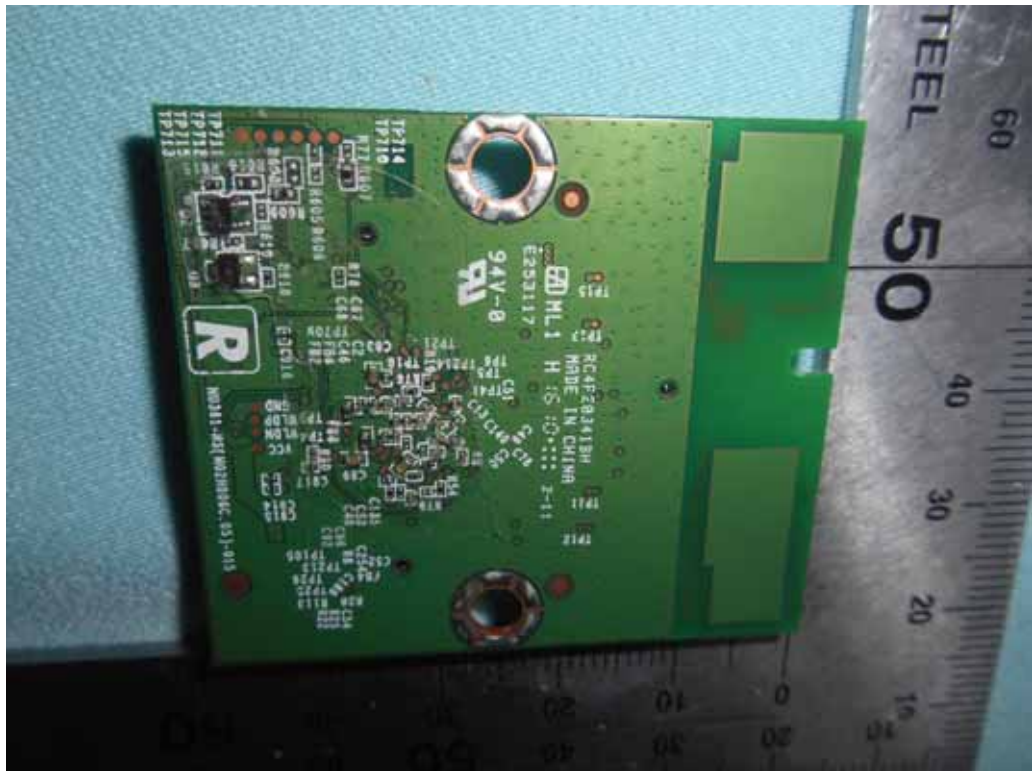
FIGURE 15 LED LCD TV (M/N: RLED4350-UHD-B-SM) RF BOARD (SOLDERED SIDE)
