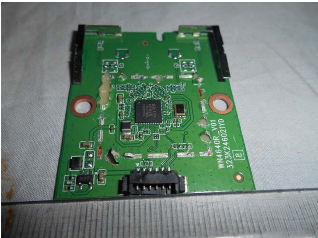
FIGURE 13 LED LCD TV (M/N: LC-40N5000U) RF BOARD COVER REMOVED
