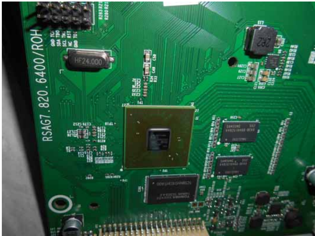
FIGURE 7 LED LCD TV (M/N: LC-43N4000U) CHIP & CRYSTAL ON MAIN BOARD
