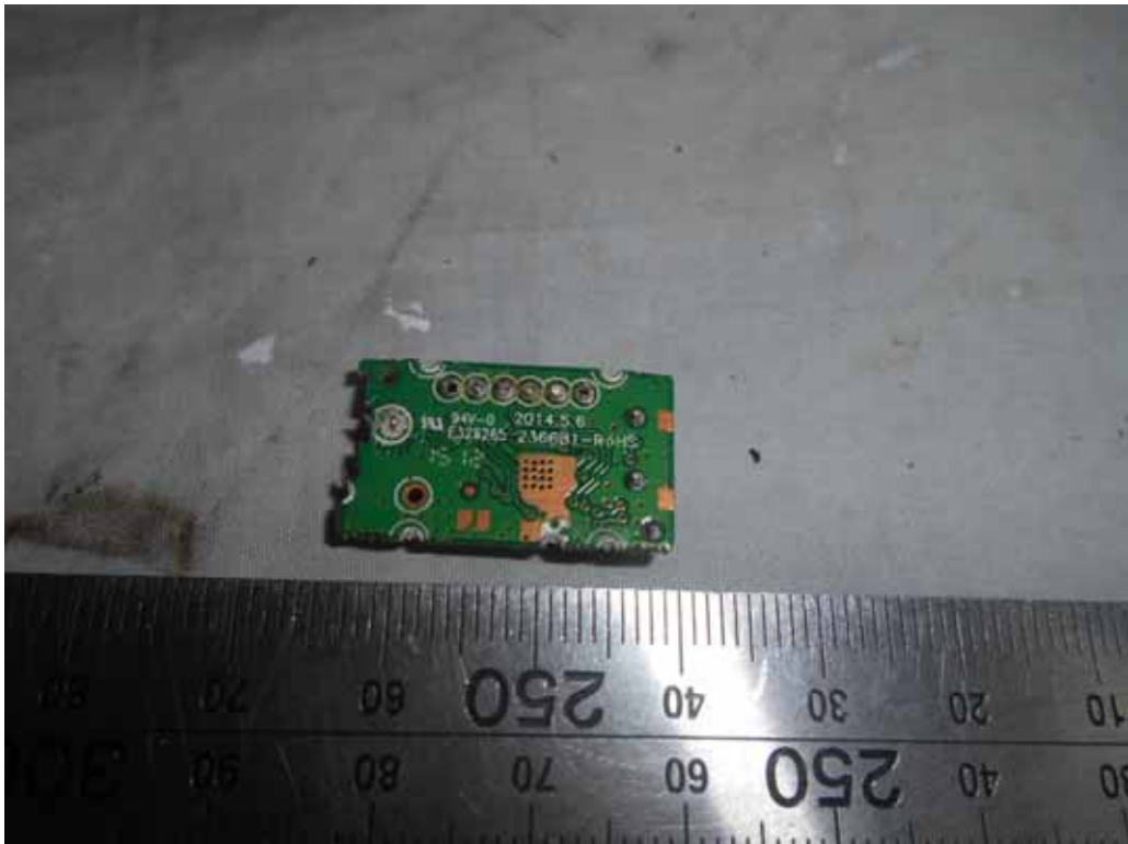
FIGURE 10 LED LCD TV (M/N: LC-43N4000U) TUNER BOARD (SOLDERED SIDE)
