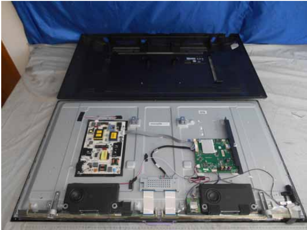
FIGURE 1 LED LCD TV (M/N: LC-43N4000U) COVER REMOVED
