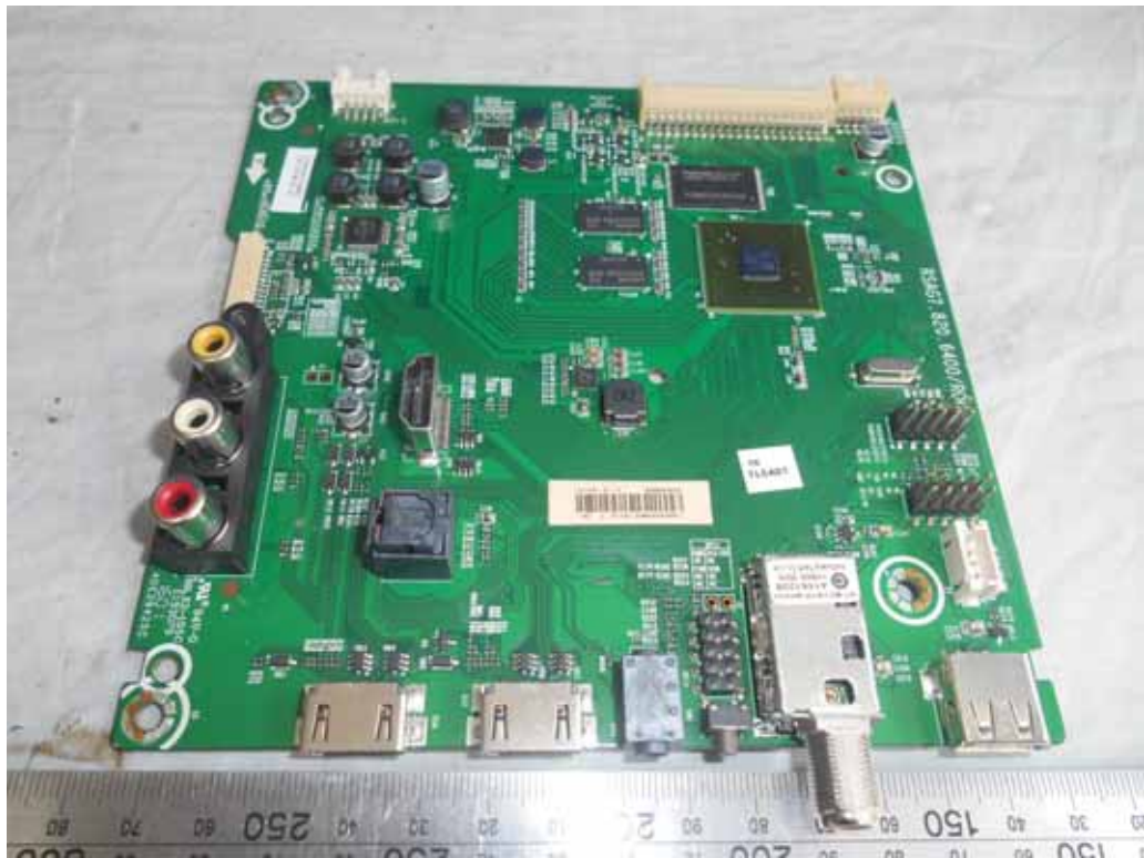
FIGURE 5 LED LCD TV (M/N: LC-43N4000U) MAIN BOARD (COMPONENT SIDE)
