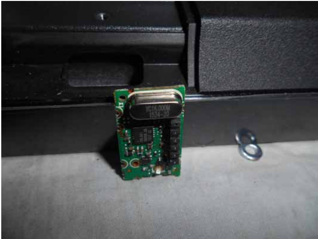
FIGURE 11 LED LCD TV (M/N: LC-43N4000U) TUNER & CRYSTAL ON MAIN BOARD
