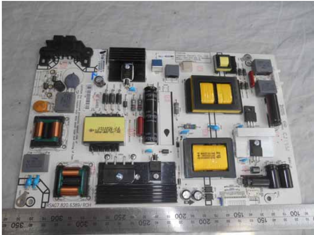
FIGURE 3 LED LCD TV (M/N: LC-43N4000U) POWER BOARD (COMPONENT SIDE)
