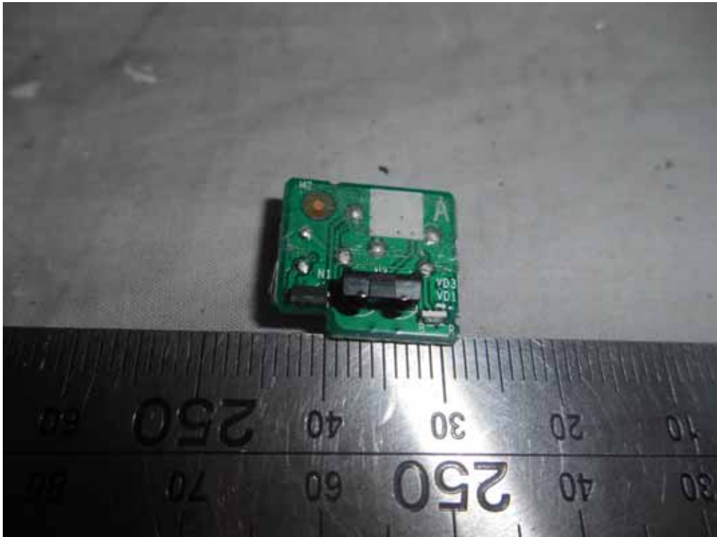
FIGURE 21 LED LCD TV (M/N: LC-43N4000U) IR BOARD (COMPONENT SIDE)
