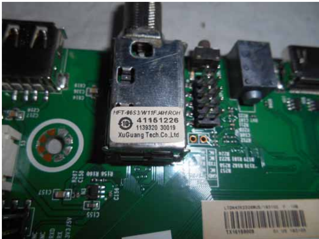
FIGURE 8 LED LCD TV (M/N: LC-43N4000U) TUNER
