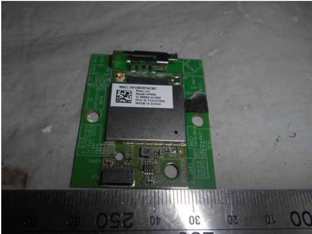
FIGURE 15 LED LCD TV (M/N: LC-43N4000U) RF BOARD (COMPONENT SIDE)
