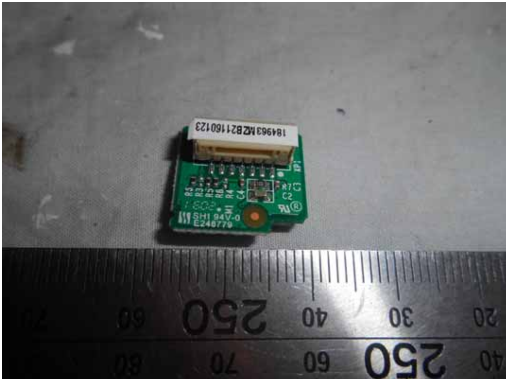
FIGURE 22 LED LCD TV (M/N: LC-43N4000U) IR BOARD (SOLDERED SIDE)
