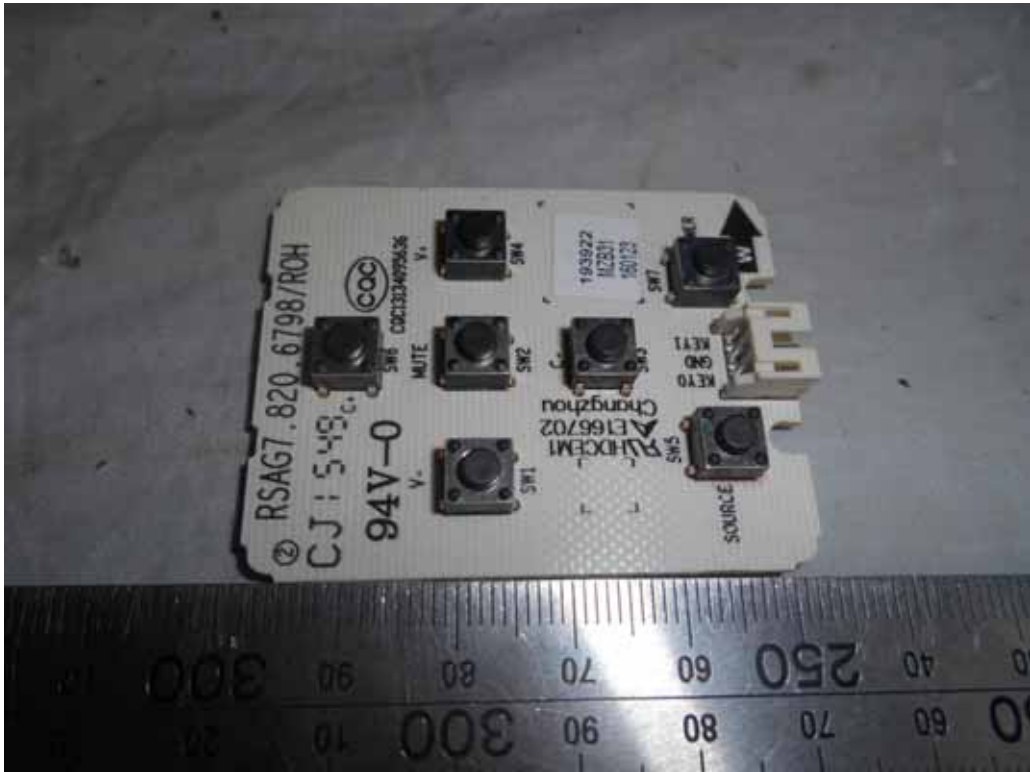
FIGURE 19 LED LCD TV (M/N: LC-43N4000U) KEY BOARD (COMPONENT SIDE)
