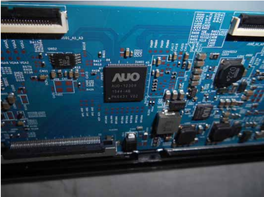
FIGURE 14 LED LCD TV (M/N: LC-43N4000U) CHIP ON PANEL BOARD
