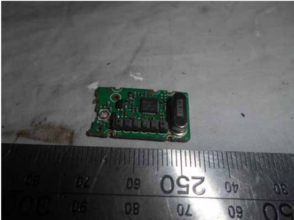
FIGURE 9 LED LCD TV (M/N: LC-43N4000U) TUNER BOARD (COMPONENT SIDE)
