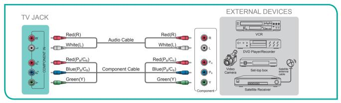
Figure 3. AV device with a component video cable
