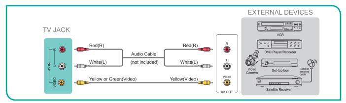
Figure 2. AV device with a composite video cable
