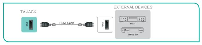
Figure 4. AV device with an HDMI cable
