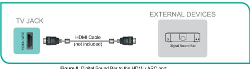
Figure 8. Digital Sound Bar to the HDMI / ARC port
