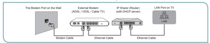
Figure 11. Connect a LAN port on the TV to an IP sharer
