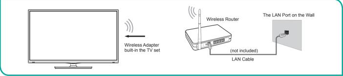
Figure 9. Connect the TV to a wireless network
