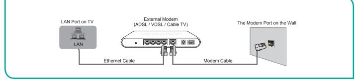
Figure 10. Connect a LAN port on the TV to an external modem
