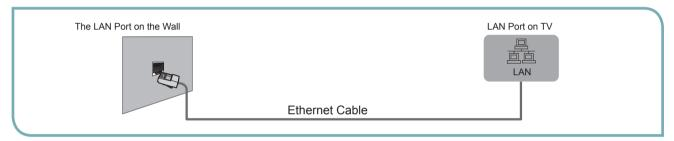
Figure 12. Connect a LAN port on the TV to a network wall outlet
