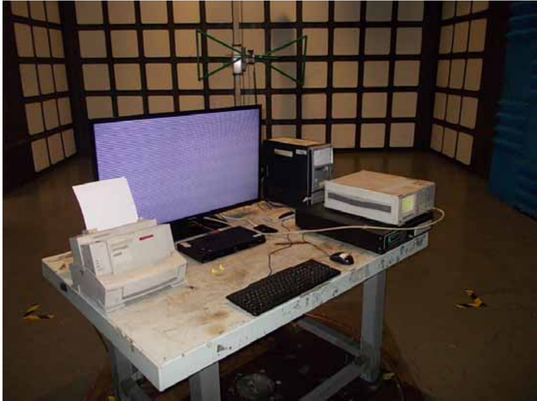
SETUP WITH MAXIMUM DETECTED EMISSION AT HORIZONTAL POLARIZATION (TEST MODE: HDMI 1920*1080@60Hz)
