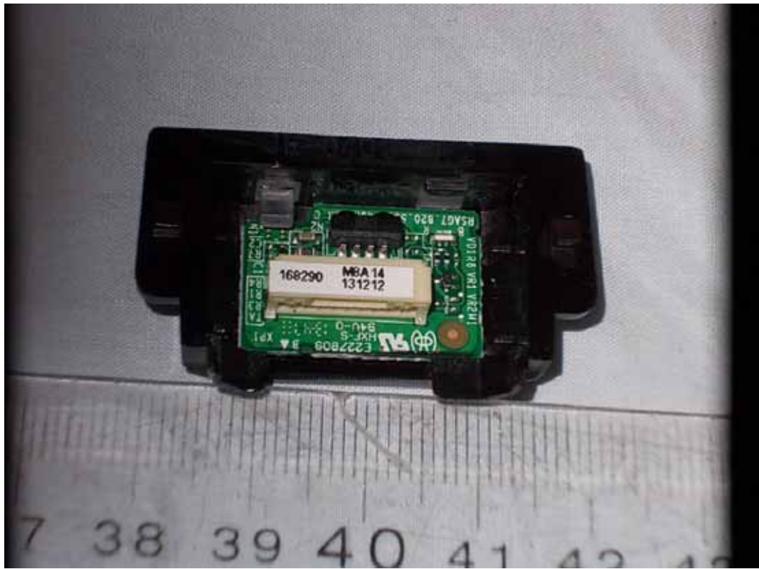
FIGURE 11 LED LCD TV (M/N: 40K20D) IR BOARD
