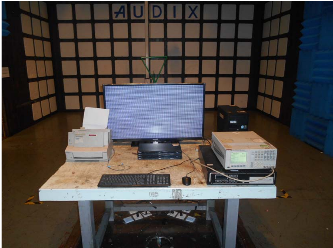
FRONT VIEW OF RADIATED EMISSION TEST
