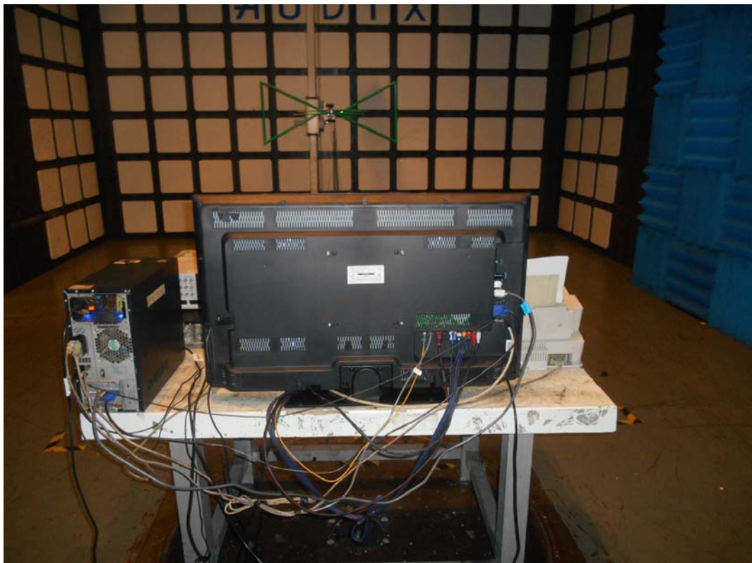
BACK VIEW OF RADIATED EMISSION TEST
