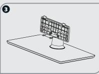
Secure the stand cover to the stand column horizontally with the 2 screws (ST4×14) provided.
