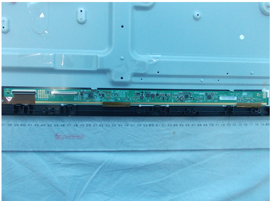
FIGURE 15 LED LCD TV (M/N: 39A300MH) LCD PANEL CONTROL BOARD (BACK SIDE)
