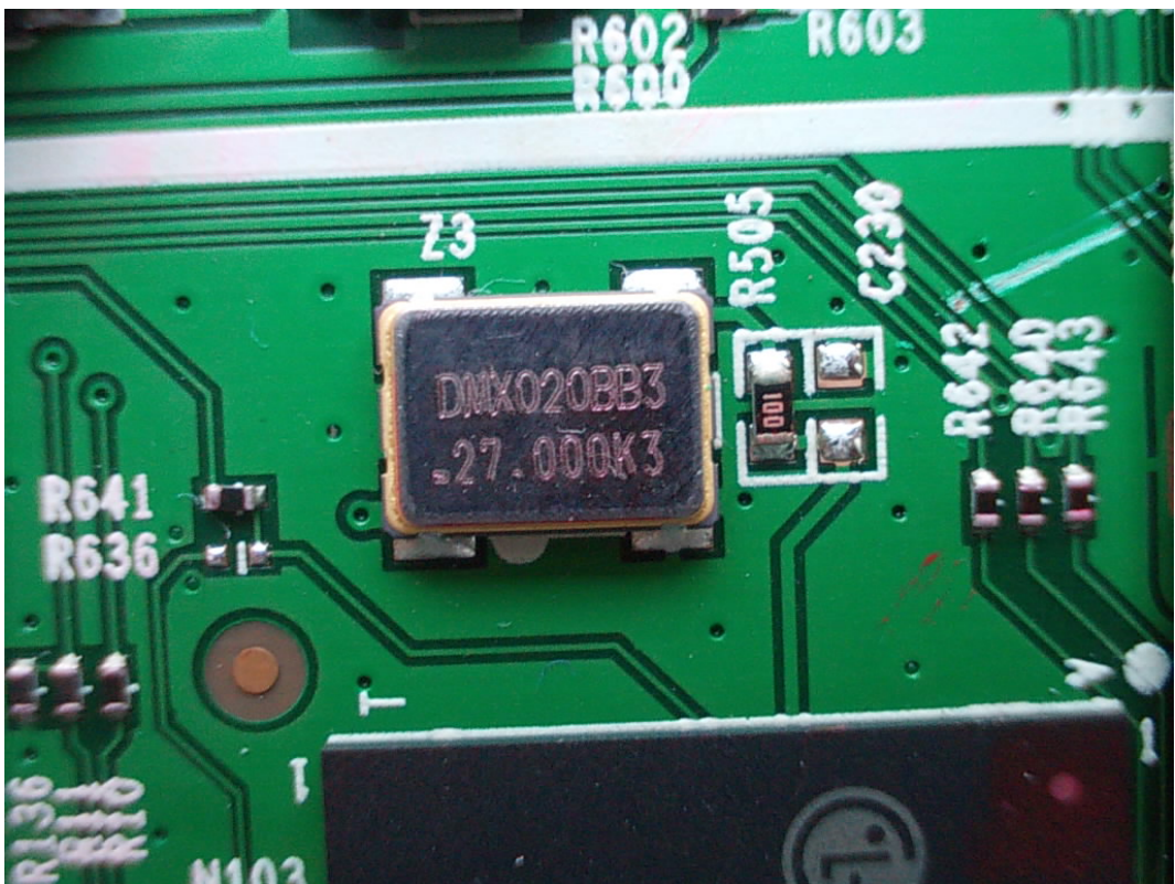
FIGURE 9 LED LCD TV (M/N: 39A300MH) CRYSTAL #3 ON MAIN BOARD
