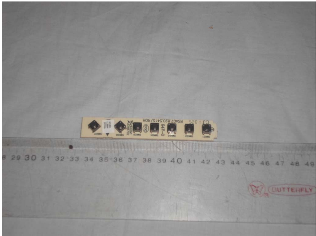
FIGURE 11 LED LCD TV (M/N: LTDN40K20DUS) KEY BOARD (COMPONENT SIDE)
