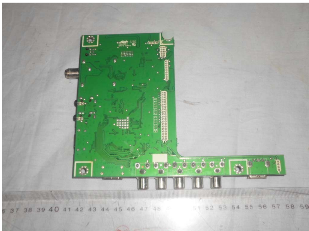
FIGURE 6 LED LCD TV (M/N: LTDN40K20DUS) MAIN BOARD (SOLDERED SIDE)
