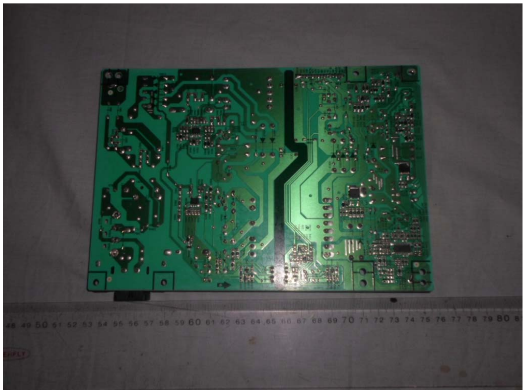
FIGURE 4 LED LCD TV (M/N: LTDN40K20DUS) POWER BOARD (SOLDERED SIDE)
