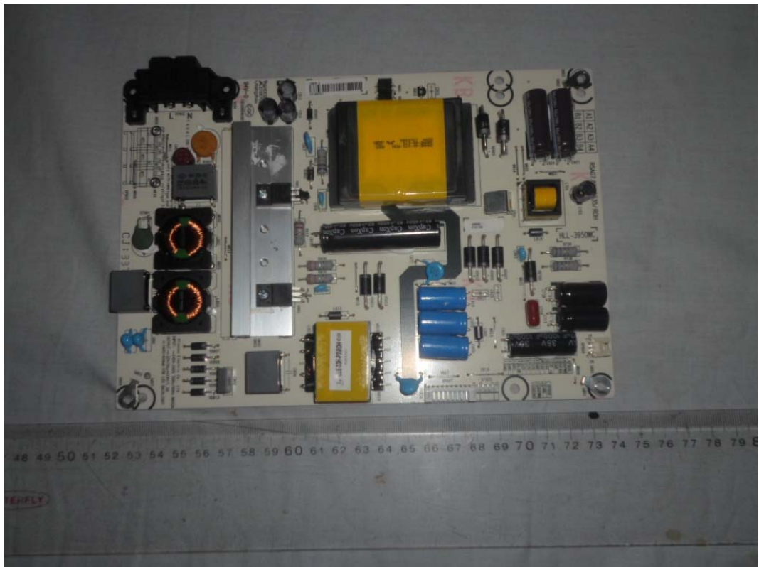
FIGURE 3 LED LCD TV (M/N: LTDN40K20DUS) POWER BOARD (COMPONENT SIDE)
