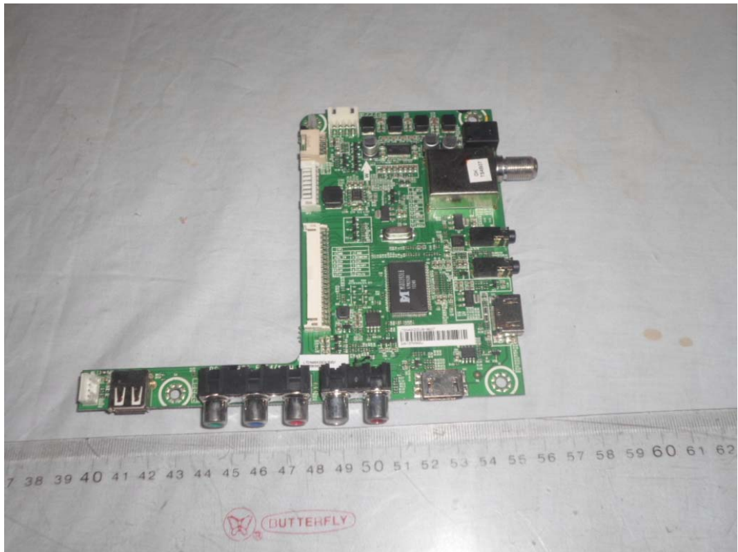
FIGURE 5 LED LCD TV (M/N: LTDN40K20DUS) MAIN BOARD (COMPONENT SIDE)
