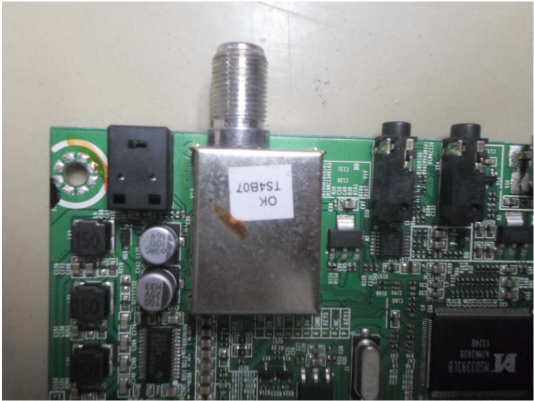
FIGURE 7 LED LCD TV (M/N: LTDN40K20DUS) TUNER ON MAIN BOARD
