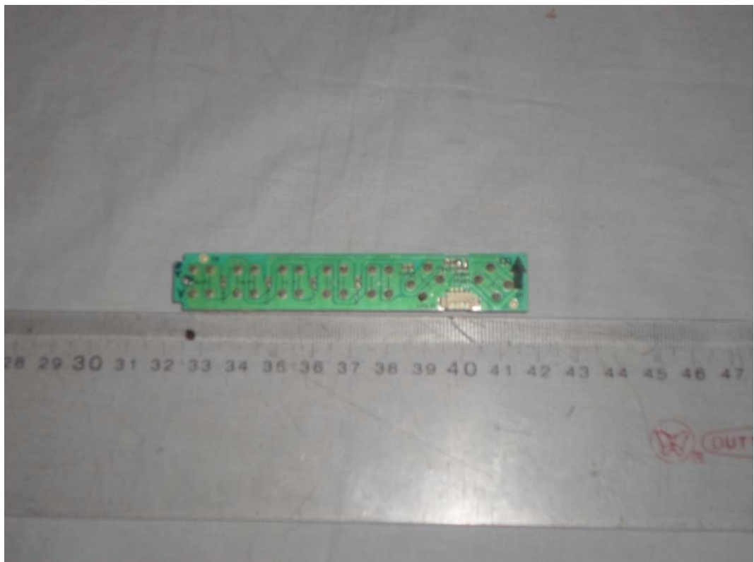
FIGURE 12 LED LCD TV (M/N: LTDN40K20DUS) KEY BOARD (SOLDERED SIDE)
