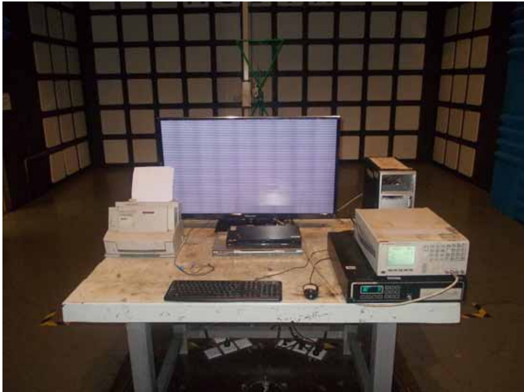
FRONT VIEW OF RADIATED EMISSION TEST
