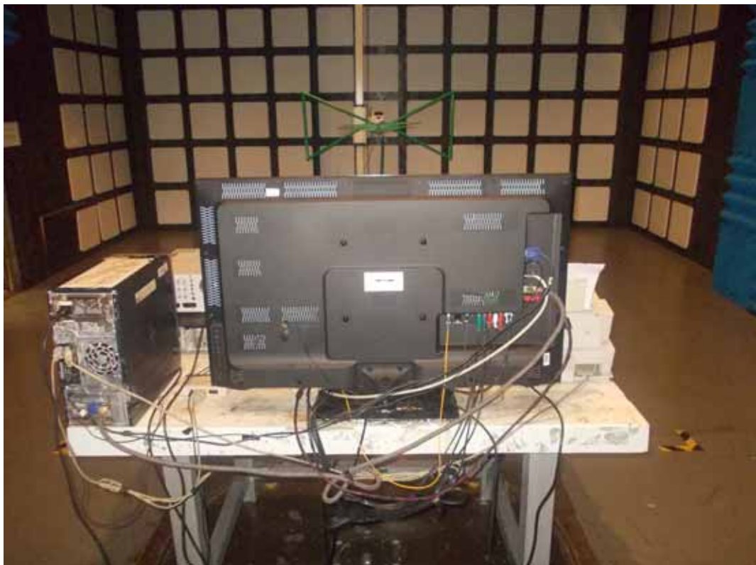
BACK VIEW OF RADIATED EMISSION TEST
