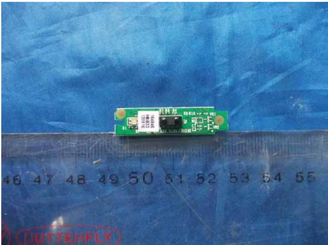
FIGURE 18 LED LCD TV (M/N: 40K368AW) IR BOARD (COMPONENT SIDE)
