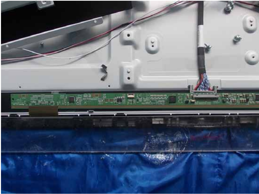
FIGURE 15 LED LCD TV (M/N: 40K368AW) LCD PANEL CONTROL BOARD (COMPONENT SIDE)
