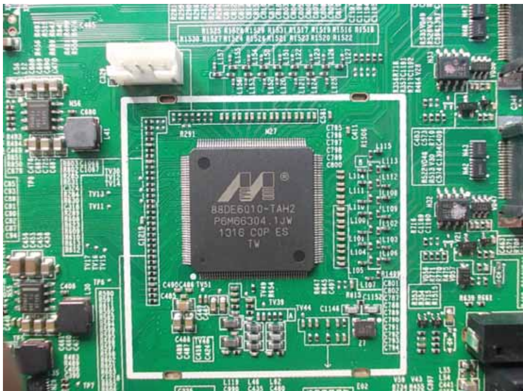
FIGURE 8 LED LCD TV (M/N: 40K368AW) CHIP #1 ON MAIN BOARD
