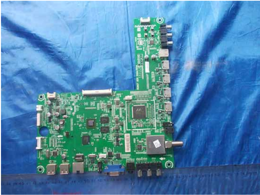
FIGURE 5 LED LCD TV (M/N: 40K368AW) MAIN BOARD (COMPONENT SIDE)
