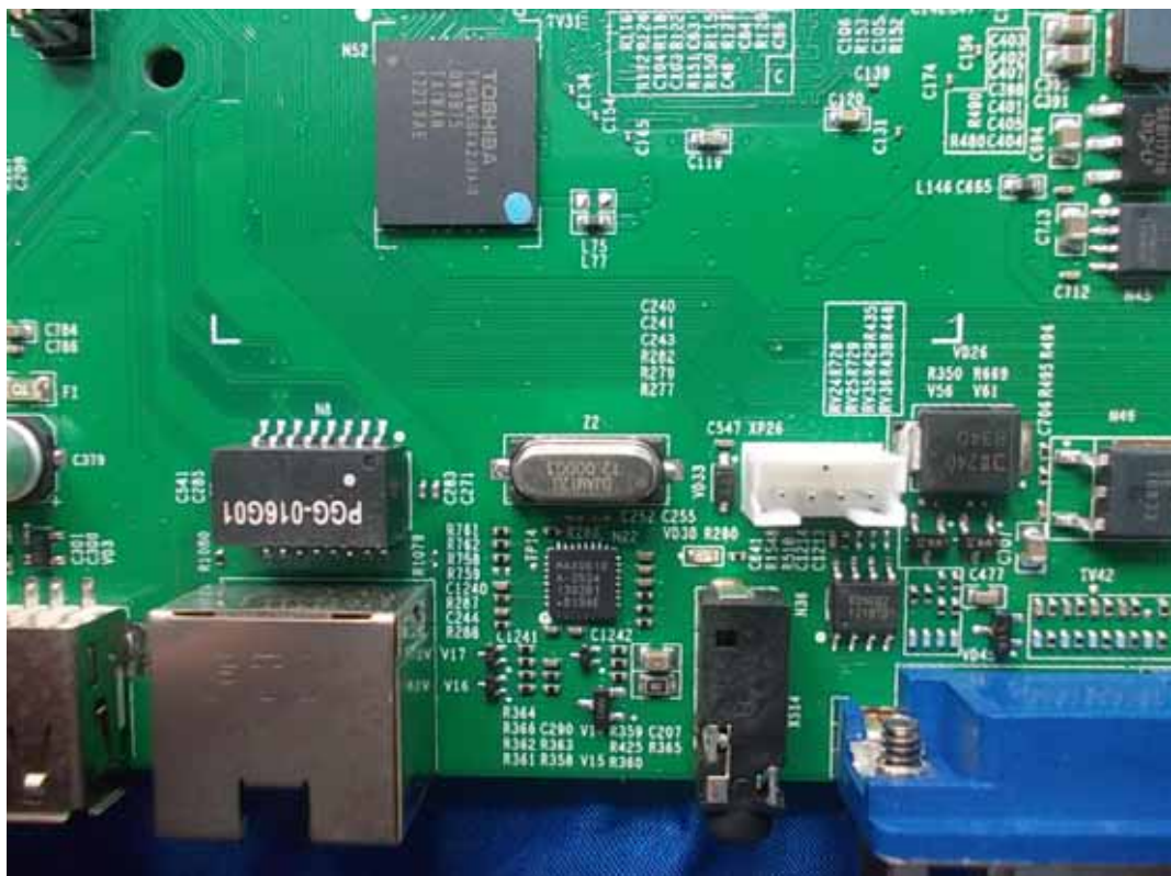
FIGURE 10 LED LCD TV (M/N: 40K368AW) CRYSTAL #1 ON MAIN BOARD
