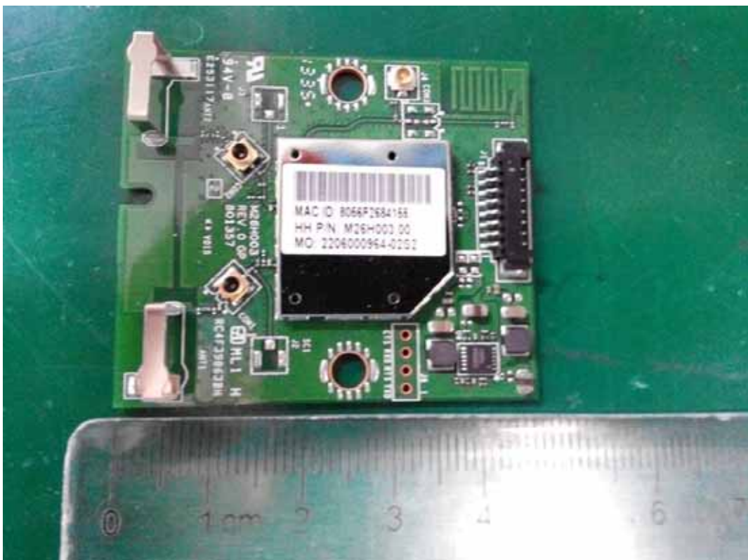
FIGURE 12 LED LCD TV (M/N: 40K368AW) RF BOARD (COMPONENT SIDE)
