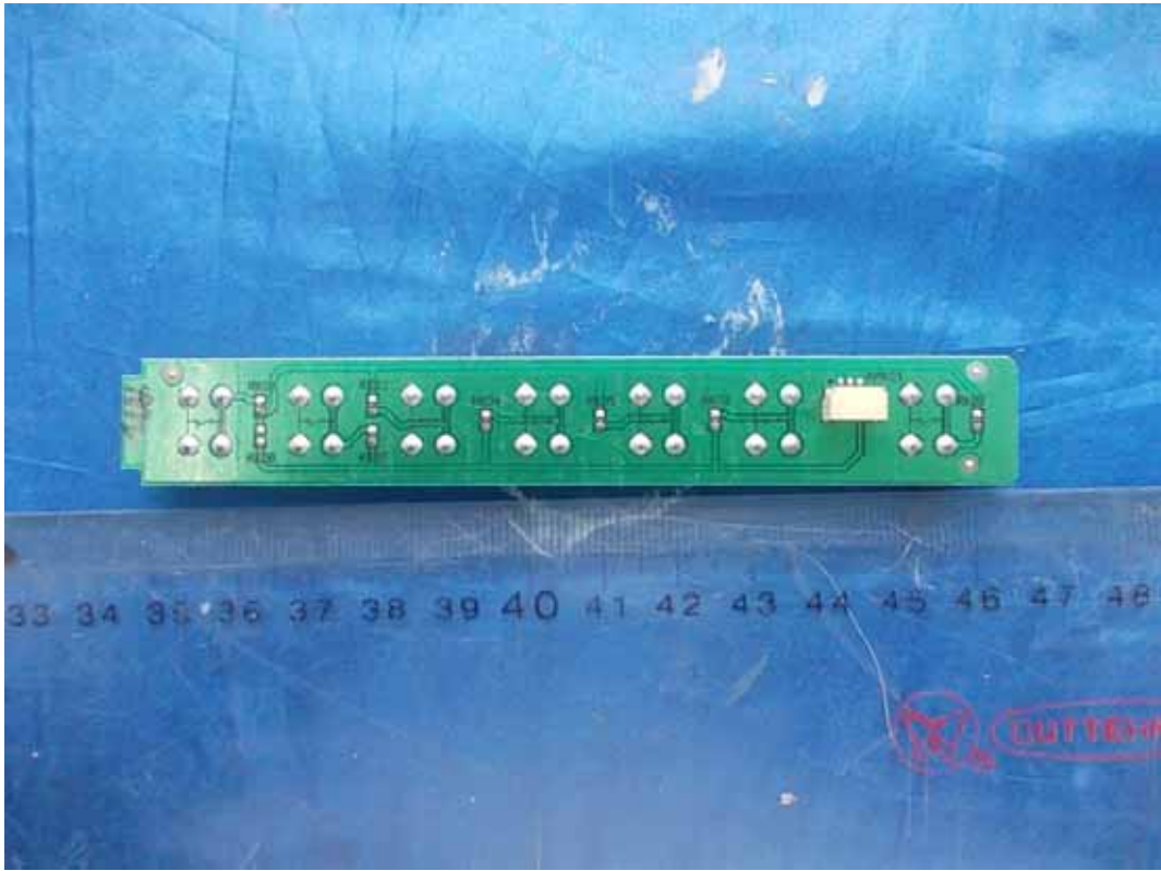
FIGURE 21 LED LCD TV (M/N: 40K368AW) KEY BOARD (SOLDERED SIDE)
