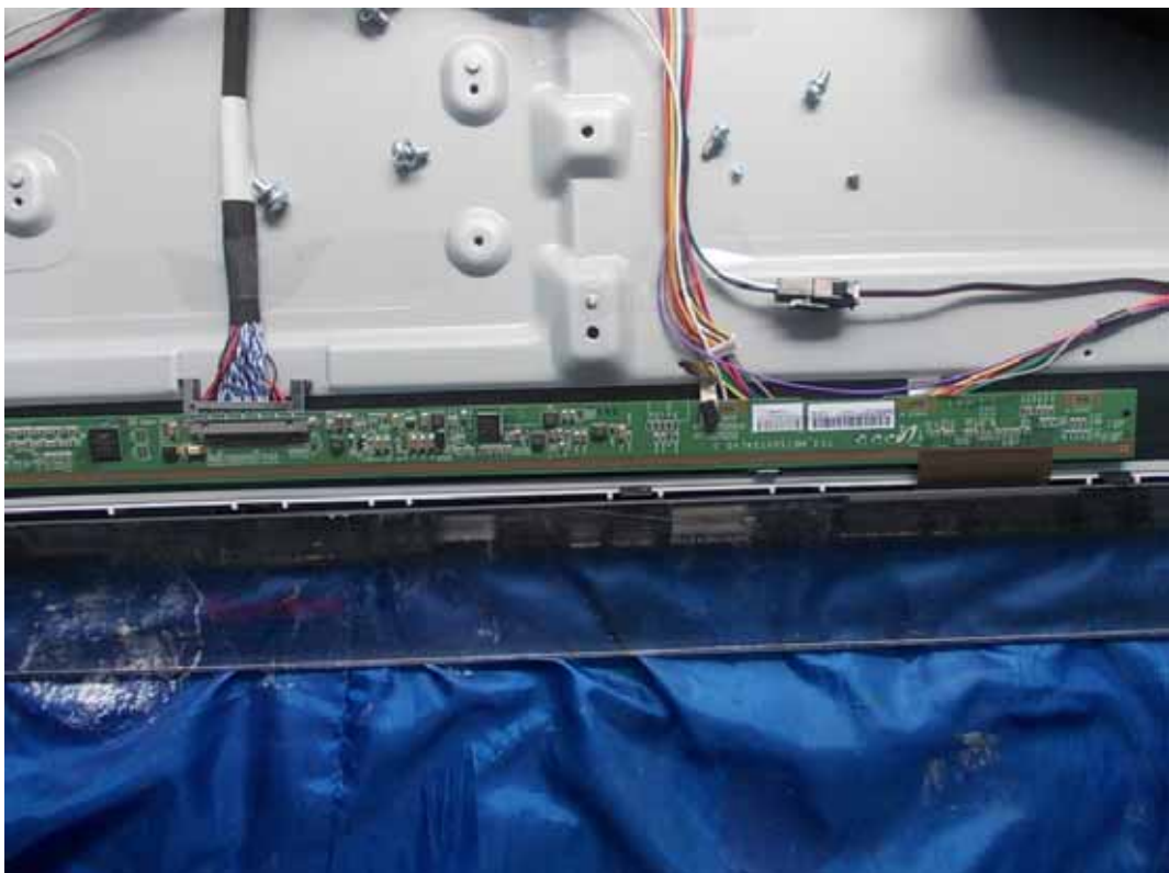
FIGURE 14 LED LCD TV (M/N: 40K368AW) LCD PANEL CONTROL BOARD (COMPONENT SIDE)
