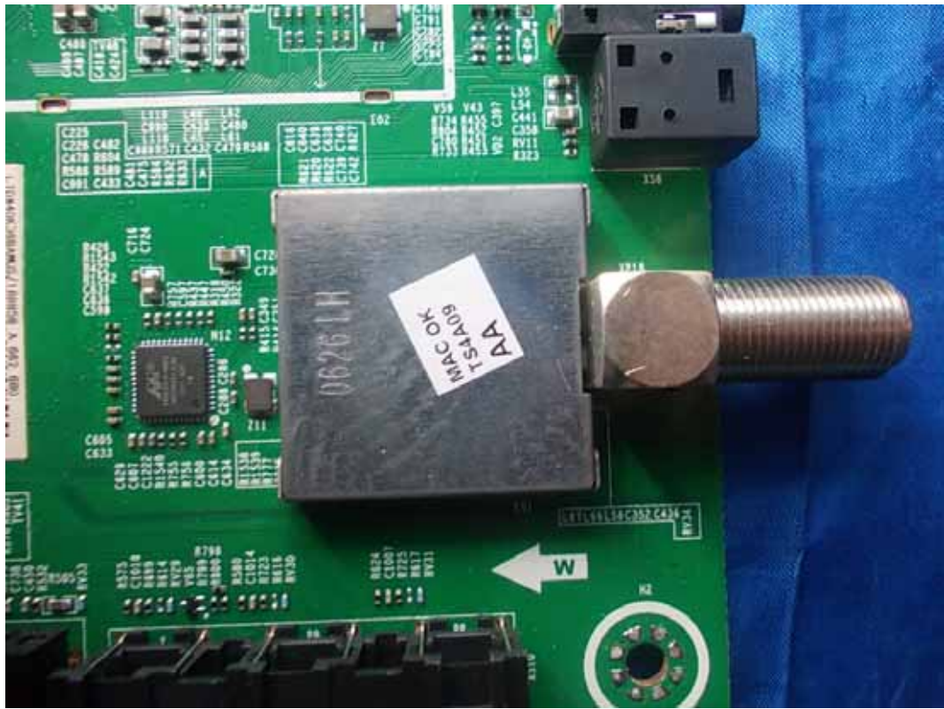
FIGURE 7 LED LCD TV (M/N: 40K368AW) TUNER ON MAIN BOARD
