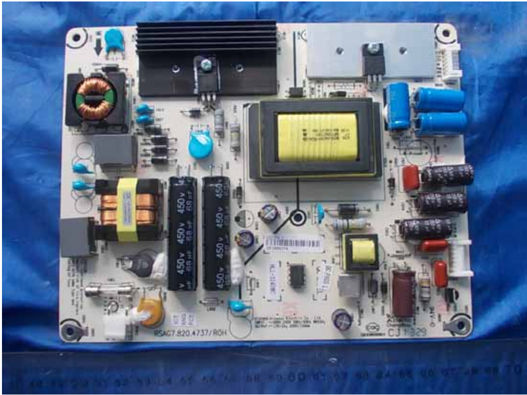
FIGURE 3 LED LCD TV (M/N: 40K368AW) POWER BOARD (COMPONENT SIDE)
