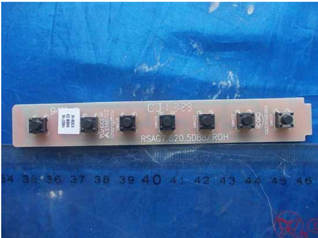
FIGURE 20 LED LCD TV (M/N: 40K368AW) KEY BOARD (COMPONENT SIDE)
