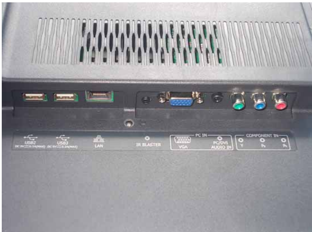
FIGURE 4 LED LCD TV (M/N: 40K368AW) PORTS #2
