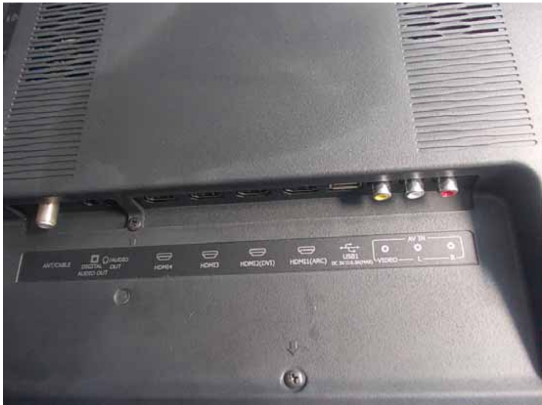
FIGURE 3 LED LCD TV (M/N: 40K368AW) PORTS #1
