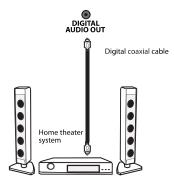
3 Connect the other end of the audio cable to the digital coaxial input jack on the home theater system.
