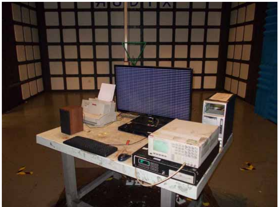
SETUP WITH MAXIMUM DETECTED EMISSION AT VERTICAL POLARIZATION (TEST MODE: D-SUB 640*480@60Hz)
