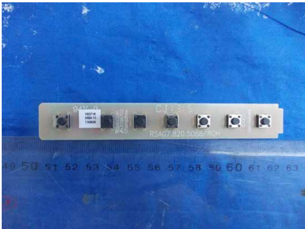
FIGURE 10 LED LCD TV (M/N: LTDN39K366MH) KEY BOARD (COMPONENT SIDE)
