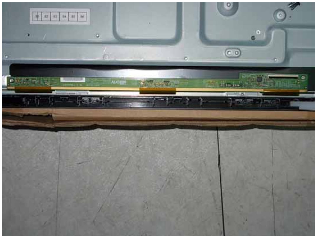
FIGURE 14 LED LCD TV (M/N: LTDN39K366MH) LCD PANEL CONTROL BOARD
