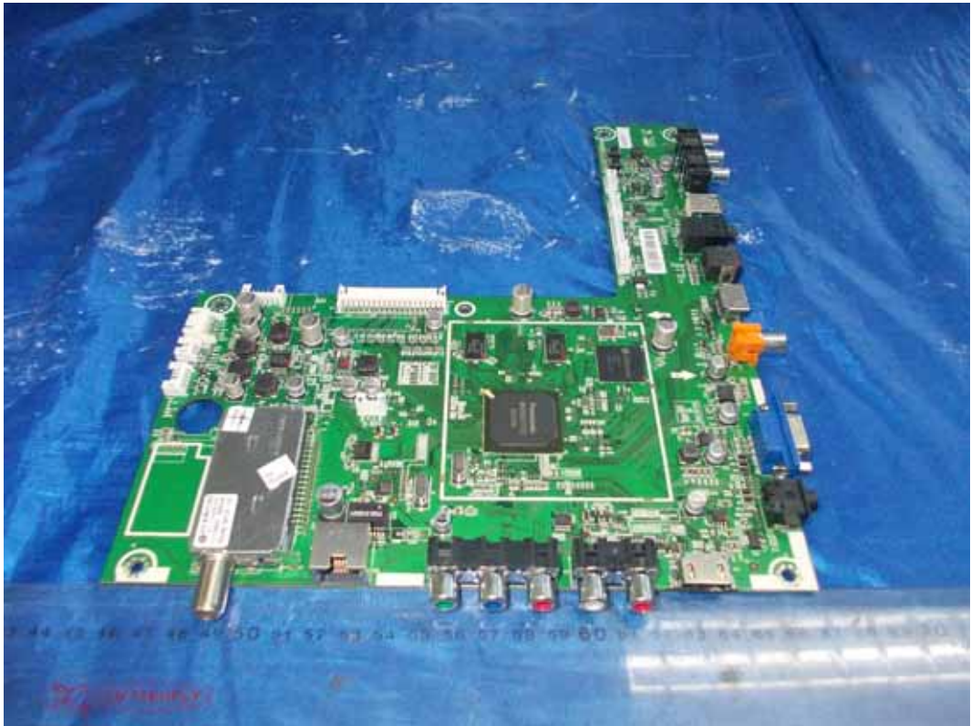
FIGURE 5 LED LCD TV (M/N: LTDN39K366MH) MAIN BOARD (COMPONENT SIDE)
