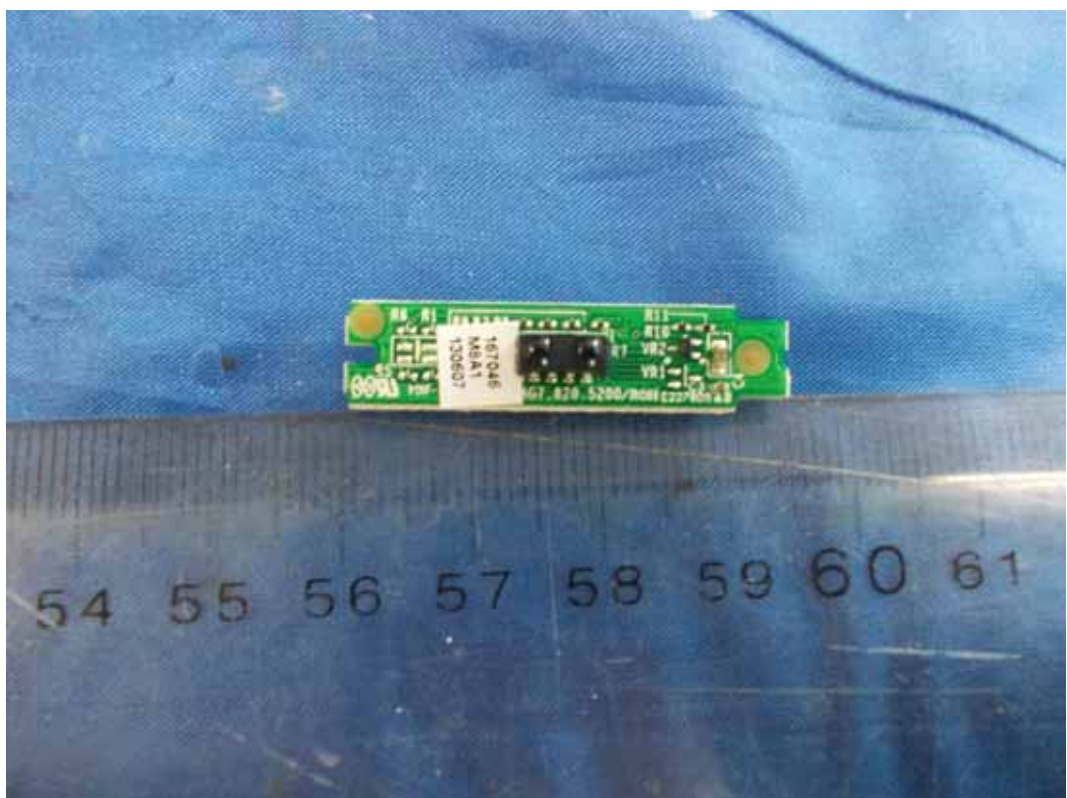
FIGURE 12 LED LCD TV (M/N: LTDN39K366MH) IR BOARD (COMPONENT SIDE)
