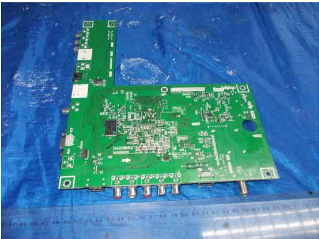
FIGURE 6 LED LCD TV (M/N: LTDN39K366MH) MAIN BOARD (SOLDERED SIDE)
