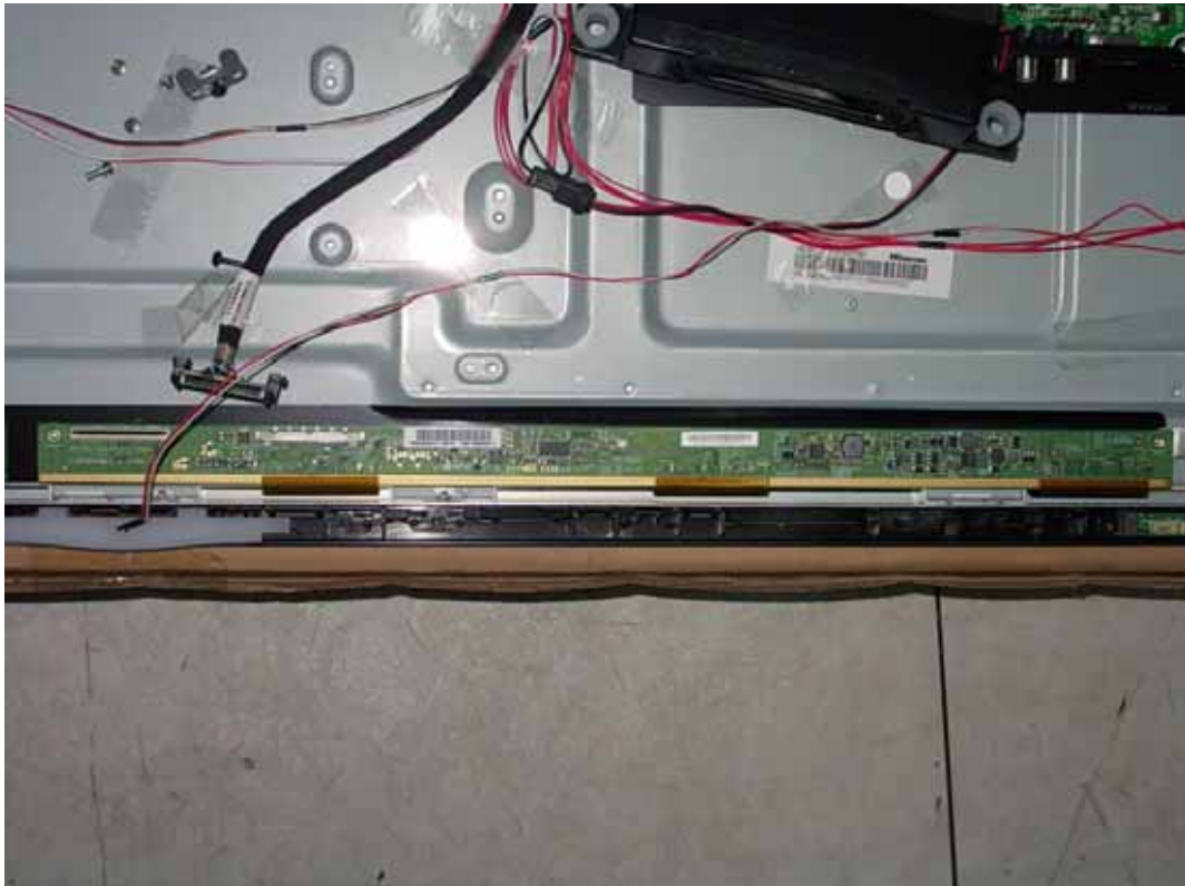
FIGURE 15 LED LCD TV (M/N: LTDN39K366MH) LCD PANEL CONTROL BOARD
