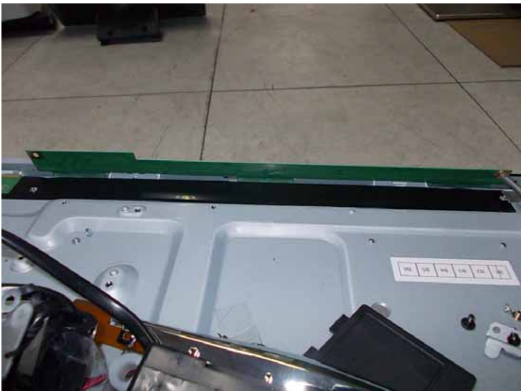
FIGURE 16 LED LCD TV (M/N: LTDN39K366MH) LCD PANEL CONTROL BOARD
