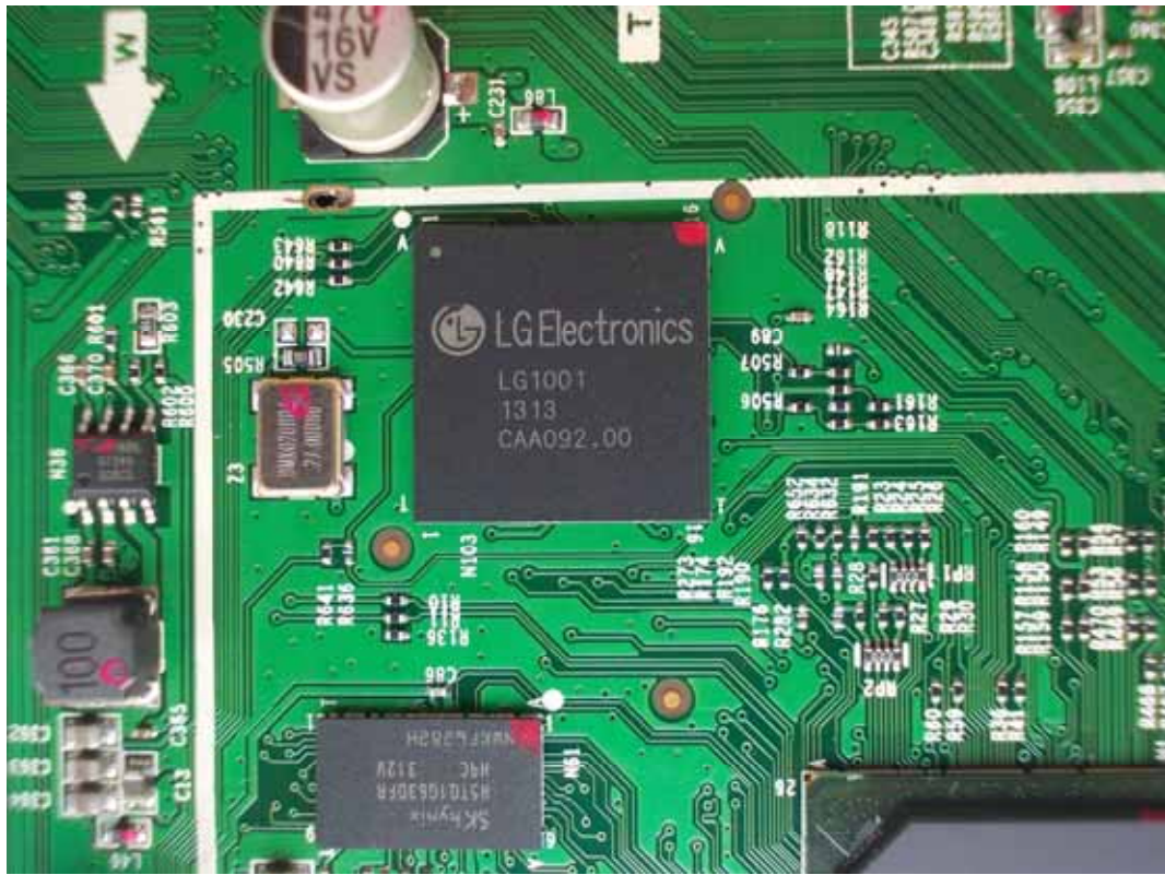
FIGURE 9 LED LCD TV (M/N: LTDN39K366MH) CHIP & CRYSTAL ON MAIN BOARD
