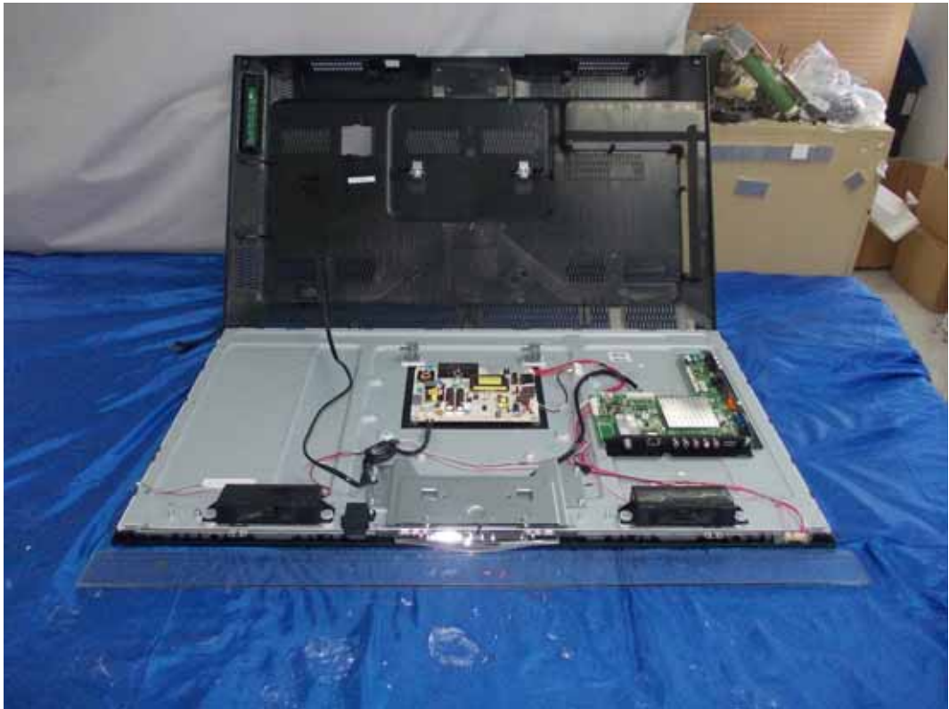
FIGURE 1 LED LCD TV (M/N: LTDN39K366MH) COVER REMOVED
