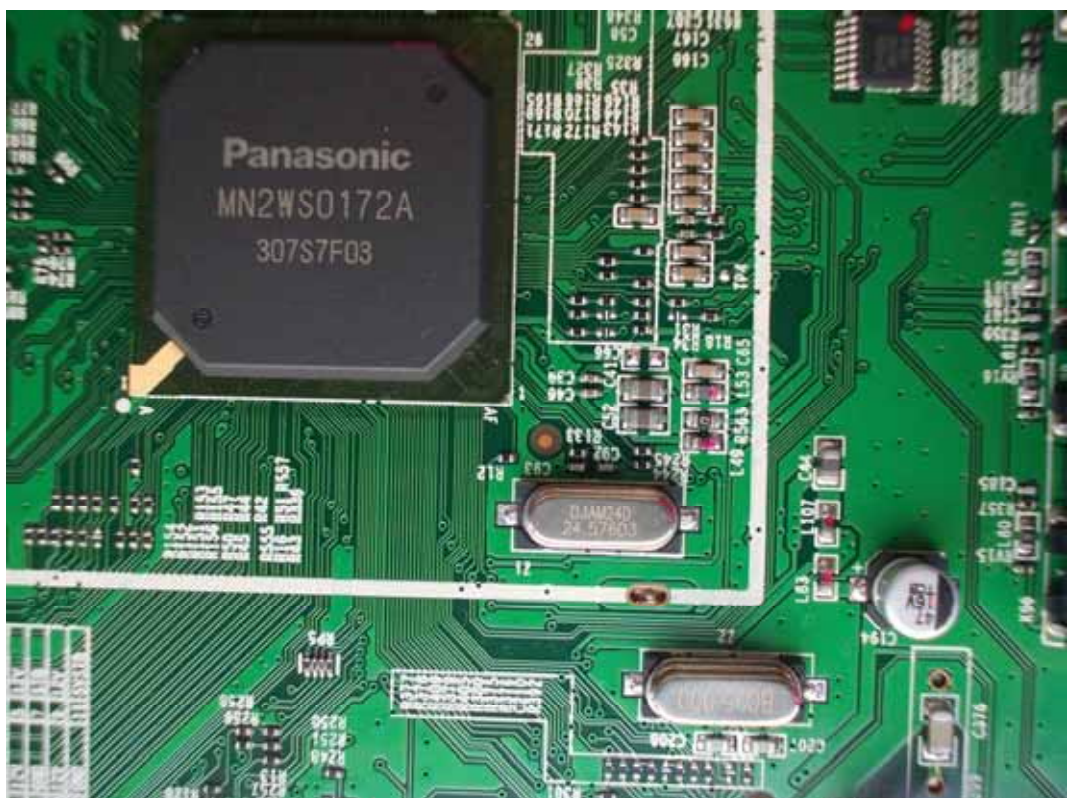
FIGURE 8 LED LCD TV (M/N: LTDN39K366MH) CHIP & CRYSTAL ON MAIN BOARD
