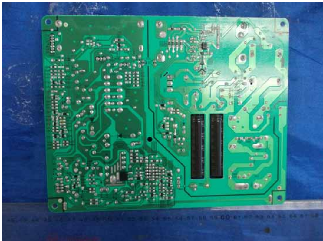
FIGURE 4 LED LCD TV (M/N: LTDN39K366MH) POWER BOARD (SOLDERED SIDE)
