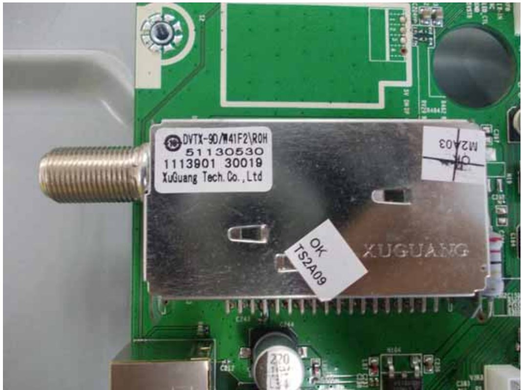
FIGURE 7 LED LCD TV (M/N: LTDN39K366MH) TUNER ON MAIN BOARD
