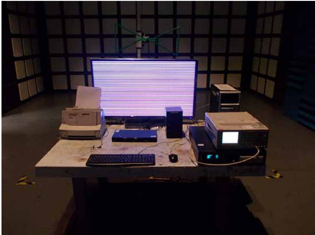
FRONT VIEW OF RADIATED EMISSION TEST
