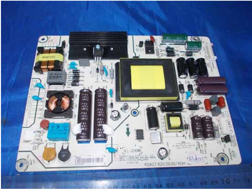
FIGURE 3 LED LCD TV (M/N: LTDN42A300MH) POWER BOARD (COMPONENT SIDE)
