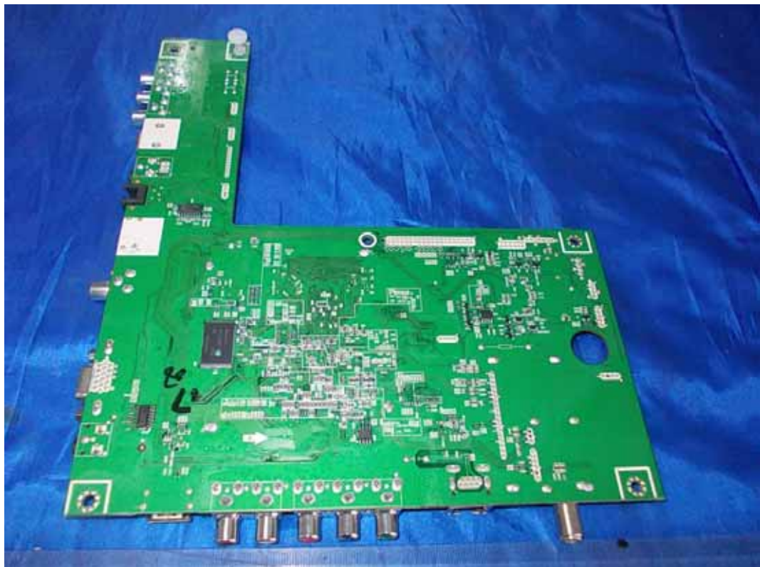
FIGURE 6 LED LCD TV (M/N: LTDN42A300MH) MAIN BOARD (SOLDERED SIDE)
