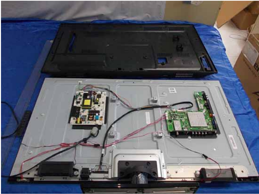
FIGURE 1 LED LCD TV (M/N: LTDN42A300MH) COVER REMOVED
