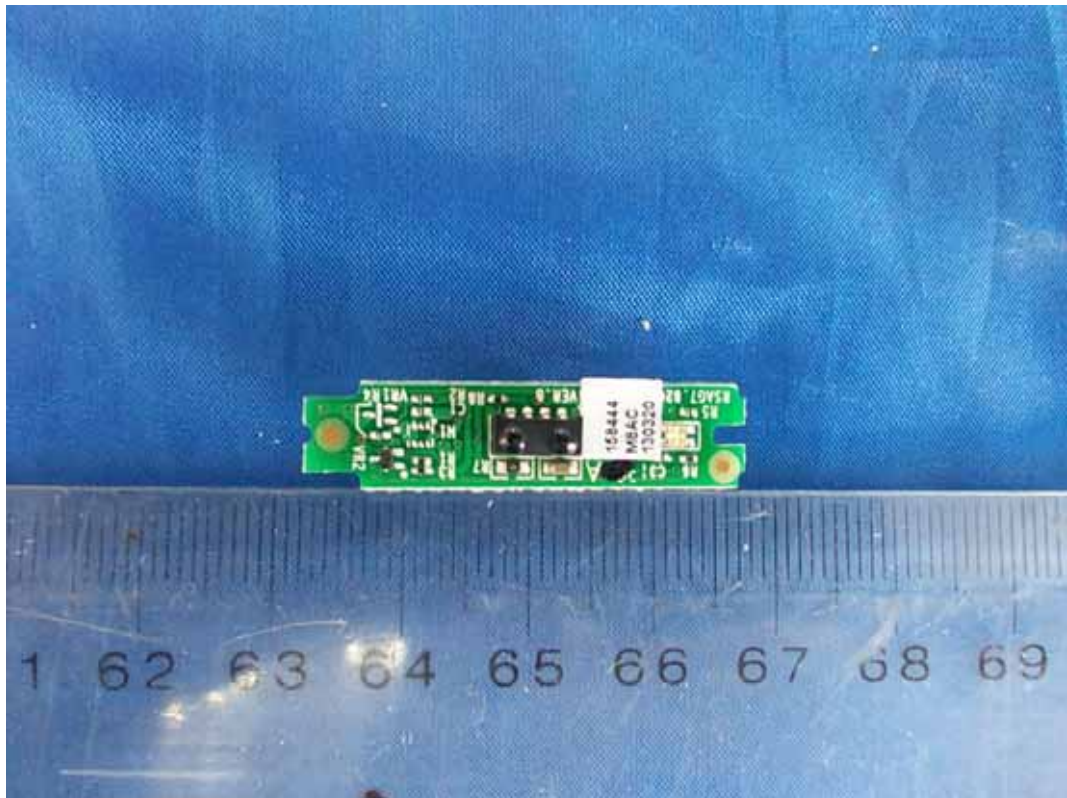
FIGURE 12 LED LCD TV (M/N: LTDN42A300MH) IR BOARD (COMPONENT SIDE)
