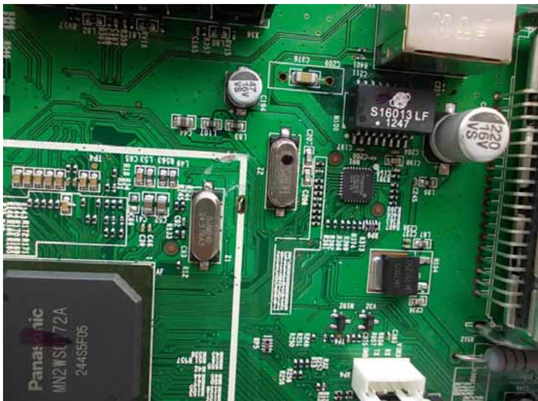
FIGURE 8 LED LCD TV (M/N: LTDN42A300MH) CRYSTAL #1/#2 ON MAIN BOARD
