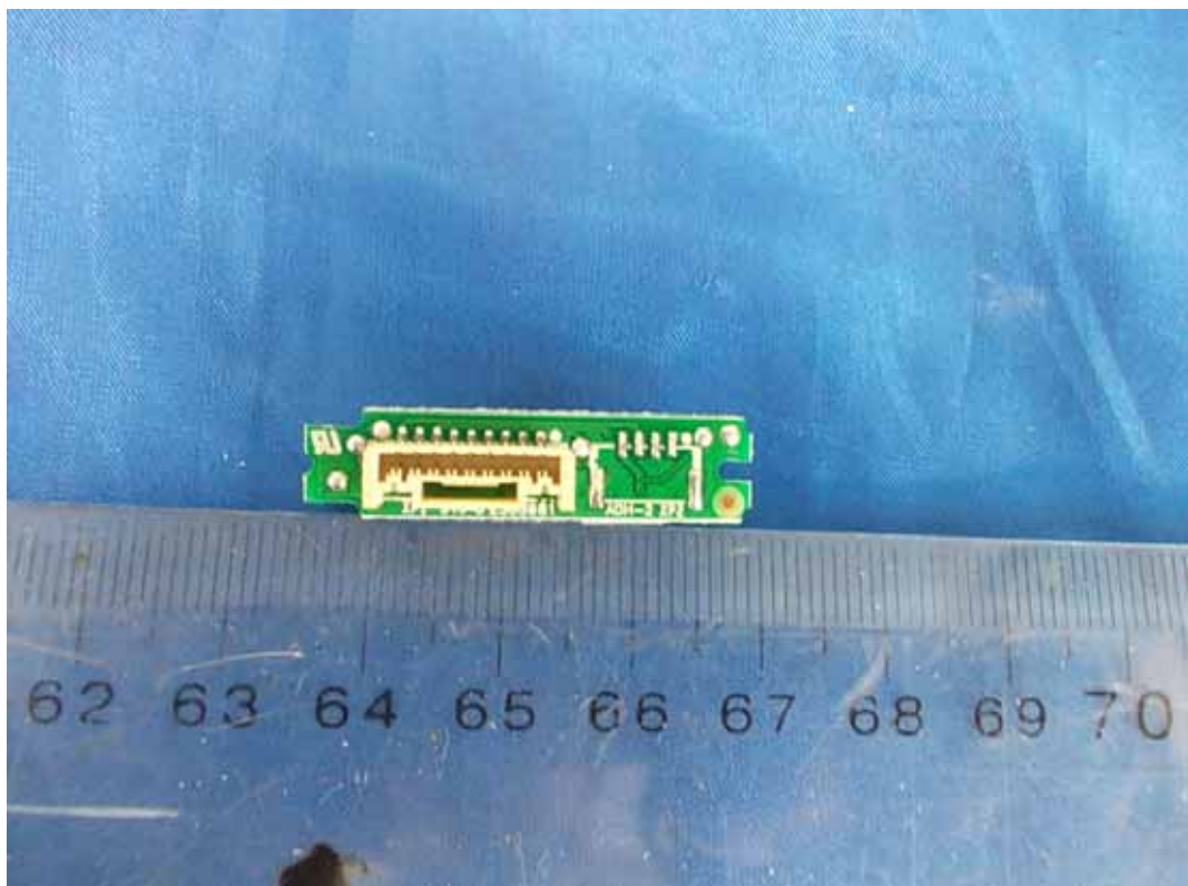
FIGURE 13 LED LCD TV (M/N: LTDN42A300MH) IR BOARD (SOLDERED SIDE)
