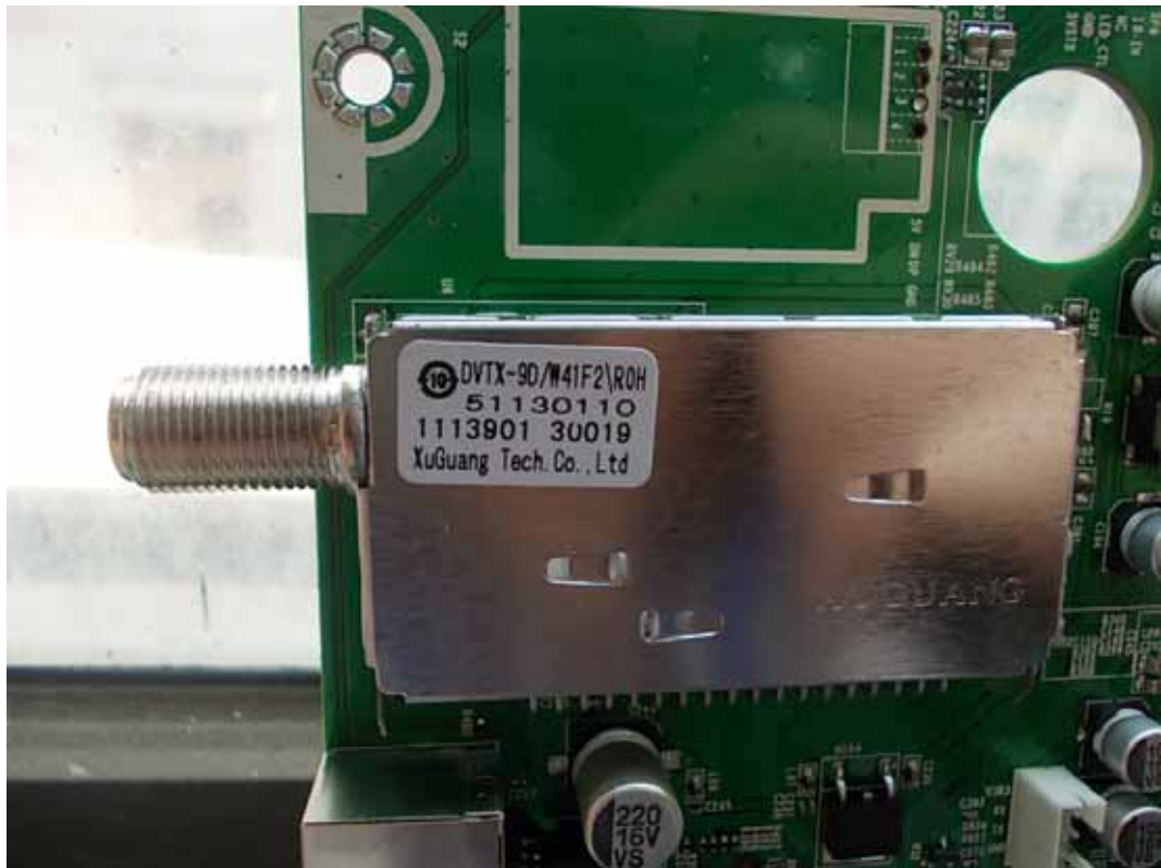
FIGURE 7 LED LCD TV (M/N: LTDN42A300MH) TUNER ON MAIN BOARD
