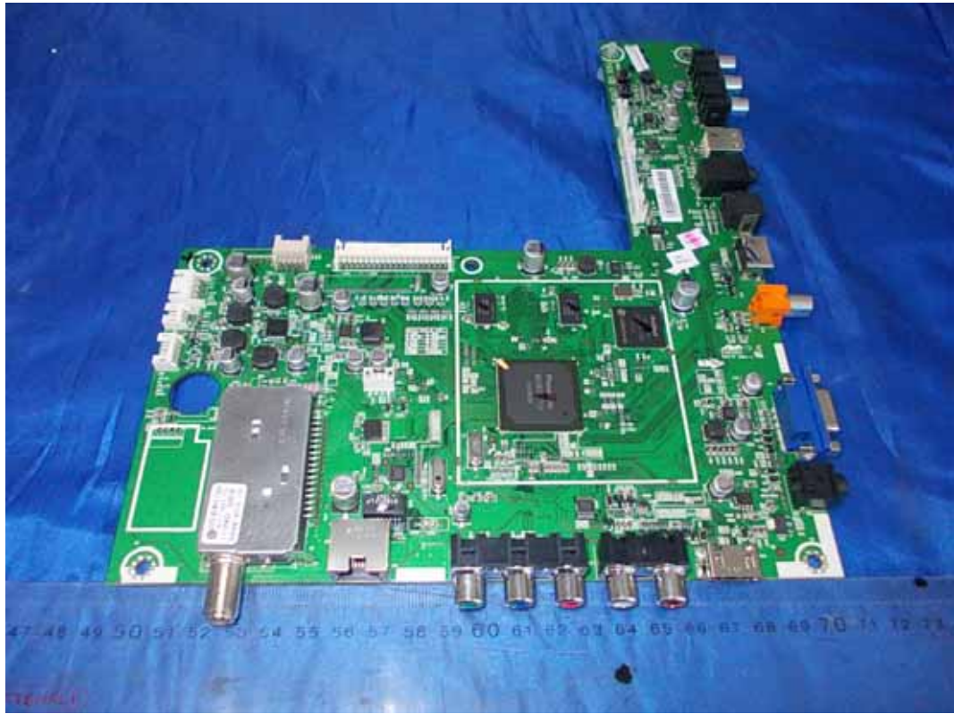
FIGURE 5 LED LCD TV (M/N: LTDN42A300MH) MAIN BOARD (COMPONENT SIDE)
