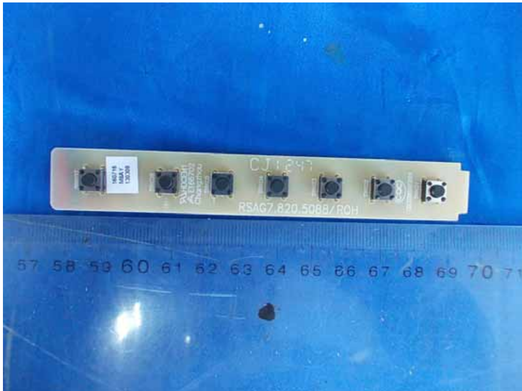
FIGURE 10 LED LCD TV (M/N: LTDN42A300MH) KEY BOARD (COMPONENT SIDE)
