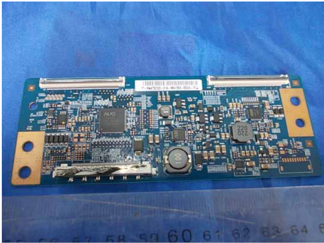
FIGURE 13 LED LCD TV (M/N: 46K360M) LCD PANEL CONTROL BOARD (COMPONENT SIDE)
