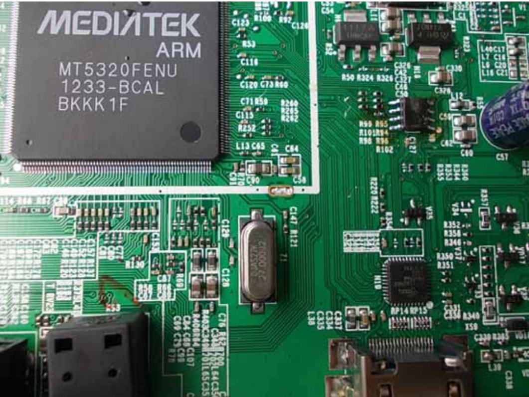
FIGURE 8 LED LCD TV (M/N: 46K360M) CHIP #1 & CRYSTAL ON MAIN BOARD
