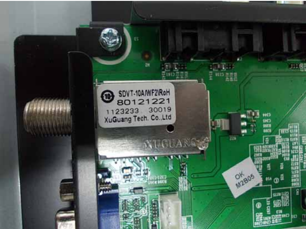
FIGURE 7 LED LCD TV (M/N: 46K360M) TUNER ON MAIN BOARD
