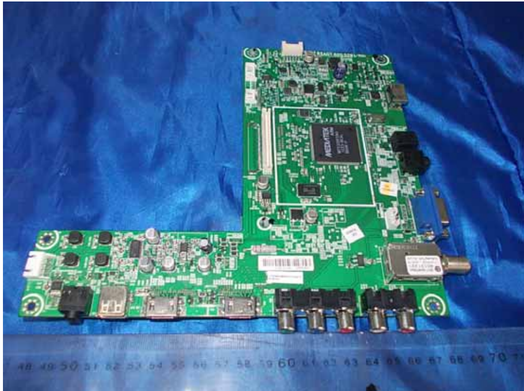
FIGURE 5 LED LCD TV (M/N: 46K360M) MAIN BOARD (COMPONENT SIDE)
