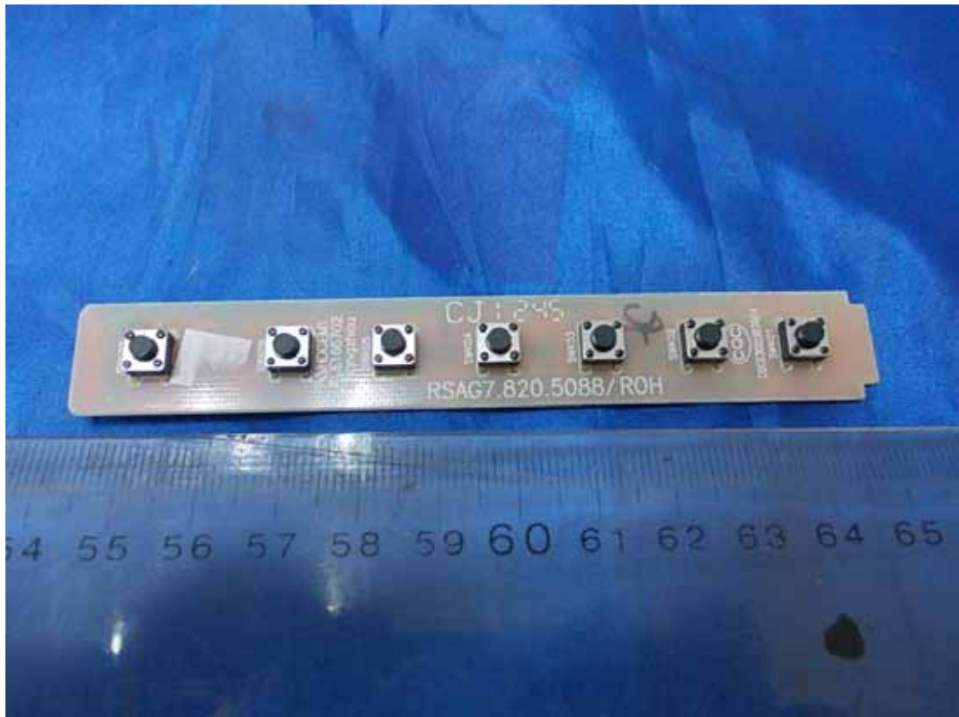
FIGURE 9 LED LCD TV (M/N: 46K360M) KEY BOARD (COMPONENT SIDE)
