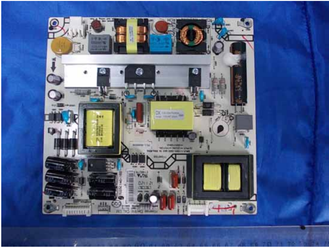
FIGURE 3 LED LCD TV (M/N: 46K360M) POWER BOARD (COMPONENT SIDE)
