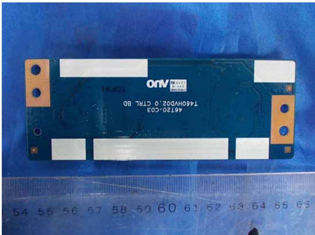
FIGURE 14 LED LCD TV (M/N: 46K360M) LCD PANEL CONTROL BOARD (SOLDERED SIDE)
