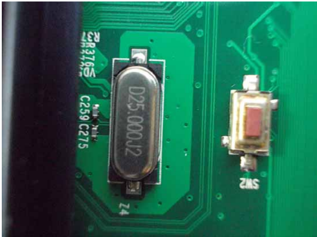
FIGURE 11 LED LCD TV (M/N: LTDN42K610XWUS3D) CRYSTAL #3 ON MAIN BOARD
