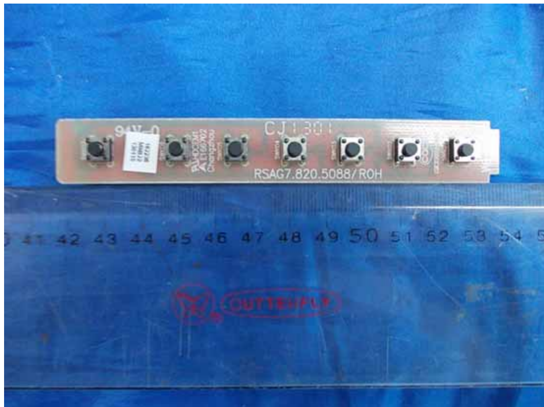
FIGURE 12 LED LCD TV (M/N: LTDN42K610XWUS3D) KEY BOARD (COMPONENT SIDE)
