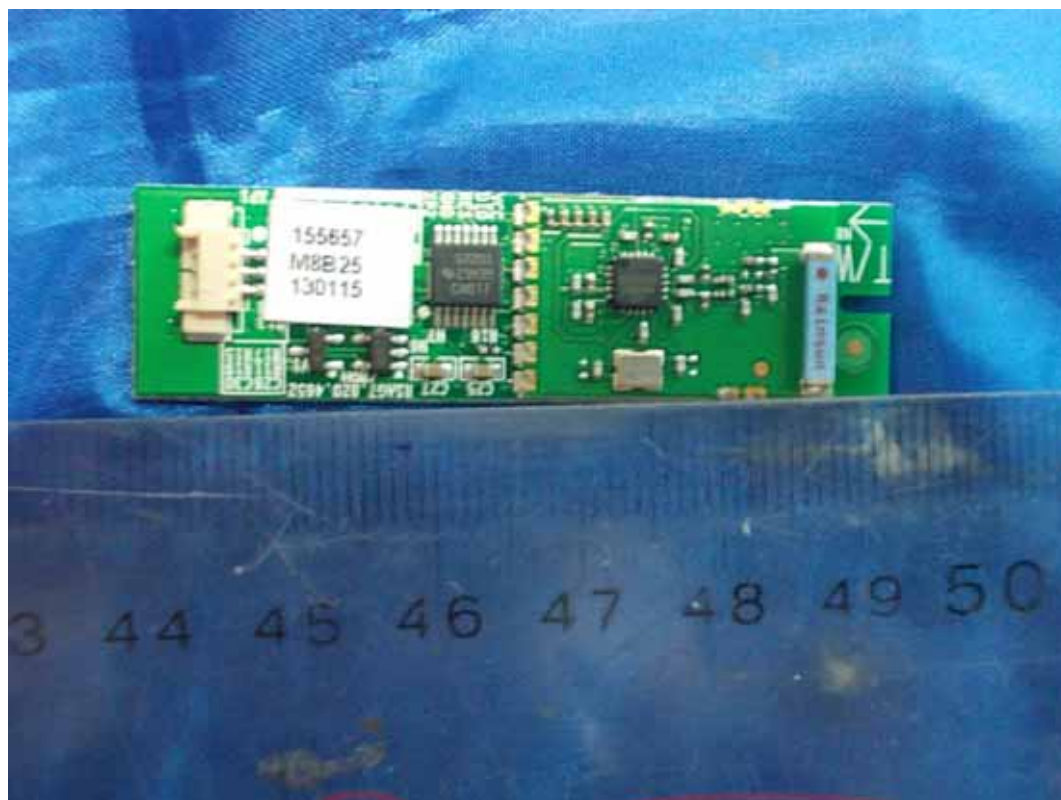
FIGURE 18 LED LCD TV (M/N: LTDN42K610XWUS3D) BOARD (COMPONENT SIDE)
