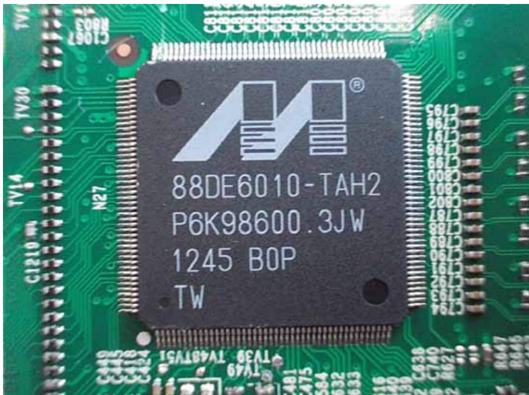
FIGURE 8 LED LCD TV (M/N: LTDN42K610XWUS3D) CHIP #1 ON MAIN BOARD
