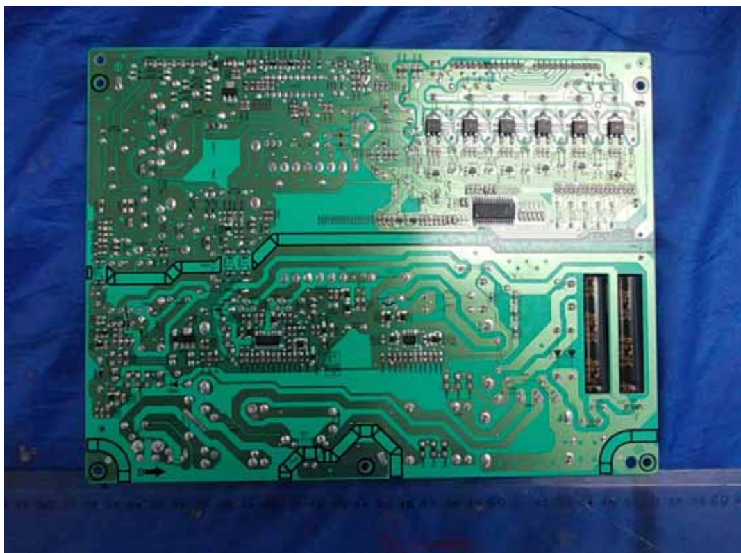
FIGURE 4 LED LCD TV (M/N: LTDN42K610XWUS3D) POWER BOARD (SOLDERED SIDE)
