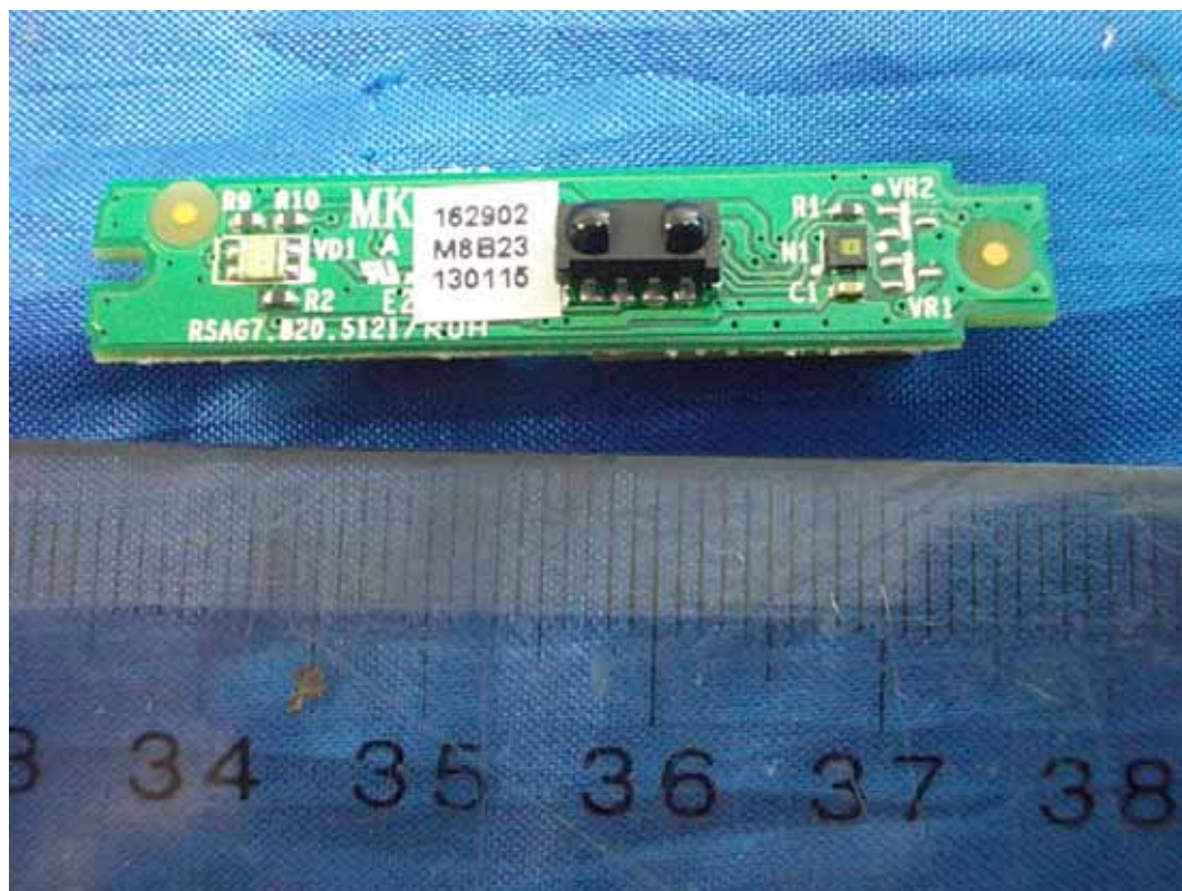
FIGURE 14 LED LCD TV (M/N: LTDN42K610XWUS3D) IR BOARD (COMPONENT SIDE)
