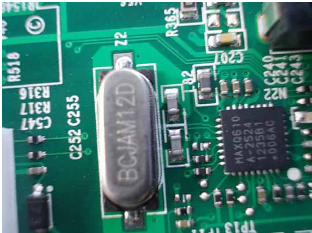
FIGURE 10 LED LCD TV (M/N: LTDN42K610XWUS3D) CHIP #3 & CRYSTAL #2 ON MAIN BOARD
