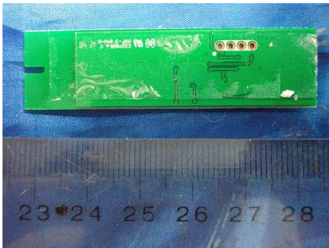
FIGURE 19 LED LCD TV (M/N: LTDN42K610XWUS3D) BOARD (SOLDERED SIDE)
