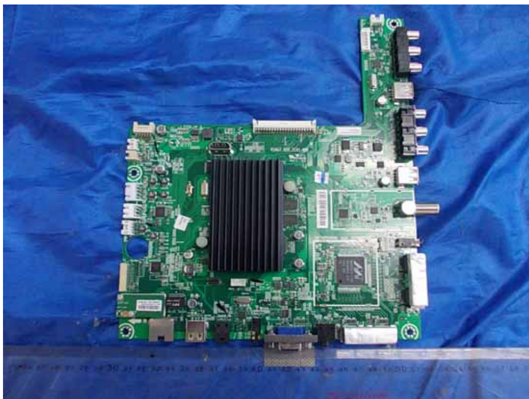
FIGURE 5 LED LCD TV (M/N: LTDN42K610XWUS3D) MAIN BOARD (COMPONENT SIDE)
