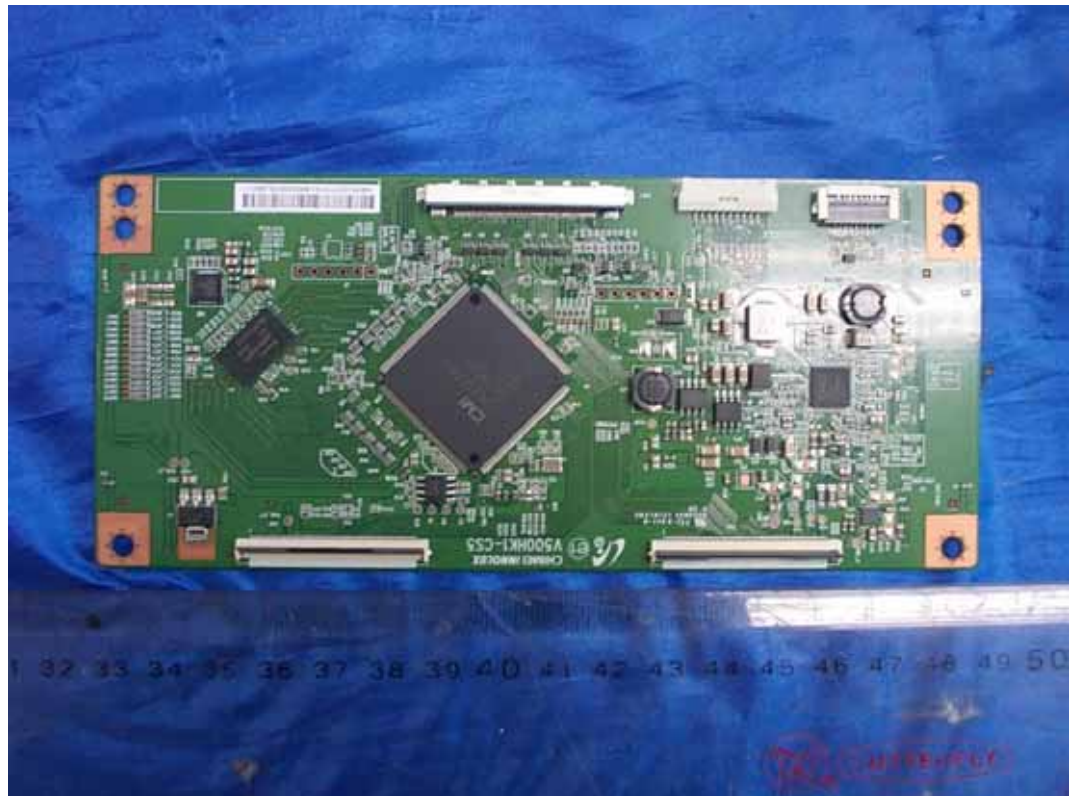
FIGURE 16 LED LCD TV (M/N: LTDN42K610XWUS3D) LCD PANEL CONTROL BOARD (COMPONENT SIDE)
