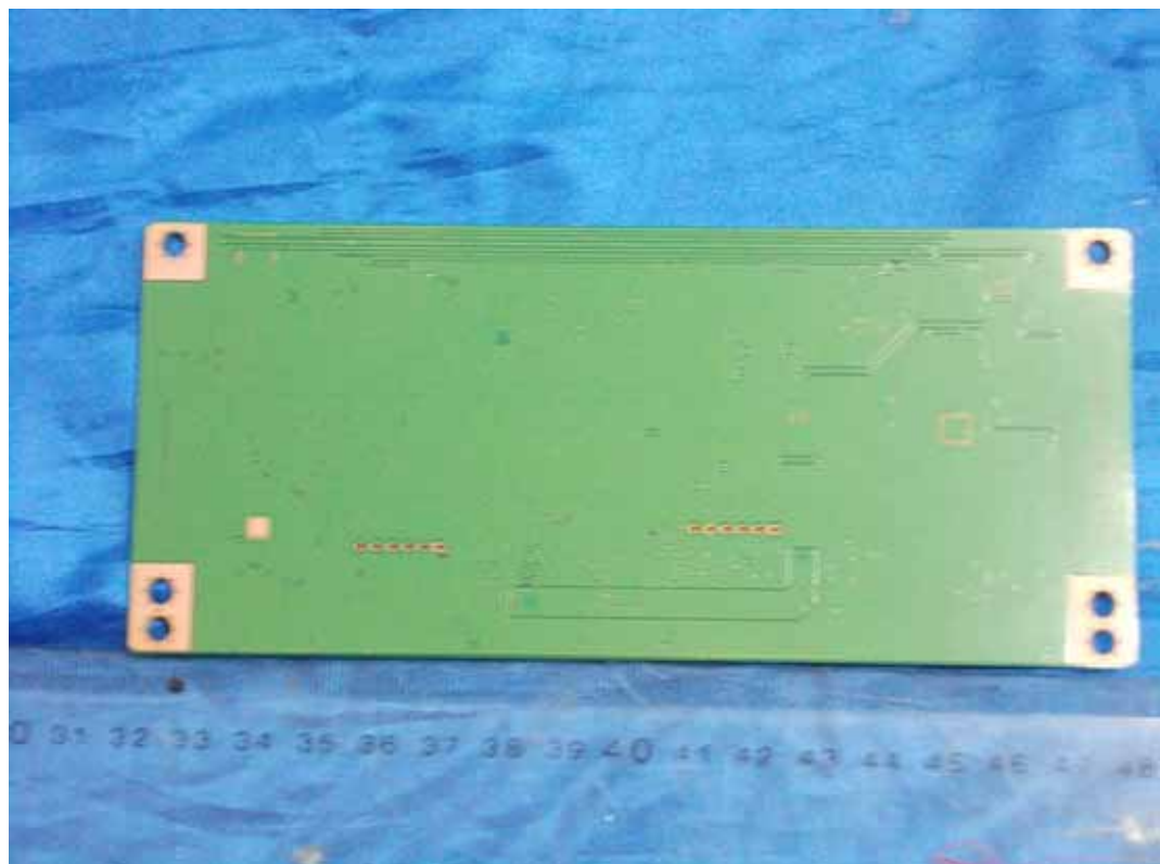
FIGURE 17 LED LCD TV (M/N: LTDN42K610XWUS3D) LCD PANEL CONTROL BOARD (SOLDERED SIDE)
