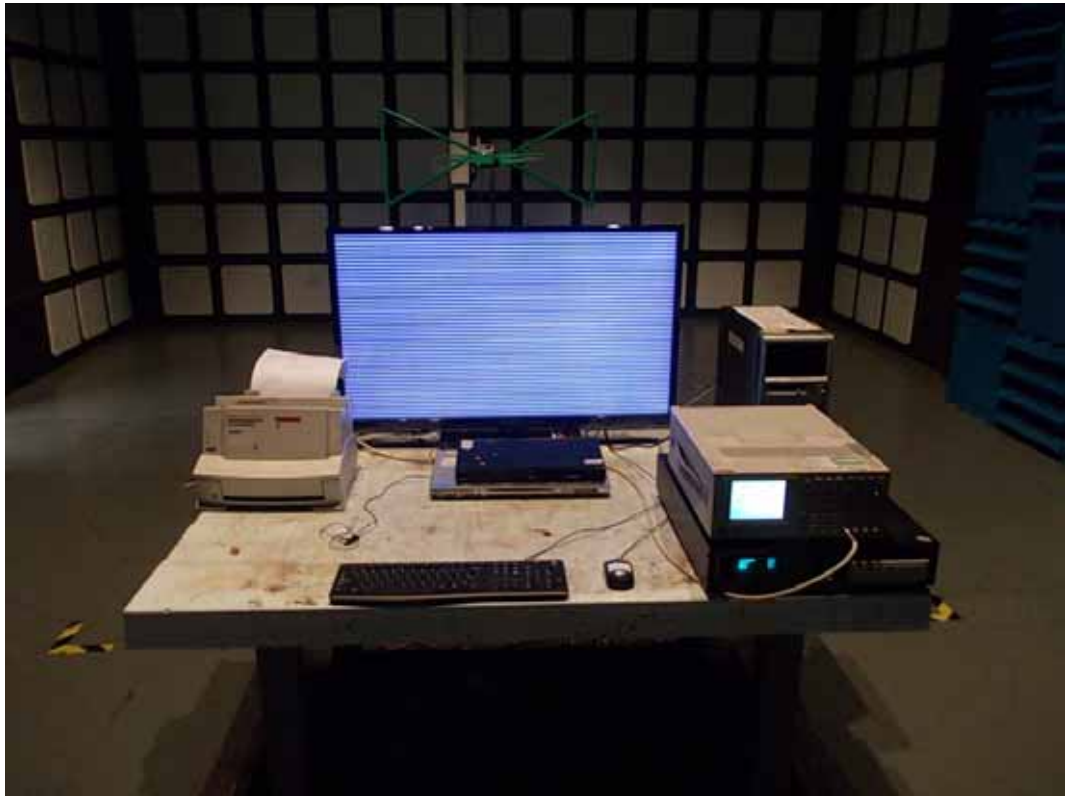
FRONT VIEW OF RADIATED EMISSION TEST
