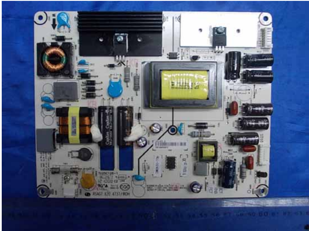
FIGURE 4 LED LCD TV (M/N: LTDN40K360MUS) POWER BOARD (COMPONENT SIDE)
