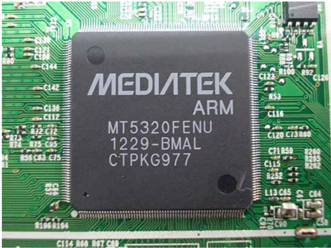
FIGURE 10 LED LCD TV (M/N: LTDN40K360MUS) CHIP ON MAIN BOARD
