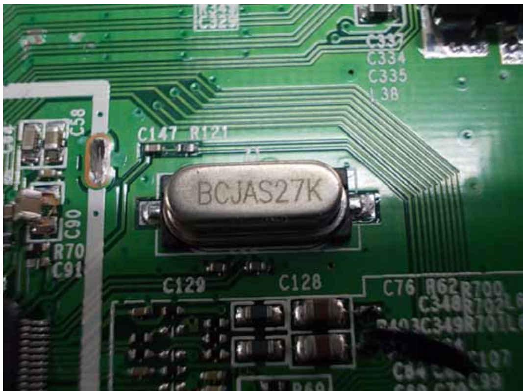
FIGURE 9 LED LCD TV (M/N: LTDN40K360MUS) CRYSTAL ON MAIN BOARD
