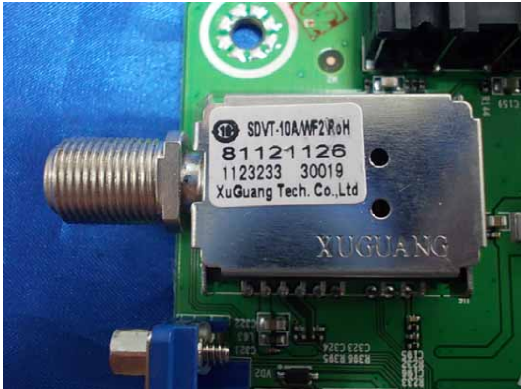
FIGURE 8 LED LCD TV (M/N: LTDN40K360MUS) TUNER ON MAIN BOARD
