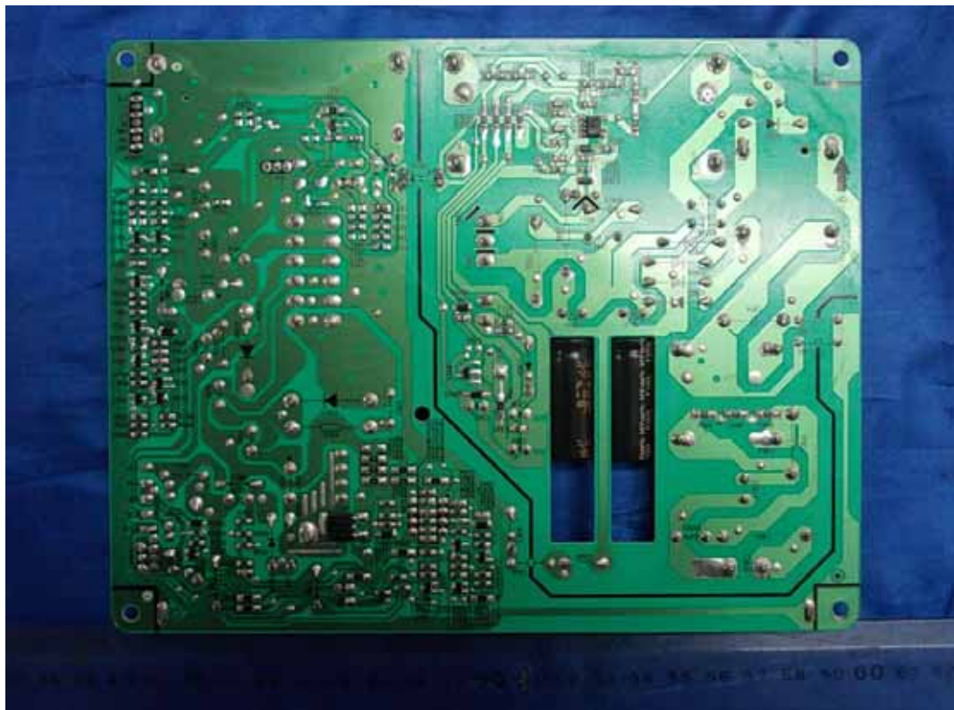
FIGURE 5 LED LCD TV (M/N: LTDN40K360MUS) POWER BOARD (SOLDERED SIDE)
