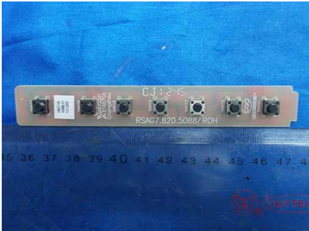
FIGURE 15 LED LCD TV (M/N: LTDN40K360MUS) KEY BOARD (COMPONENT SIDE)
