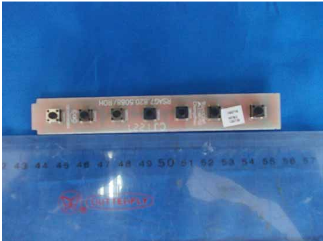
FIGURE 9 LED LCD TV (M/N: LTDN40K360US) KEY BOARD (COMPONENT SIDE)
