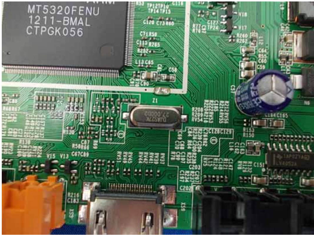
FIGURE 6 LED LCD TV (M/N: LTDN40K360US) CRYSTAL ON MAIN BOARD
