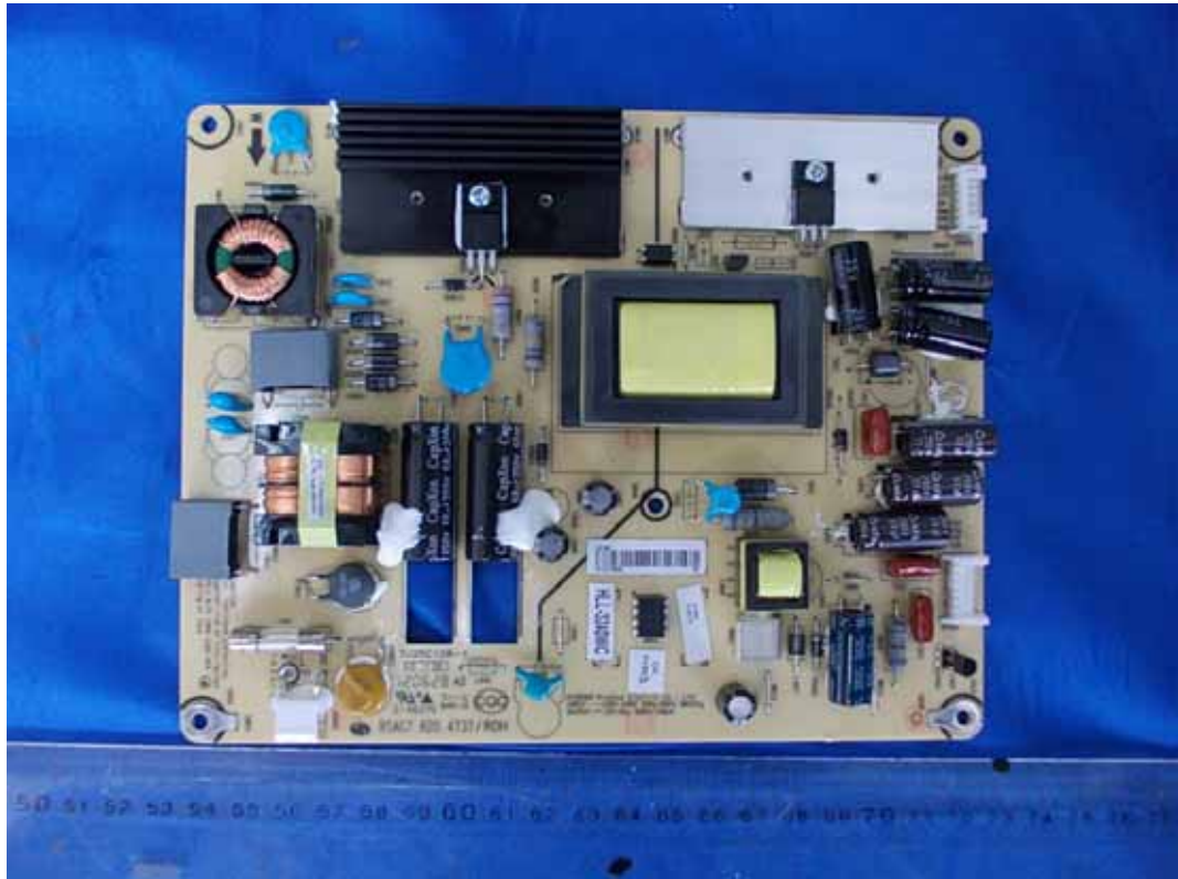
FIGURE 2 LED LCD TV (M/N: LTDN40K360US) POWER BOARD (COMPONENT SIDE)
