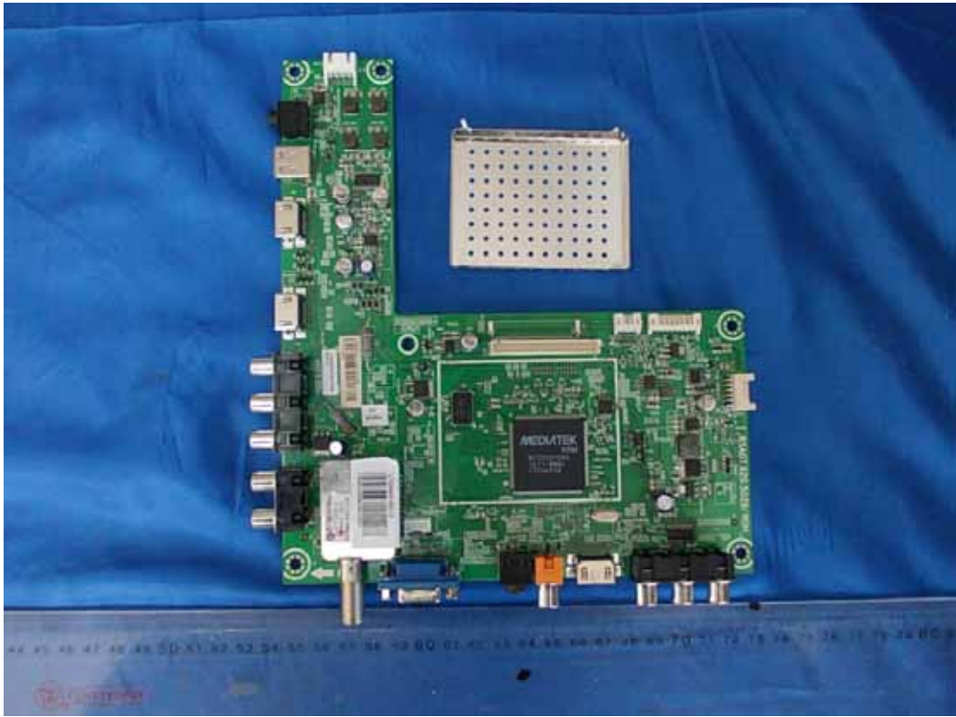
FIGURE 4 LED LCD TV (M/N: LTDN40K360US) MAIN BOARD (COMPONENT SIDE)
