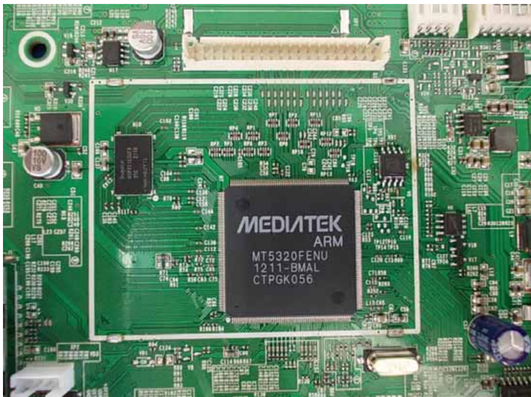
FIGURE 7 LED LCD TV (M/N: LTDN40K360US) CHIP ON MAIN BOARD
