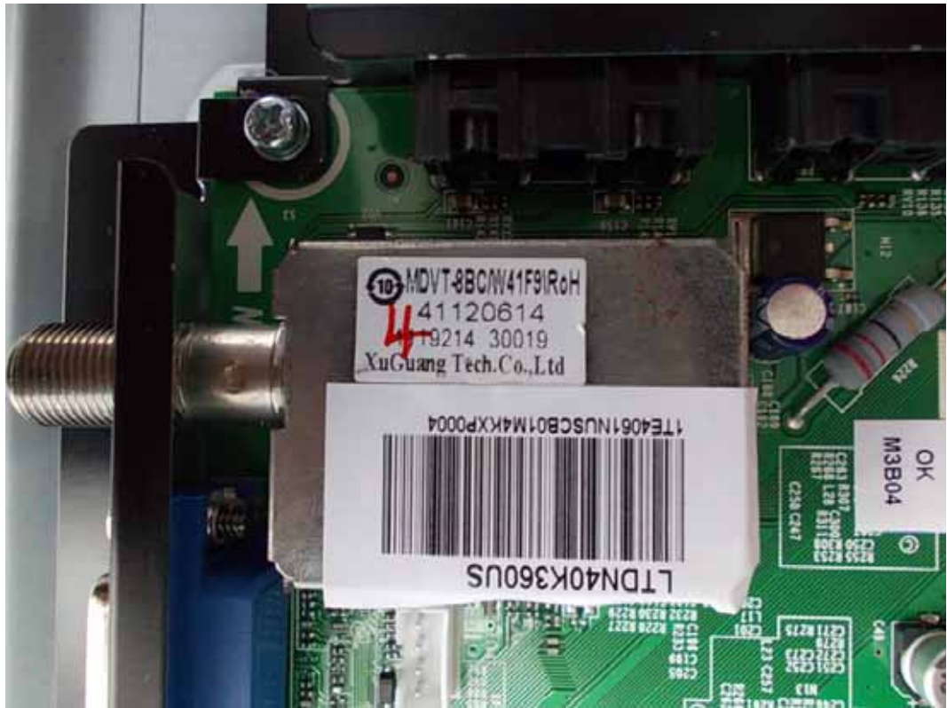
FIGURE 8 LED LCD TV (M/N: LTDN40K360US) TUNER ON MAIN BOARD
