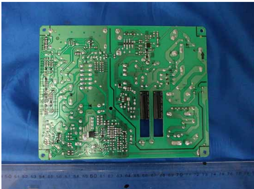
FIGURE 3 LED LCD TV (M/N: LTDN40K360US) POWER BOARD (SOLDERED SIDE)
