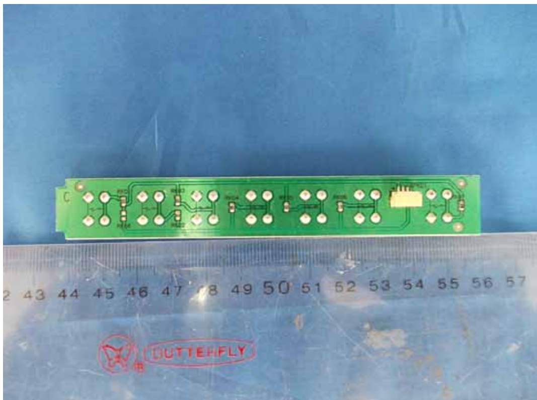
FIGURE 10 LED LCD TV (M/N: LTDN40K360US) KEY BOARD (SOLDERED SIDE)
