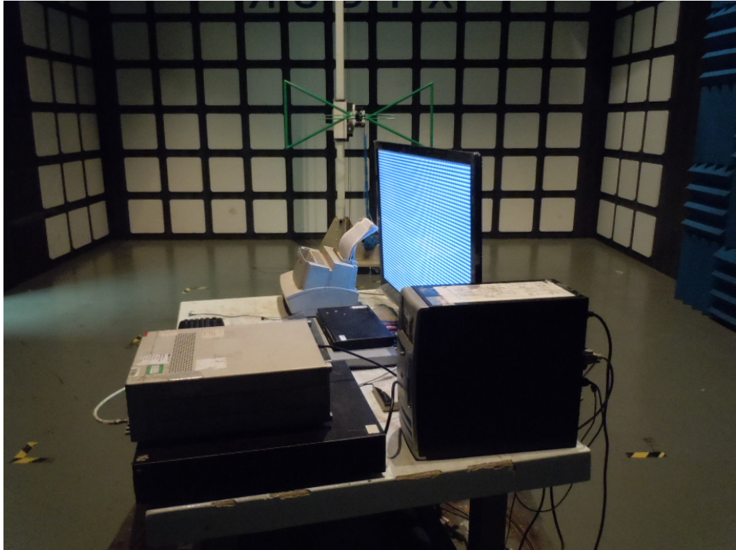
SETUP WITH MAXIMUM DETECTED EMISSION AT HORIZONTAL POLARIZATION (TEST MODE: D-SUB 640*480@60Hz)
