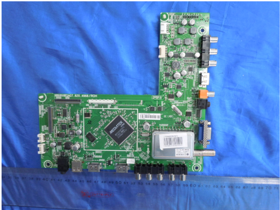
FIGURE 5 LED LCD TV (M/N: LTDN42K20US) MAIN BOARD (COMPONENT SIDE)
