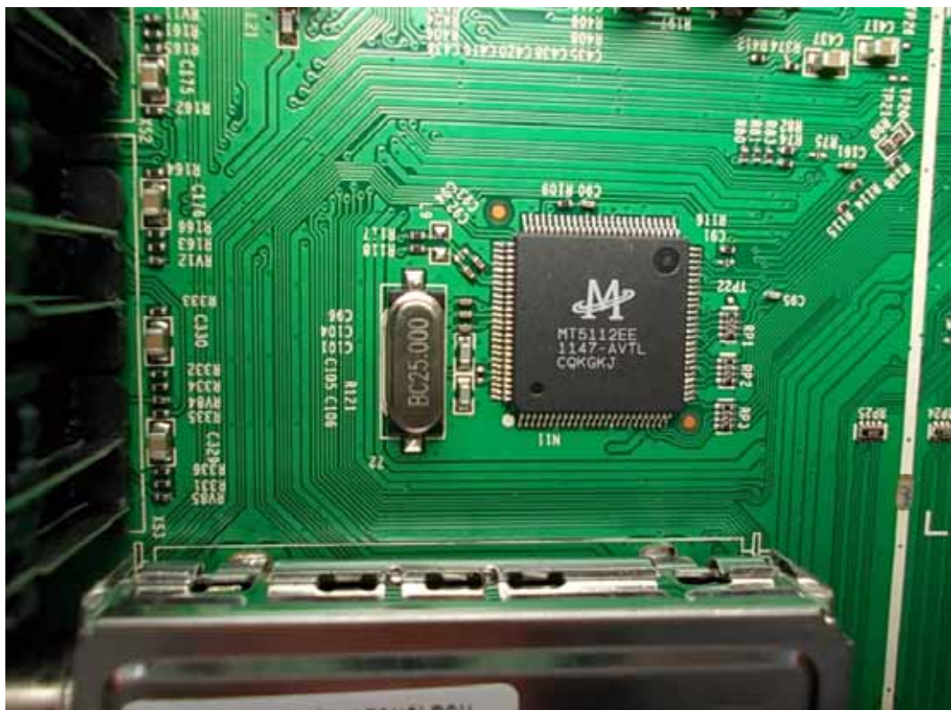
FIGURE 7 LED LCD TV (M/N: LTDN42D77WUS) CHIP#1 & CRYSTAL#1 ON MAIN BOARD
