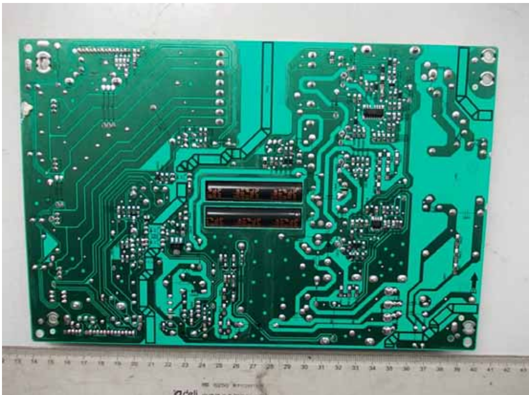
FIGURE 3 LED LCD TV (M/N: LTDN42D77WUS) POWER BOARD (SOLDERED SIDE)
