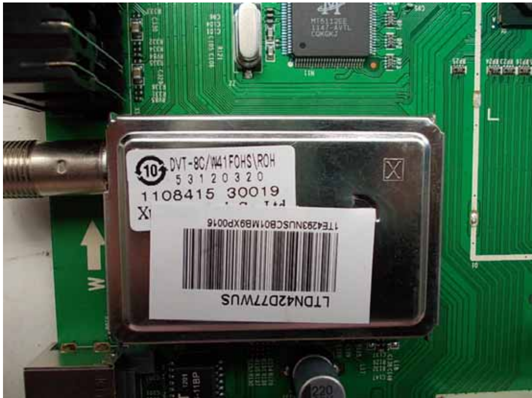
FIGURE 6 LED LCD TV (M/N: LTDN42D77WUS) TUNER ON MAIN BOARD
