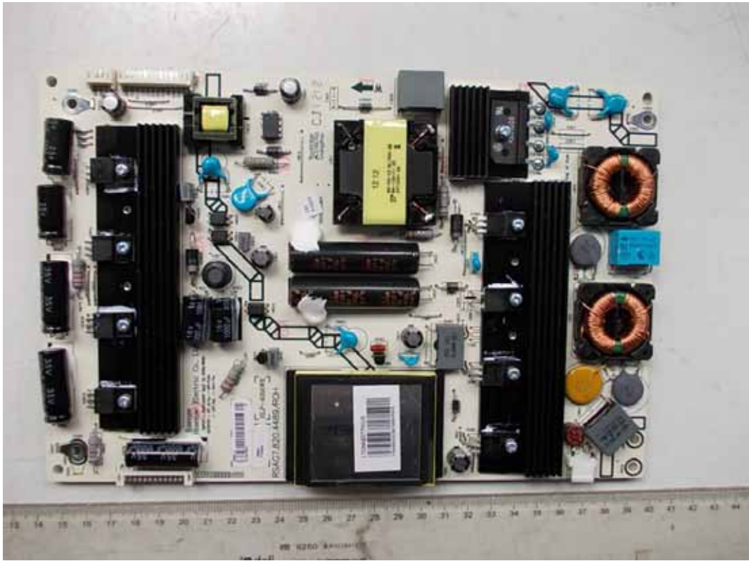
FIGURE 2 LED LCD TV (M/N: LTDN42D77WUS) POWER BOARD (COMPONENT SIDE)
