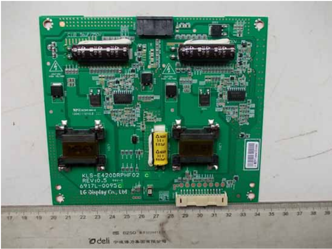
FIGURE 16 LED LCD TV (M/N: LTDN42D77WUS) HIGH VOLTAGE SIGNAL BOARD (COMPONENT SIDE)
