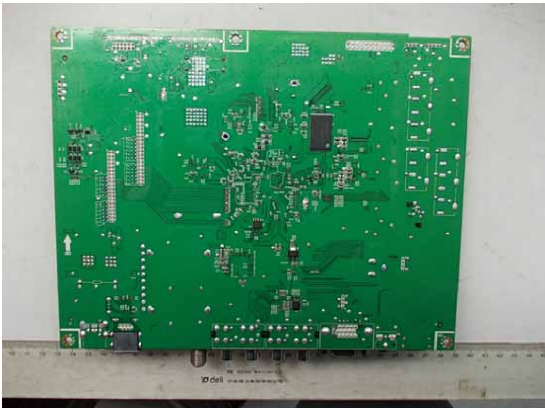
FIGURE 5 LED LCD TV (M/N: LTDN42D77WUS) MAIN BOARD (SOLDERED SIDE)
