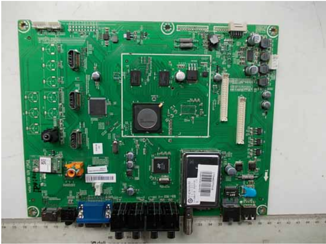
FIGURE 4 LED LCD TV (M/N: LTDN42D77WUS) MAIN BOARD (COMPONENT SIDE)
