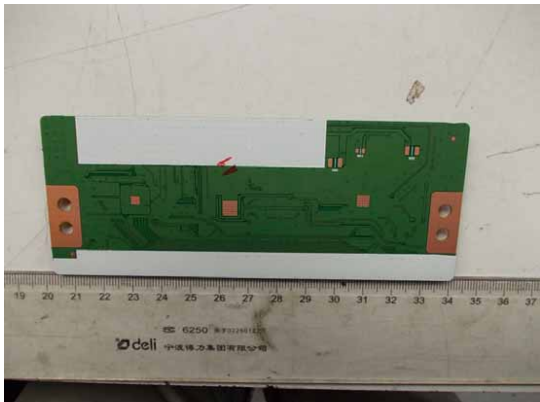
FIGURE 15 LED LCD TV (M/N: LTDN42D77WUS) LCD PANEL CONTROL BOARD (SOLDERED SIDE)
