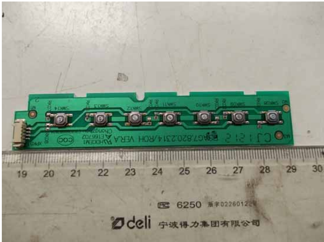
FIGURE 10 LED LCD TV (M/N: LTDN42D77WUS) KEY BOARD (COMPONENT SIDE)
