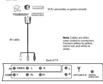
3 Connect the audio connectors of the AV cable (the red and white connectors) to the AV OUT AUDIO jacks of the external device, then connect them to the AV IN L and R jacks on the back of your TV.
