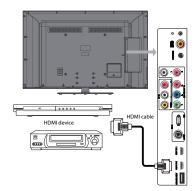
Note: To connect a DVI device, use a DVI to HDMI adapter cable to connect to the HDMI jack on the TV, then connect an audio cable to the PC IN AUDIO jack on the back of the TV.
