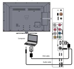
Note: The VGA cable will not supplied with product. We strongly recommend to use VGA cable with 2 cores as shown in the figure.
