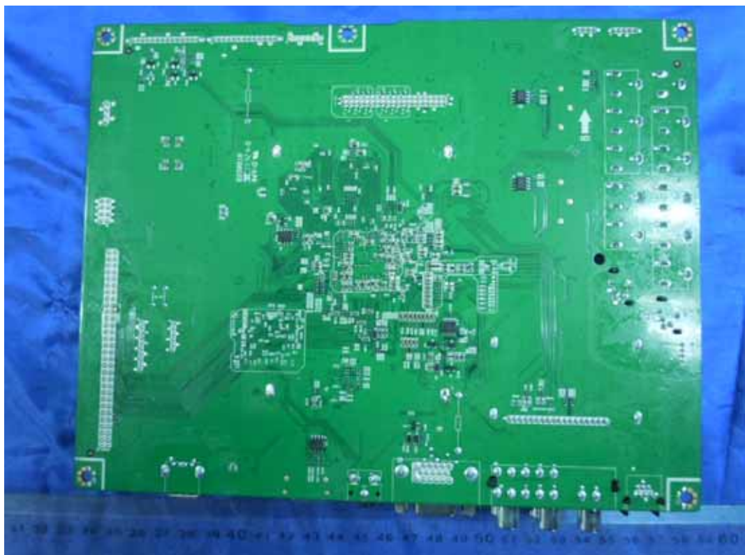
FIGURE 6 LCD TV (M/N: LTDN42V77KMH) MAIN BOARD (SOLDERED SIDE)
