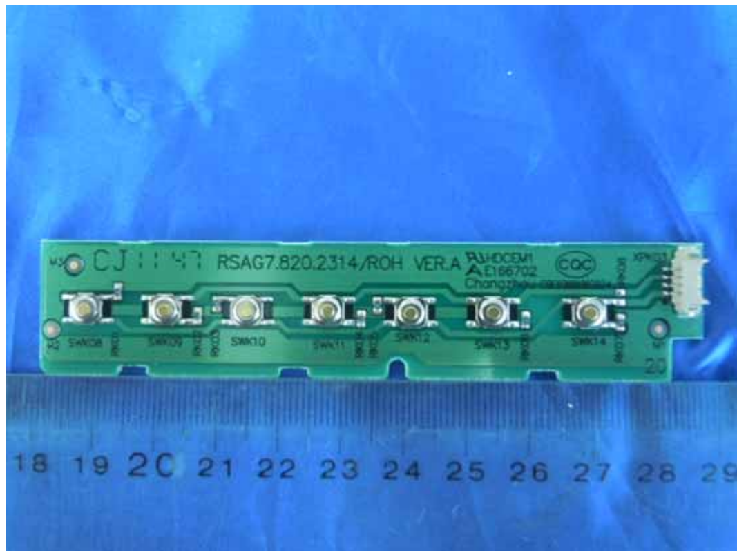
FIGURE 13 LCD TV (M/N: LTDN42V77KMH) KEY BOARD (COMPONENT SIDE)
