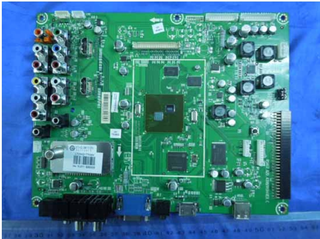
FIGURE 5 LCD TV (M/N: LTDN42V77KMH) MAIN BOARD (COMPONENT SIDE)
