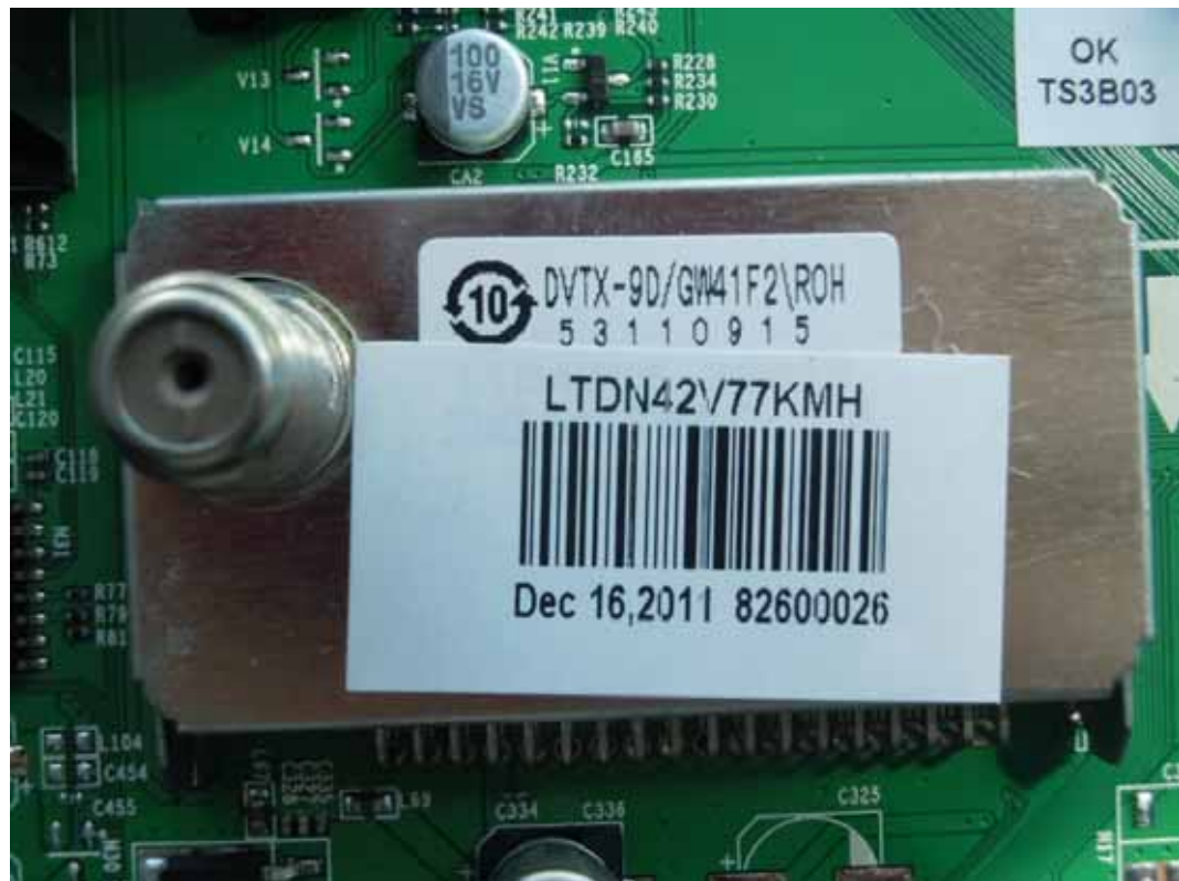
FIGURE 7 LCD TV (M/N: LTDN42V77KMH) TUNER ON MAIN BOARD
