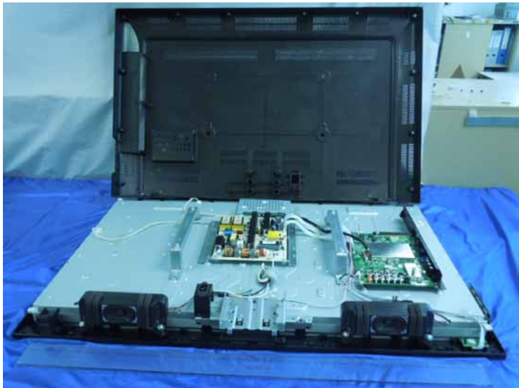
FIGURE 1 LCD TV (M/N: LTDN42V77KMH) COVER REMOVED
