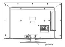
4 Carefully lift the TV into an upright position.
