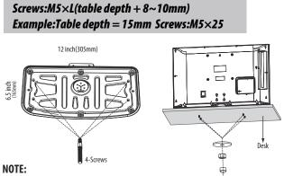
Be sure to follow the instructions, in correct installation of the stand (pedestal) may result in the TV falling over.
