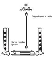
**3** Connect the other end of the audio cable to the digital coaxial input jack on the home theater system.
