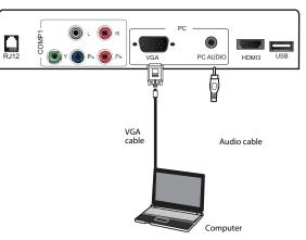
**3** Connect one end of an audio cable with a stereo mini-plug (not included) to the **PC AUDIO** jack on the side of the TV, then connect the other end of the cable to the **AUDIO OUT** jack on the computer.
