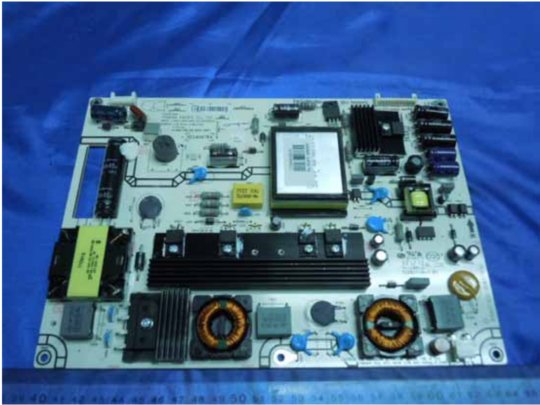
FIGURE 2 LED LCD TV (M/N: LTDN42K20US) POWER BOARD (COMPONENT SIDE)
