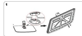
Make sure the front of the stand column match the front of the base plate. Insert the stand column onto the base plate, aligning the groove in the column with the ridge in the base plate. Secure the stand column to the base plate with three screws (M5 x12).
