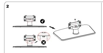
Assemble the stand cover and the stand column well with appropriate strength(" $\sqrt{}$ " is right and "x" is wrong).
