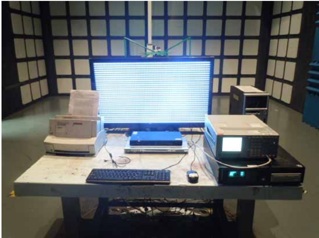
FRONT VIEW OF RADIATED EMISSION TEST
