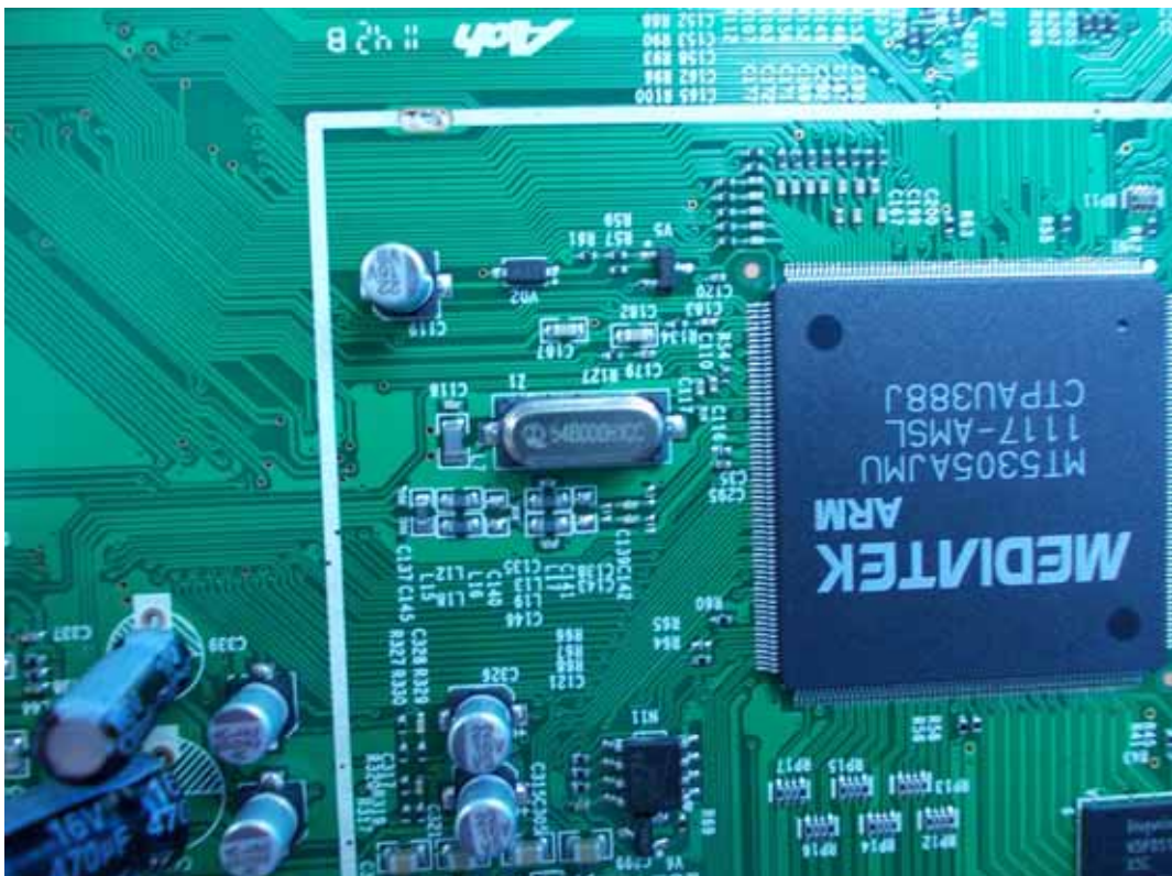
FIGURE 7 LCD TV (M/N: LTDN39V77US) CHIP & CRYSTAL ON MAIN BOARD
