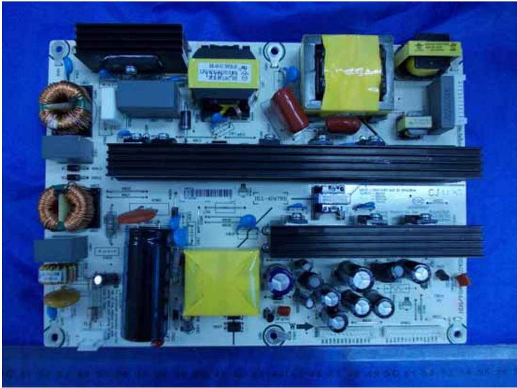
FIGURE 2 LCD TV (M/N: LTDN39V77US) POWER BOARD (COMPONENT SIDE)
