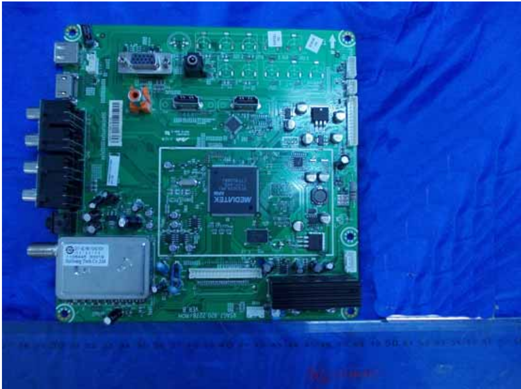
FIGURE 4 LCD TV (M/N: LTDN39V77US) MAIN BOARD (COMPONENT SIDE)
