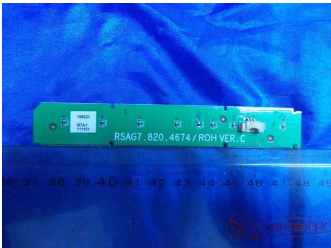
FIGURE 9 LCD TV (M/N: LTDN39V77US) KEY BOARD (SOLDERED SIDE)
