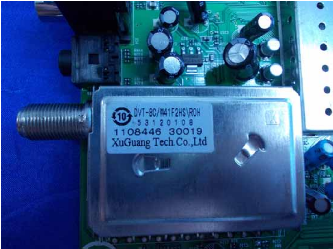
FIGURE 6 LCD TV (M/N: LTDN39V77US) TUNER ON MAIN BOARD
