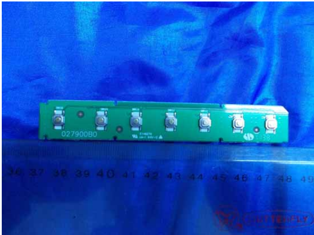
FIGURE 8 LCD TV (M/N: LTDN39V77US) KEY BOARD (COMPONENT SIDE)
