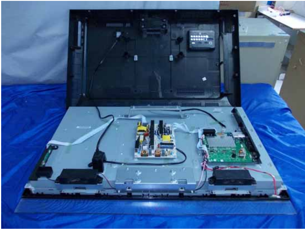
FIGURE 1 LCD TV (M/N: LTDN39V77US) COVER REMOVED
