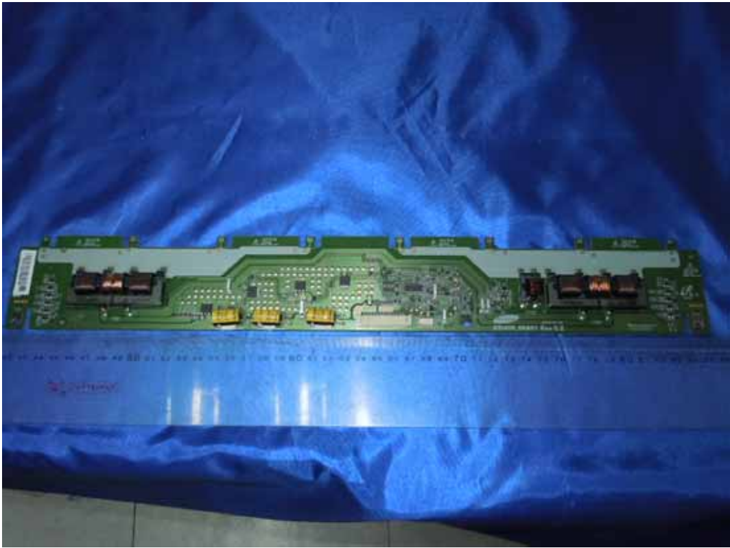
FIGURE 13 LCD TV (M/N: LTDN40V87HUS) CONTROL BOARD (COMPONENT SIDE)
