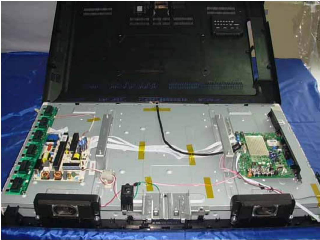
FIGURE 1 LCD TV (M/N: LTDN42V77MH) COVER REMOVED
