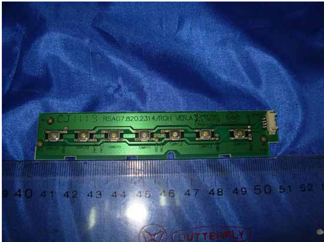
FIGURE 12 LCD TV (M/N: LTDN42V77MH) KEY BOARD (COMPONENT SIDE)
