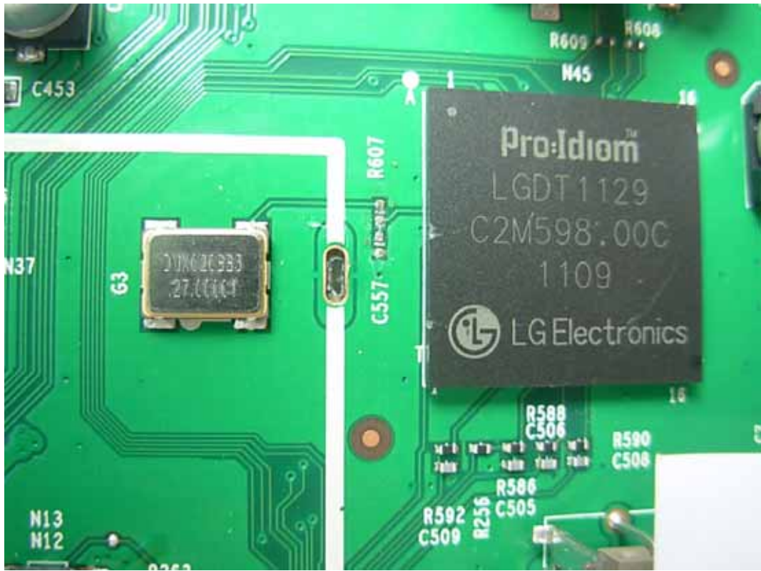
FIGURE 8 LCD TV (M/N: LTDN42V77MH) CHIP #2 & CRYSTAL #2 ON MAIN BOARD
