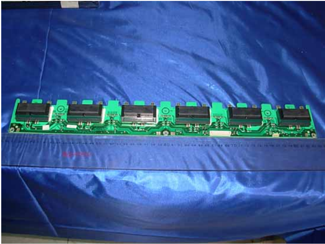
FIGURE 10 LCD TV (M/N: LTDN42V77MH) HIGH VOLTAGE SIGNAL BOARD (COMPONENT SIDE)
