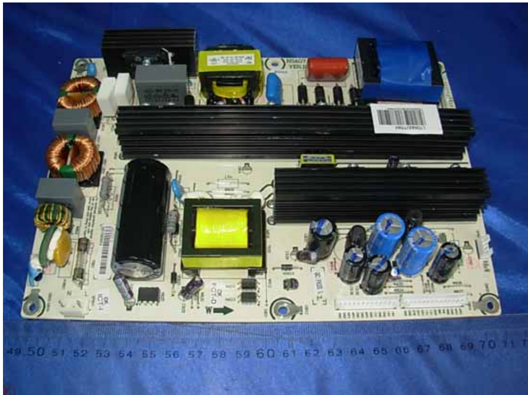
FIGURE 2 LCD TV (M/N: LTDN42V77MH) POWER BOARD (COMPONENT SIDE)
