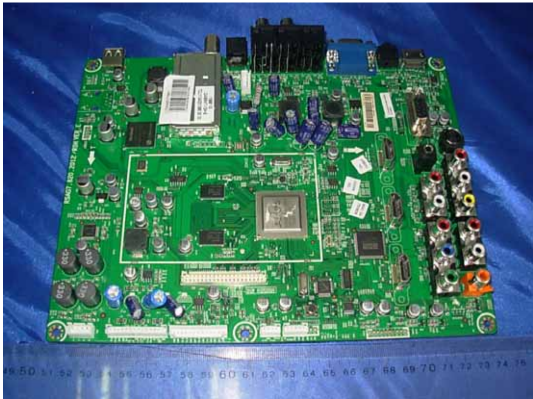
FIGURE 4 LCD TV (M/N: LTDN42V77MH) MAIN BOARD (COMPONENT SIDE)
