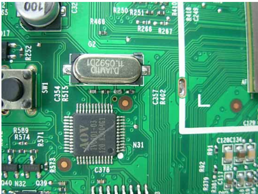
FIGURE 9 LCD TV (M/N: LTDN42V77MH) CHIP #3 & CRYSTAL #3 ON MAIN BOARD
