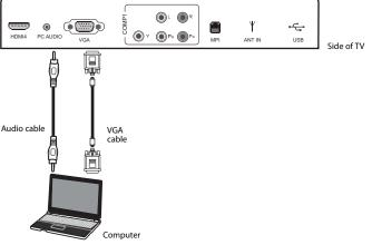
3 Connect one end of an audio cable with a stereo mini-plug (not included) to the **PC AUDIO** jack on the side of the TV, then connect the other end of the cable to the **AUDIO OUT** jack on the computer.
