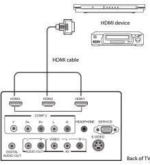
Note: To connect a DVI device, use a DVI to HDMI adapter cable to connect to the HDMI jack on the TV, then connect an audio cable to the PC AUDIO jack on the side of the TV.
