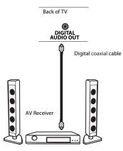
**3** Connect the other end of the audio cable to the digital coaxial input jack on the AV receiver.
