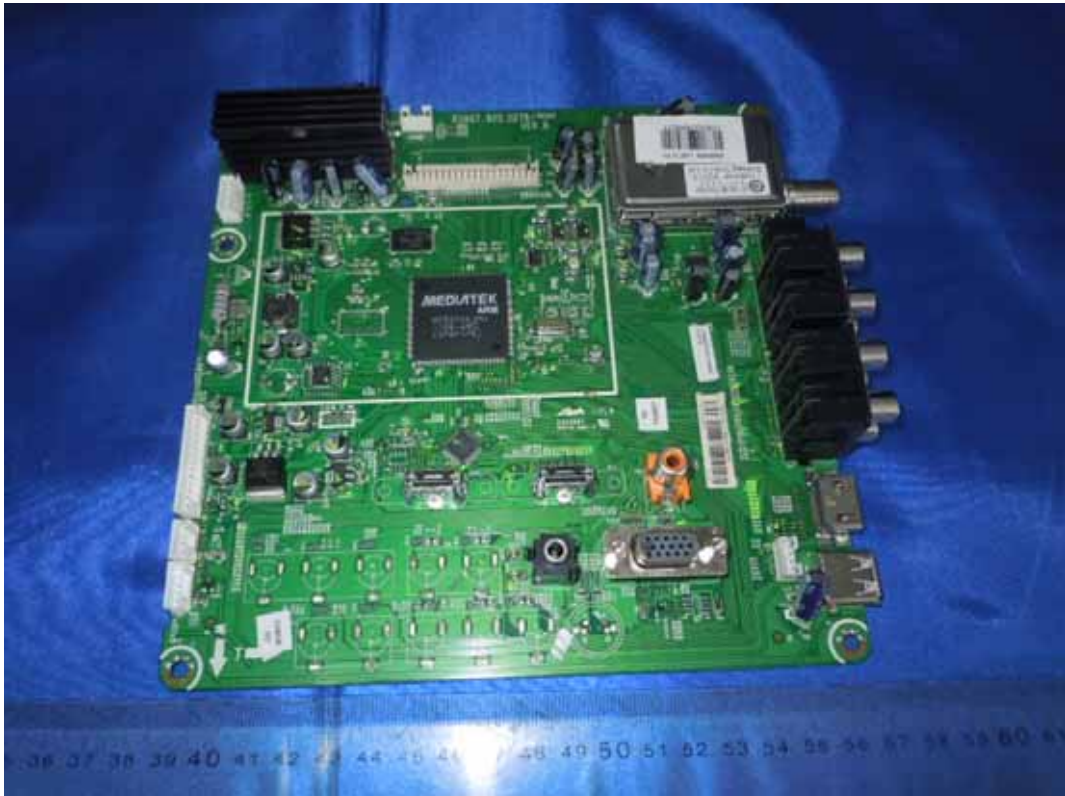
FIGURE 5 LCD TV (M/N: LTDN42V77US) MAIN BOARD (COMPONENT SIDE)
