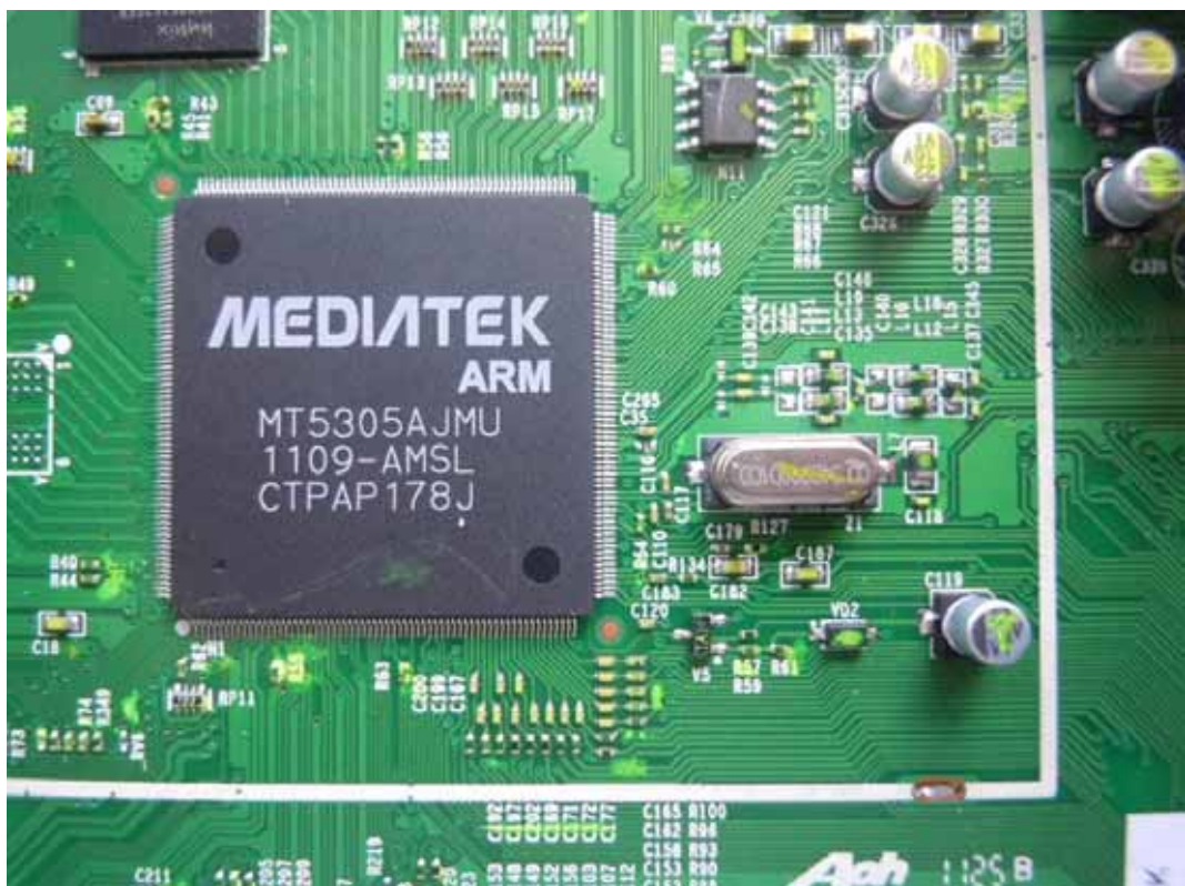
FIGURE 8 LCD TV (M/N: LTDN42V77US) CHIP & CRYSTAL ON MAIN BOARD
