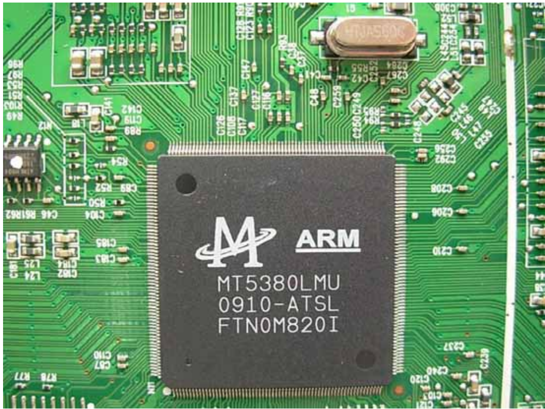
FIGURE 4 LCD TV (M/N: LTDN42W58US) CHIP & CRYSTAL ON MAIN BOARD
