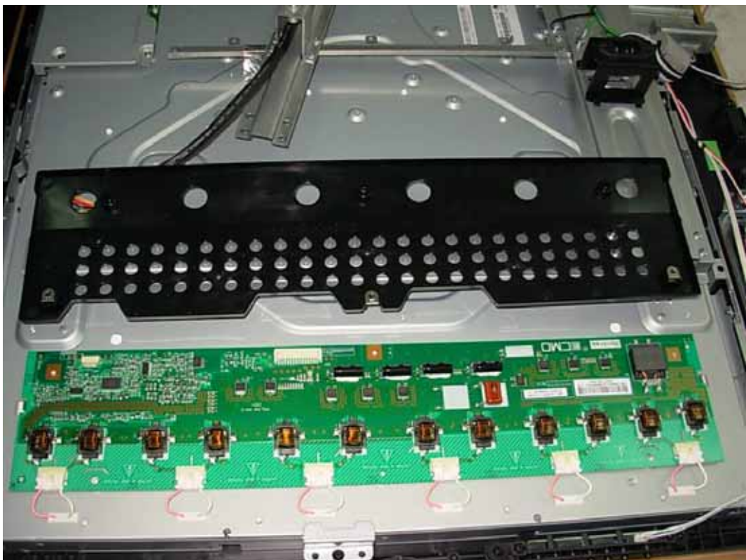
FIGURE 13 LCD TV (M/N: LTDN42W58US) INVERTER COVER REMOVED
