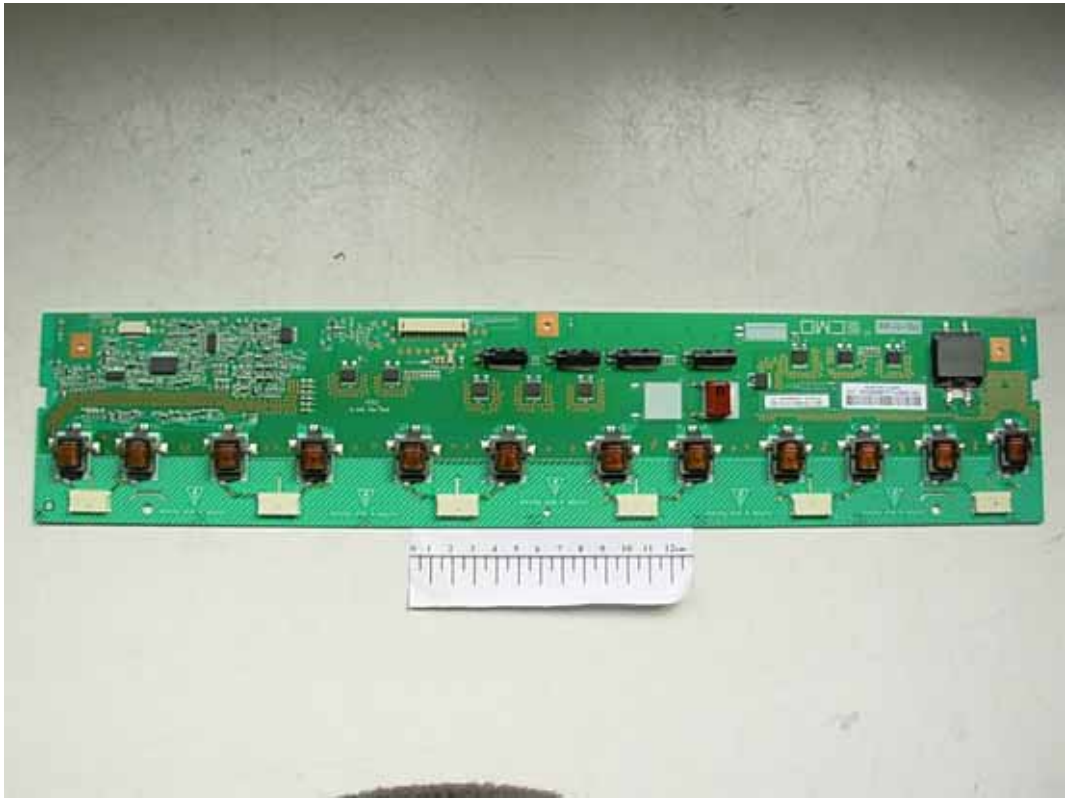
FIGURE 14 LCD TV (M/N: LTDN42W58US) INVERTER (COMPONENT SIDE)
