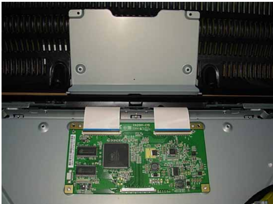
FIGURE 17 LCD TV (M/N: LTDN42W58US) LCD PANEL MAIN BOARD (COVER REMOVED)
