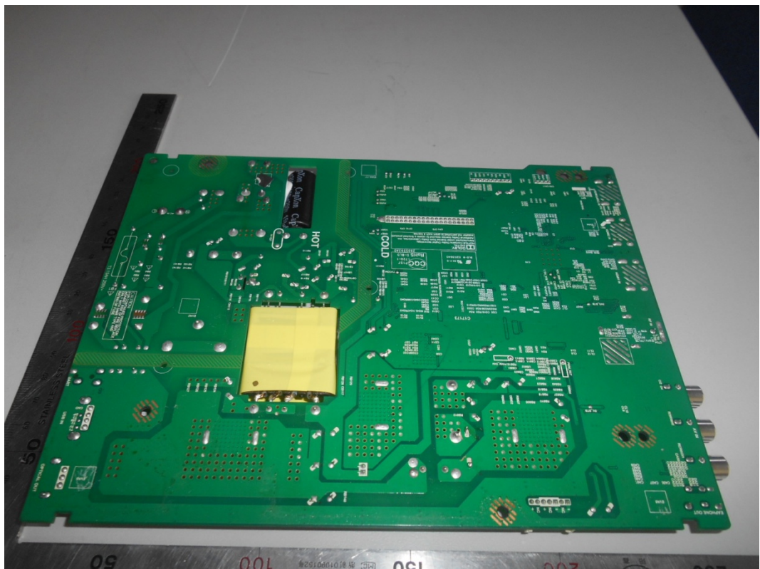
FIGURE 4 LED LCD TV (M/N: LC-32P3000U) MAIN BOARD (SOLDERED SIDE)
