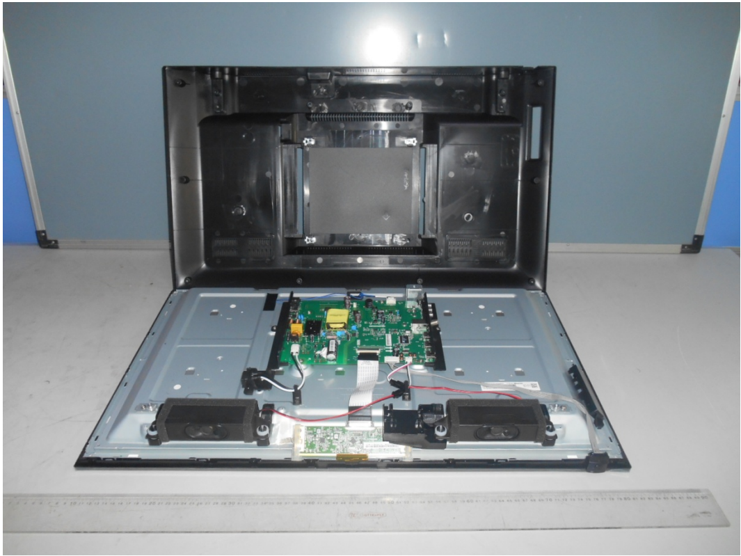
FIGURE 1 LED LCD TV (M/N: LC-32P3000U) COVER REMOVED
