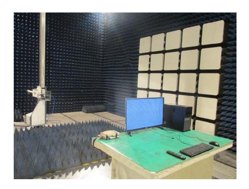
Photos of Radiation Spurious Emission Measurement
