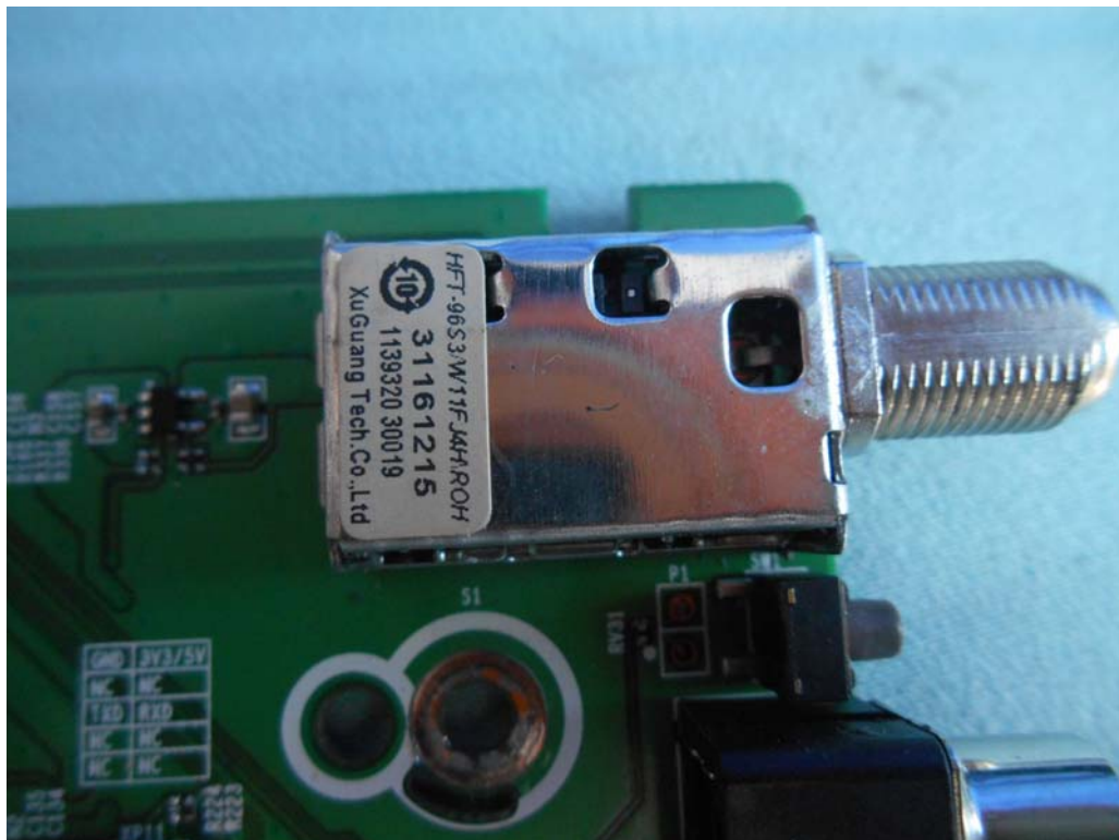
FIGURE 6 LED LCD TV (M/N: 32H4D) TUNER
