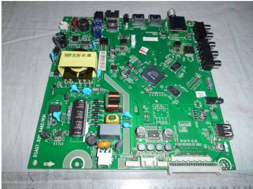
FIGURE 4 LED LCD TV (M/N: LTDN32K220WUS) MAIN BOARD (COMPONENT SIDE)
