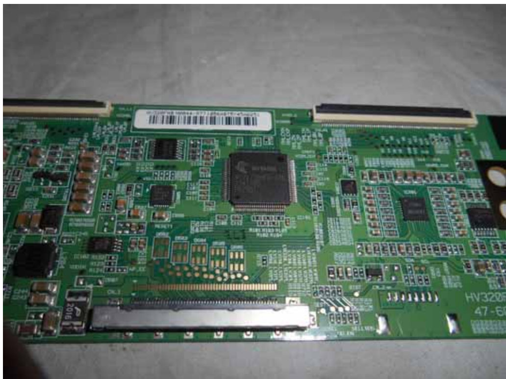
FIGURE 18 LED LCD TV (M/N: LTDN32K220WUS) CHIP ON SIGNAL BOARD
