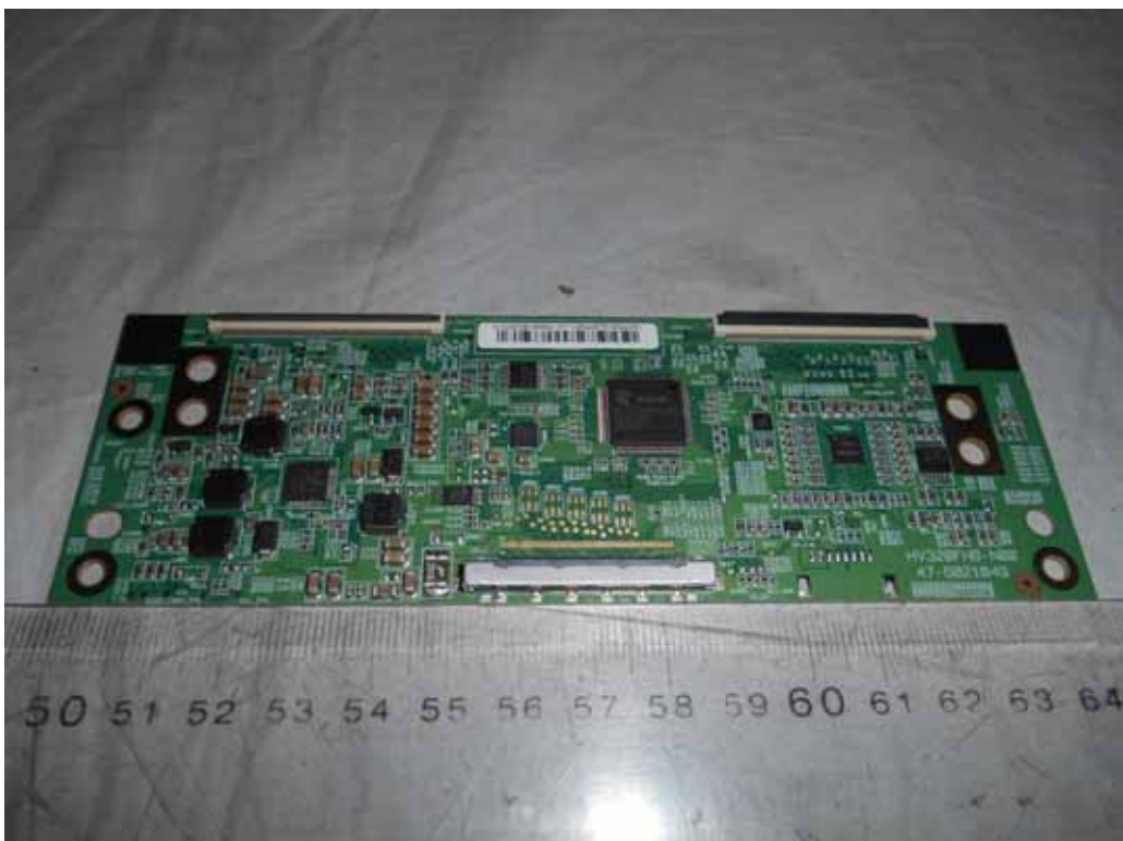
FIGURE 16 LED LCD TV (M/N: LTDN32K220WUS) SIGNAL BOARD (COMPONENT SIDE)
