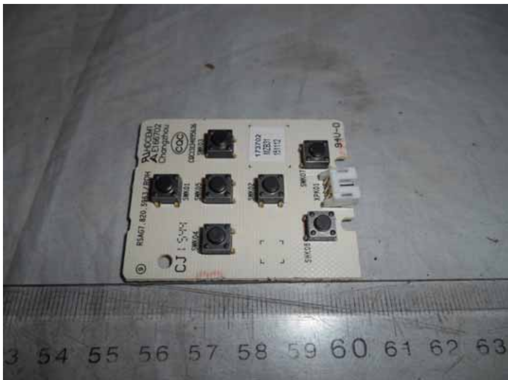
FIGURE 12 LED LCD TV (M/N: LTDN32K220WUS) KEY BOARD (COMPONENT SIDE)
