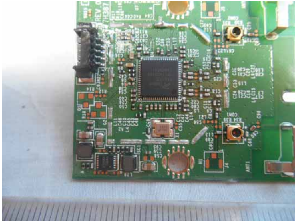
FIGURE 11 LED LCD TV (M/N: LTDN32K220WUS) CHIP & CRYSTAL ON RF BOARD
