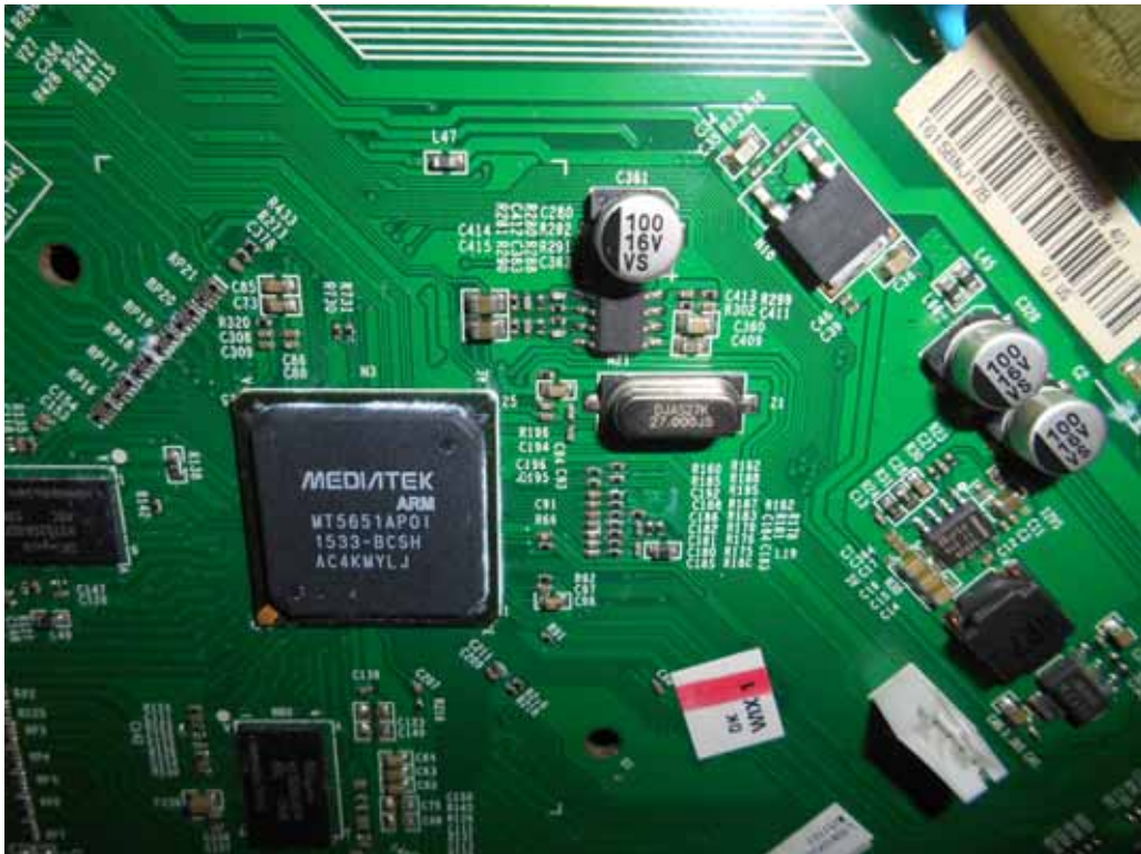
FIGURE 6 LED LCD TV (M/N: LTDN32K220WUS) CHIP & CRYSTAL ON MAIN BOARD
