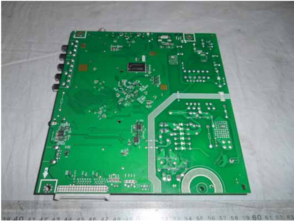
FIGURE 5 LED LCD TV (M/N: LTDN32K220WUS) MAIN BOARD (SOLDERED SIDE)
