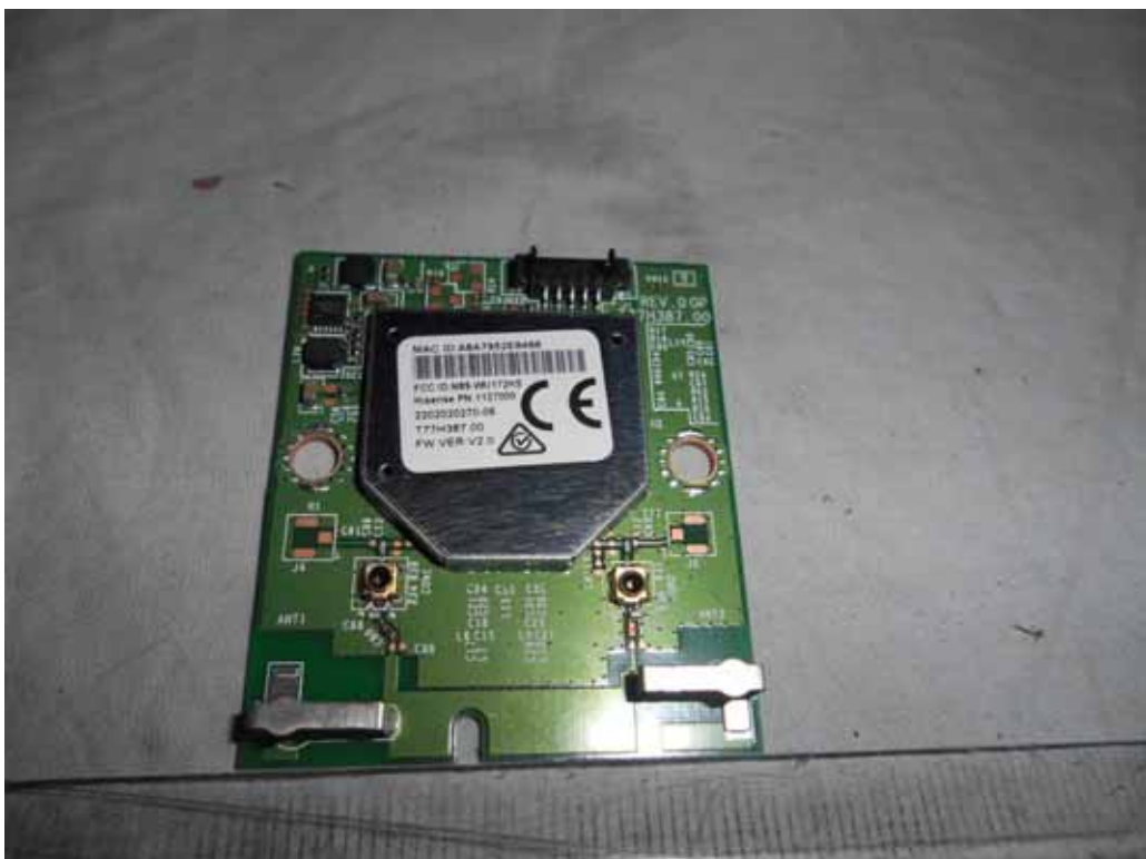
FIGURE 8 LED LCD TV (M/N: LTDN32K220WUS) RF BOARD (COMPONENT SIDE)
