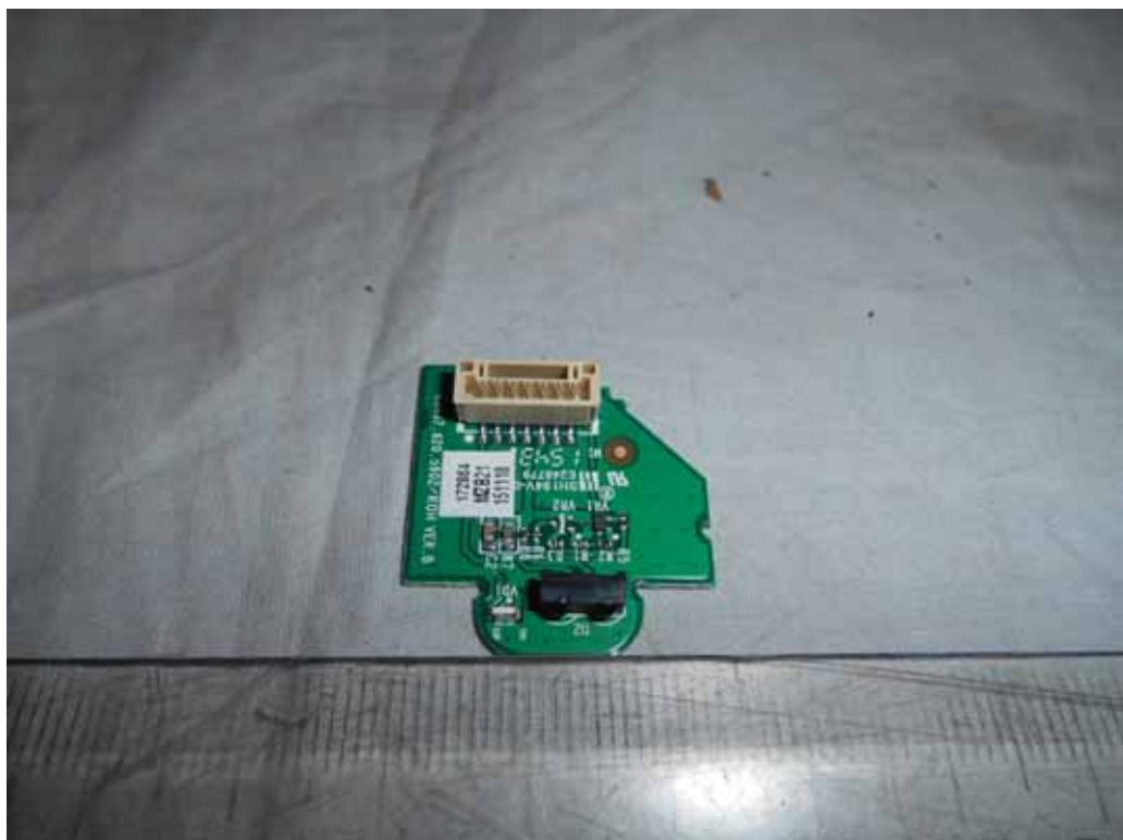
FIGURE 14 LED LCD TV (M/N: LTDN32K220WUS) IR BOARD (COMPONENT SIDE)
