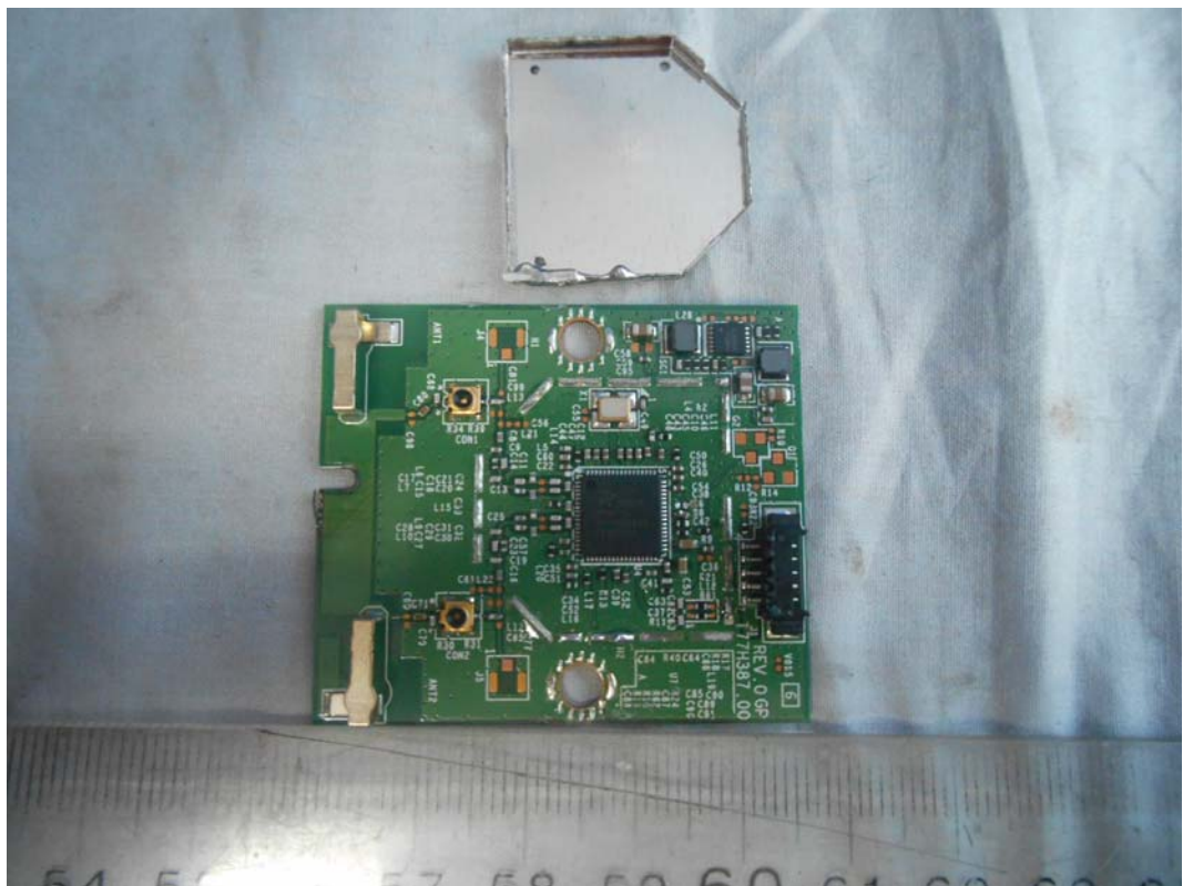
FIGURE 18 LED LCD TV (M/N: LHD32K220WUS) RF BOARD COVER REMOVED
