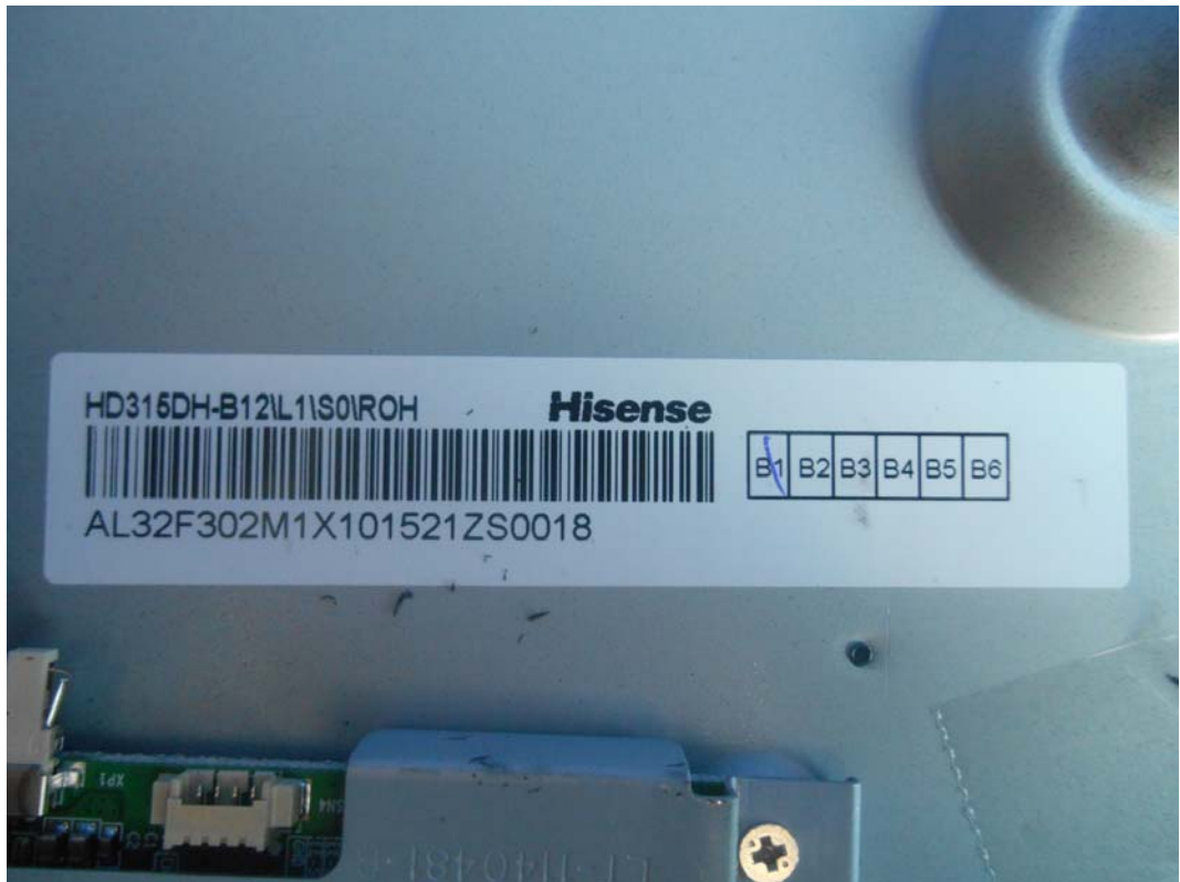
FIGURE 3 LED LCD TV (M/N: LHD32K220WUS) LCD PANEL LABEL
