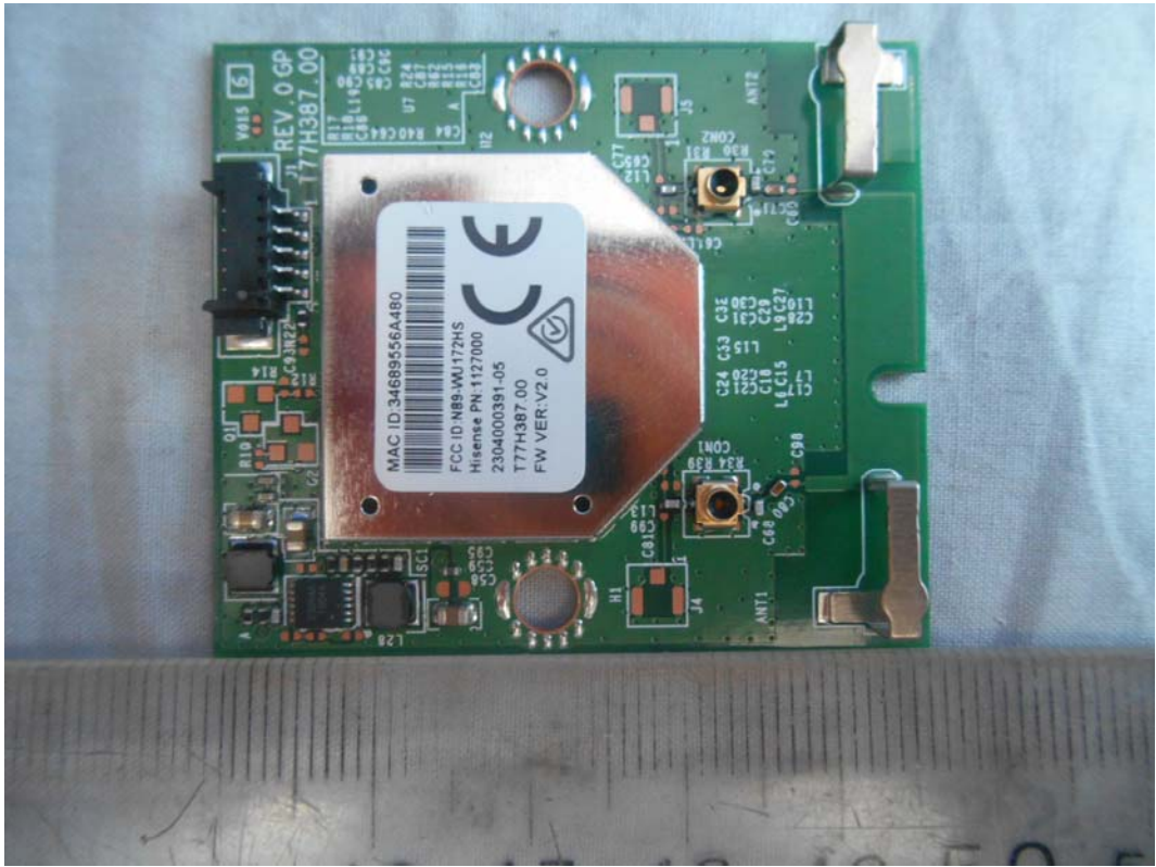
FIGURE 15 LED LCD TV (M/N: LHD32K220WUS) RF BOARD (COMPONENT SIDE)
