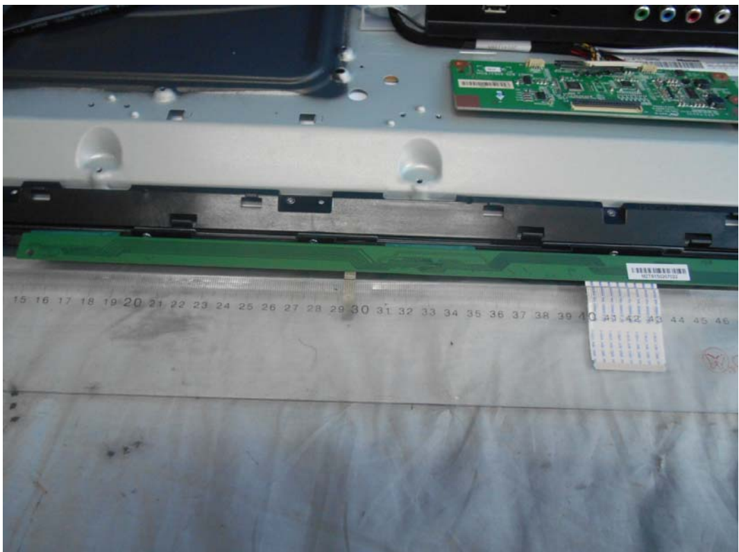
FIGURE 25 LED LCD TV (M/N: LHD32K220WUS) CONTROL BOARD #2 (COMPONENT SIDE)
