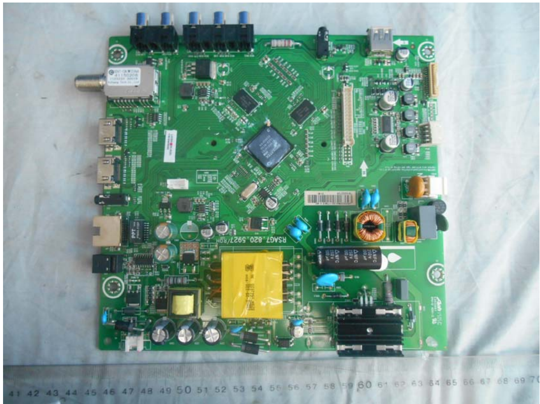
FIGURE 5 LED LCD TV (M/N: LHD32K220WUS) MAIN BOARD (COMPONENT SIDE)
