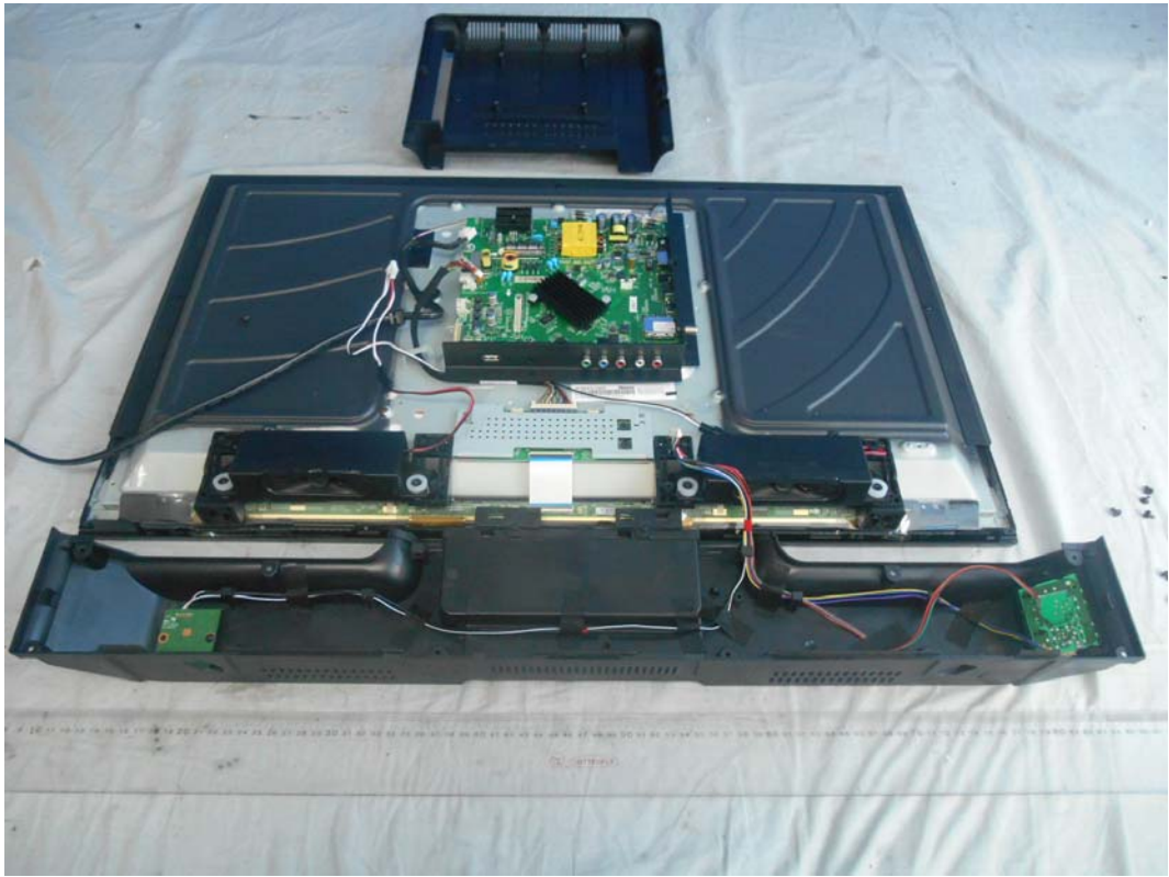
FIGURE 1 LED LCD TV (M/N: LHD32K220WUS) COVER REMOVED #1
