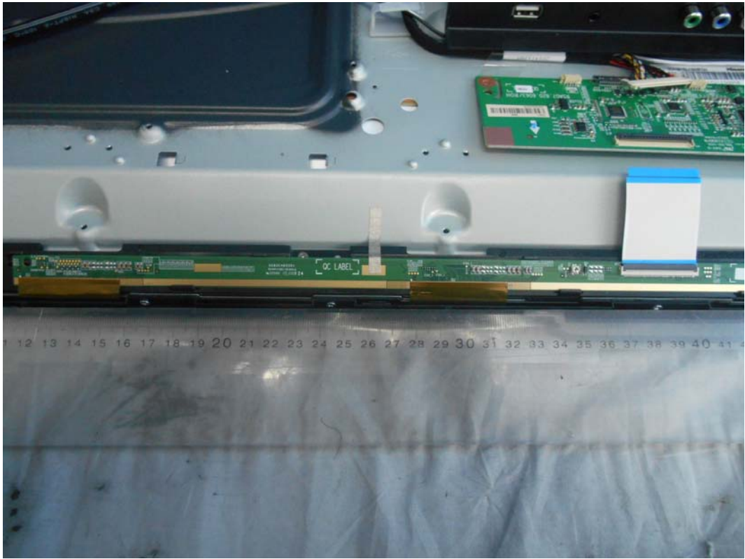
FIGURE 24 LED LCD TV (M/N: LHD32K220WUS) CONTROL BOARD #1 (COMPONENT SIDE)
