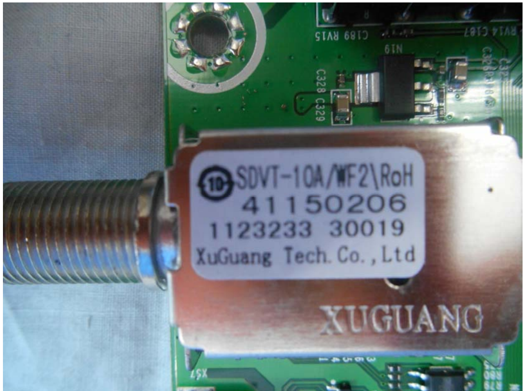
FIGURE 11 LED LCD TV (M/N: LHD32K220WUS) TUNER LABEL
