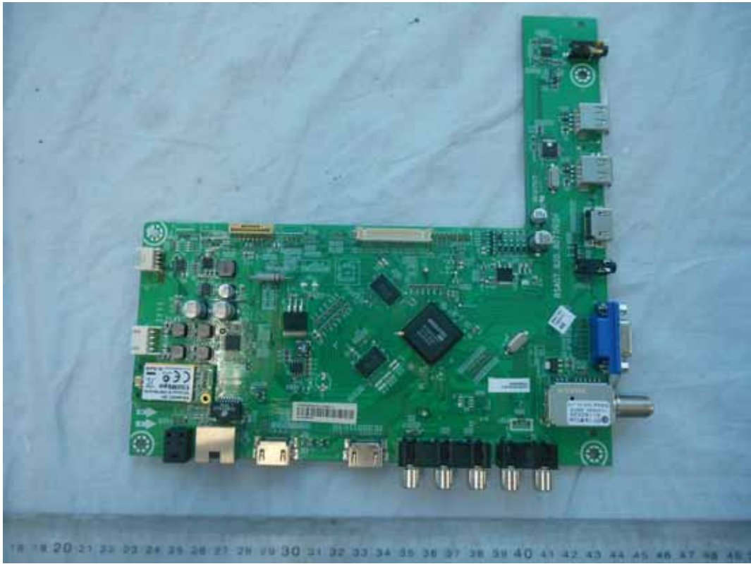
FIGURE 5 LED LCD TV (M/N: 32K20DW) MAIN BOARD (COMPONENT SIDE)
