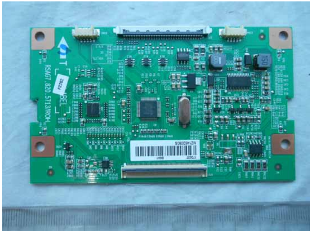
FIGURE 14 LED LCD TV (M/N: 32K20DW) LCD PANEL CONTROL BOARD (COMPONENT SIDE)
