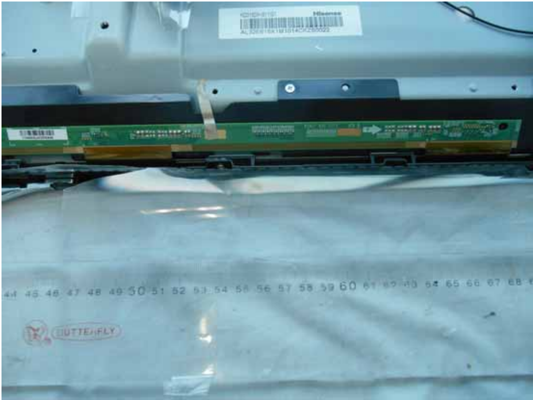
FIGURE 18 LED LCD TV (M/N: 32K20DW) LCD PANEL CONTROL BOARD (COMPONENT SIDE #2)
