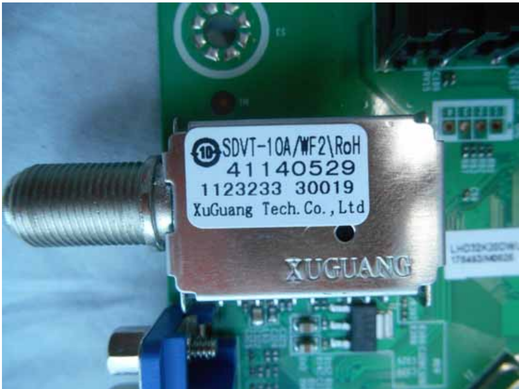
FIGURE 9 LED LCD TV (M/N: 32K20DW) TUNER ON MAIN BOARD
