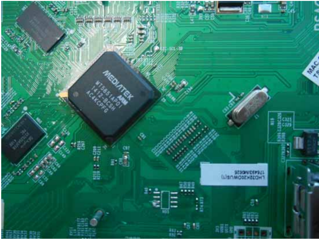
FIGURE 7 LED LCD TV (M/N: 32K20DW) CRYSTAL & CHIP #1 ON MAIN BOARD
