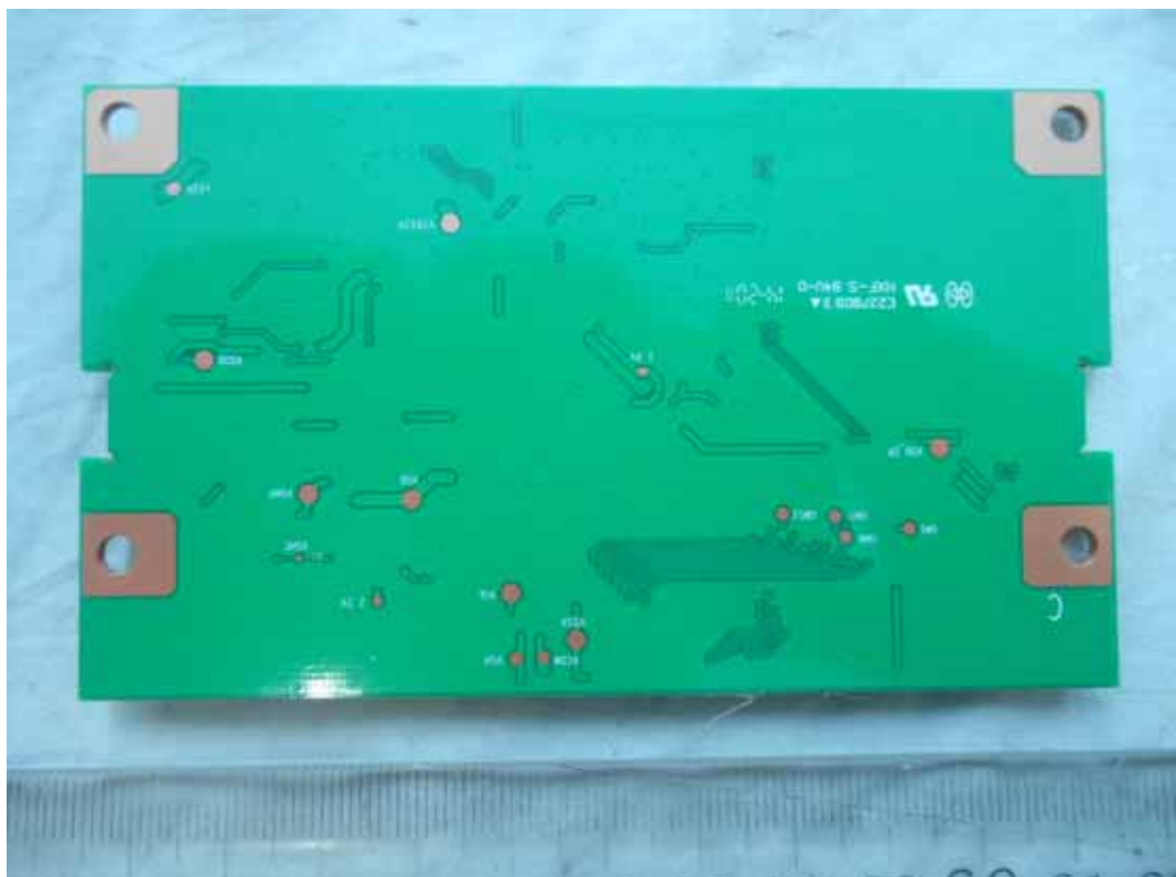
FIGURE 15 LED LCD TV (M/N: 32K20DW) LCD PANEL CONTROL BOARD (SOLDERED SIDE)
