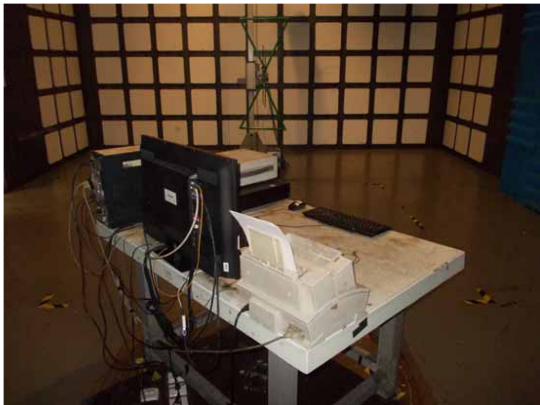
SETUP WITH MAXIMUM DETECTED EMISSION AT VERTICAL POLARIZATION (TEST MODE: HDMI 1920*1080@60Hz)
