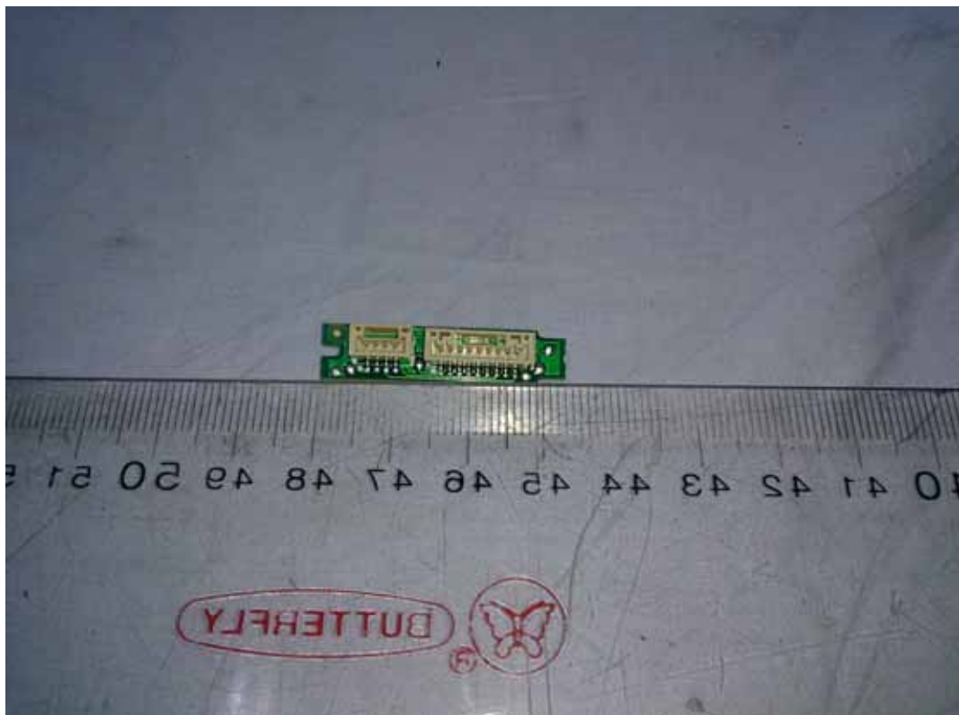
FIGURE 12 LED LCD TV (M/N: 32K20D) IR BOARD (SOLDERED SIDE)
