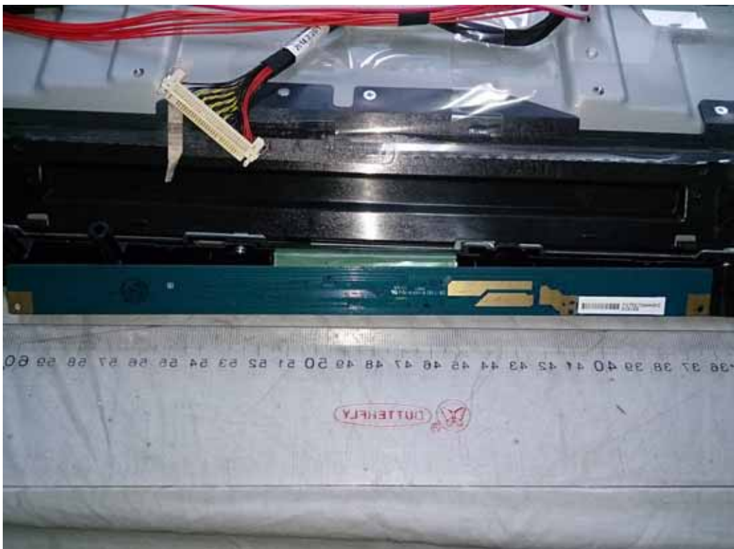
FIGURE 14 LED LCD TV (M/N: 32K20D) LCD PANEL CONTROL BOARD (SOLDERED SIDE)
