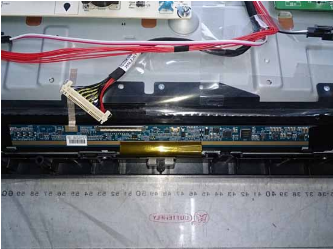
FIGURE 13 LED LCD TV (M/N: 32K20D) LCD PANEL CONTROL BOARD (COMPONENT SIDE)
