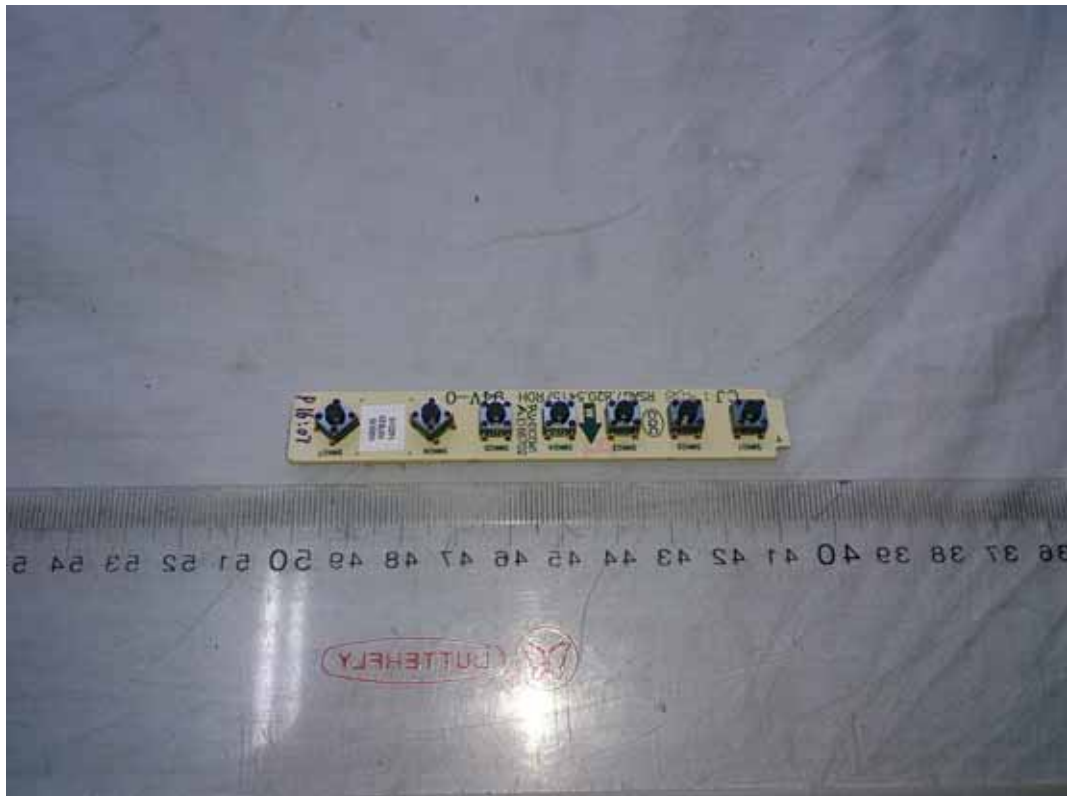
FIGURE 9 LED LCD TV (M/N: 32K20D) KEY BOARD (COMPONENT SIDE)
