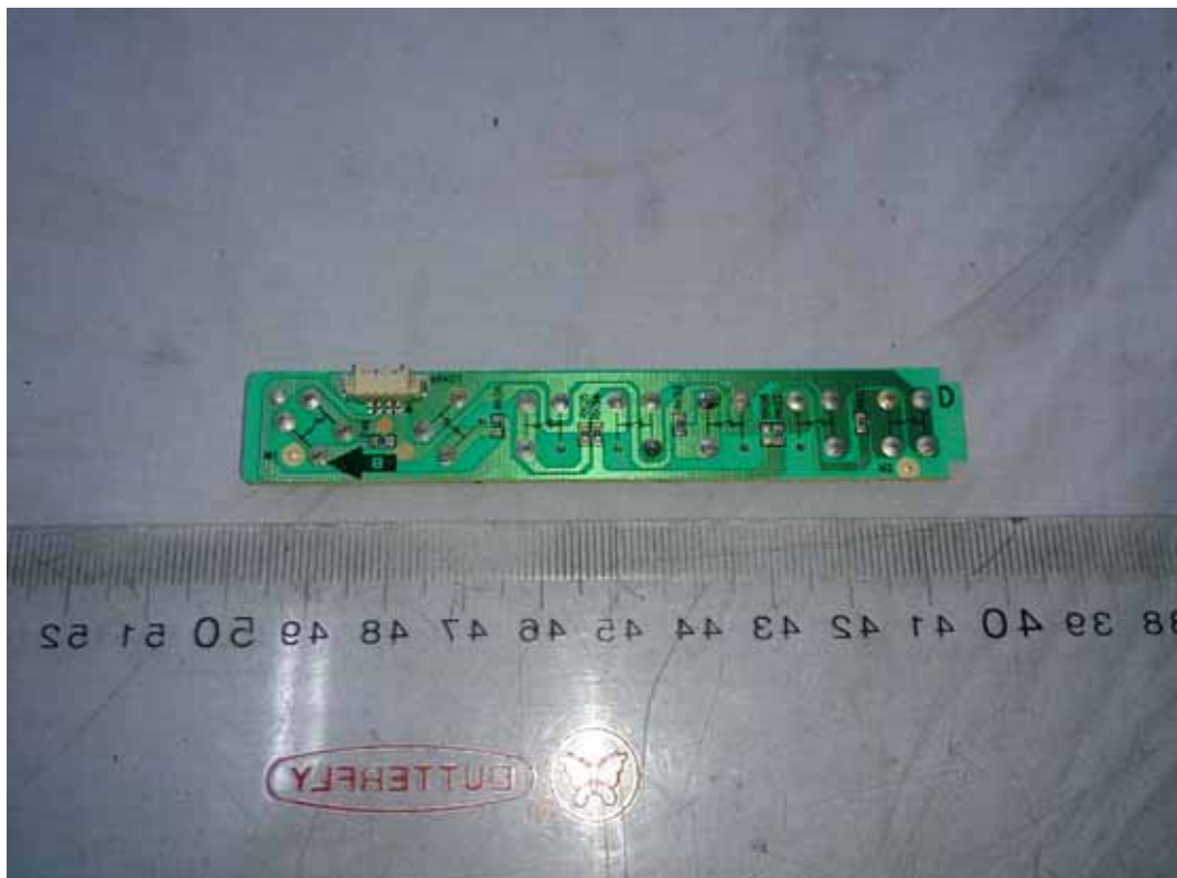
FIGURE 10 LED LCD TV (M/N: 32K20D) KEY BOARD (SOLDERED SIDE)
