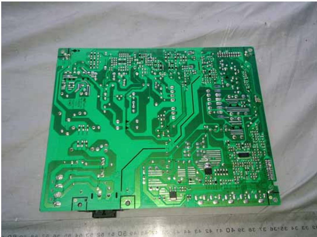
FIGURE 4 LED LCD TV (M/N: 32K20D) POWER BOARD (SOLDERED SIDE)
