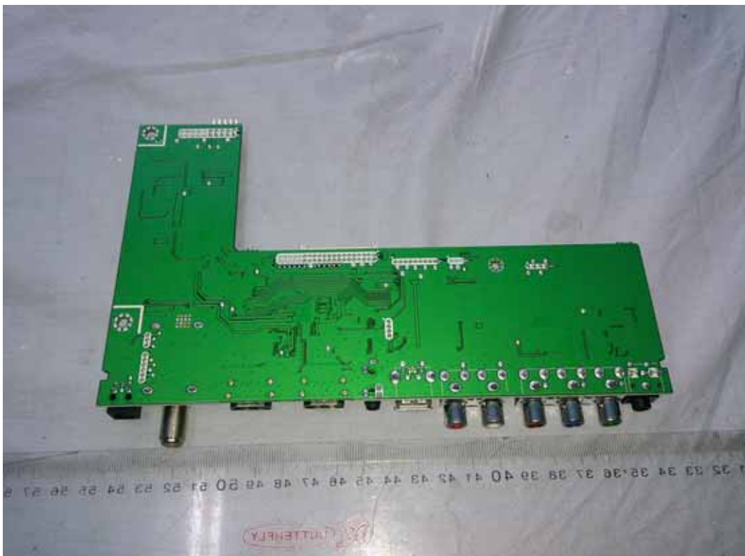
FIGURE 6 LED LCD TV (M/N: 32K20D) MAIN BOARD (SOLDERED SIDE)
