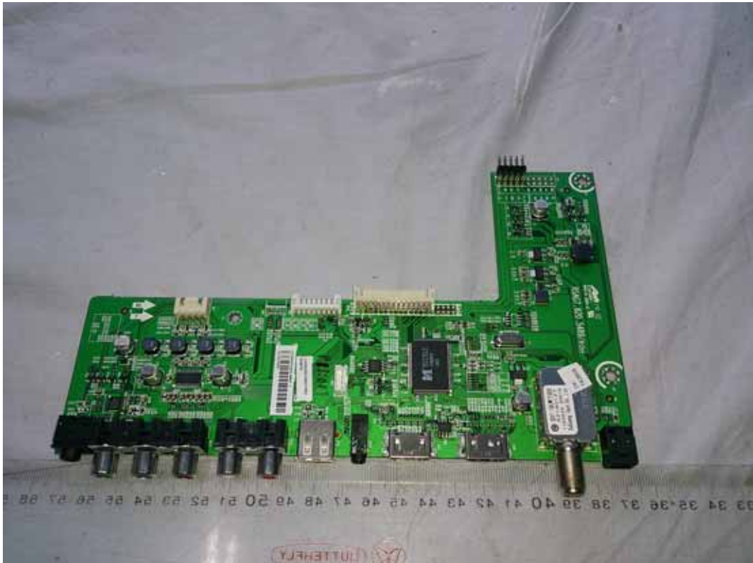
FIGURE 5 LED LCD TV (M/N: 32K20D) MAIN BOARD (COMPONENT SIDE)
