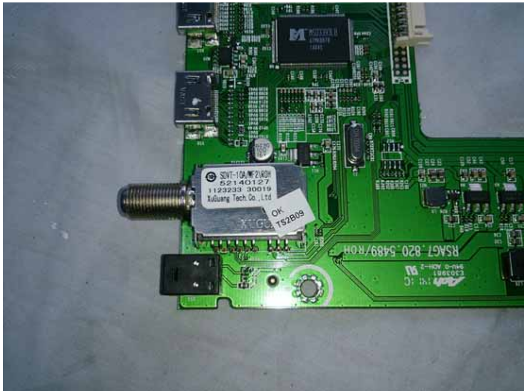
FIGURE 7 LED LCD TV (M/N: 32K20D) TUNER ON MAIN BOARD
