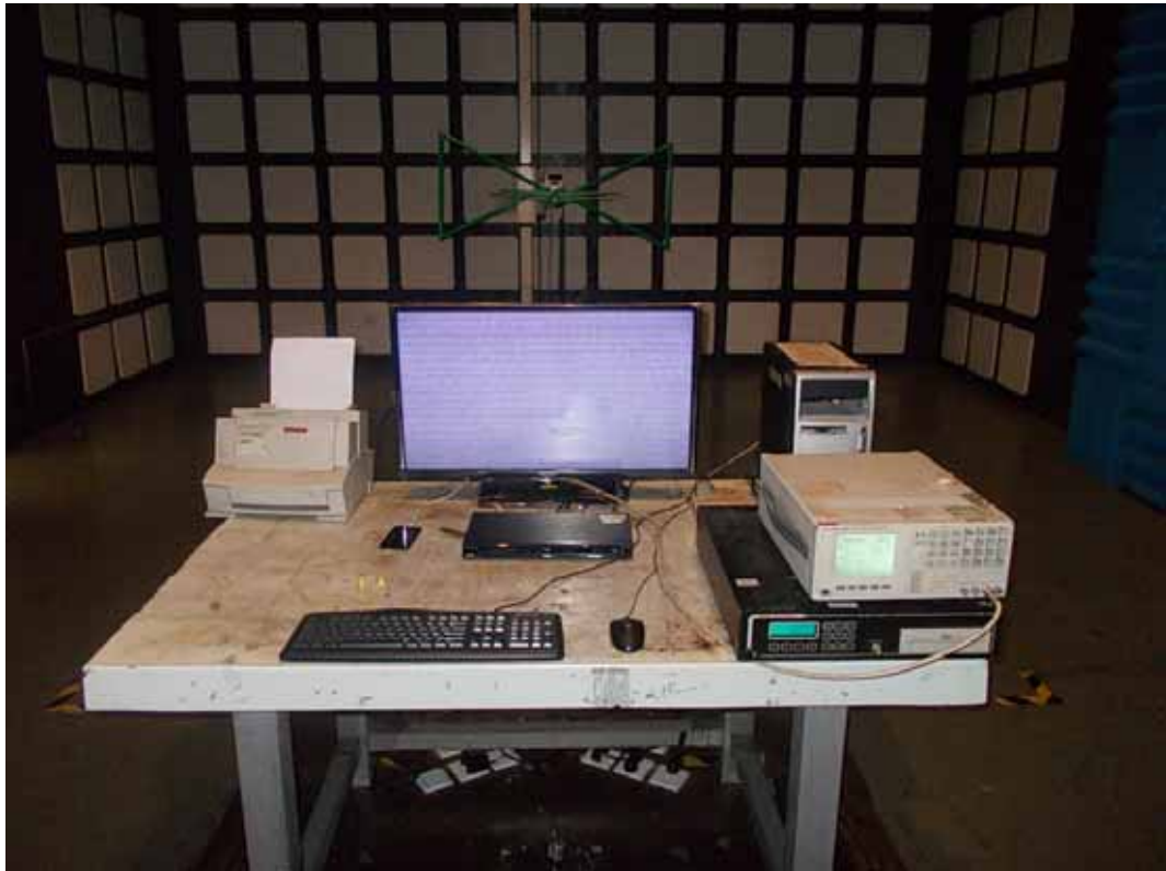
FRONT VIEW OF RADIATED EMISSION TEST
