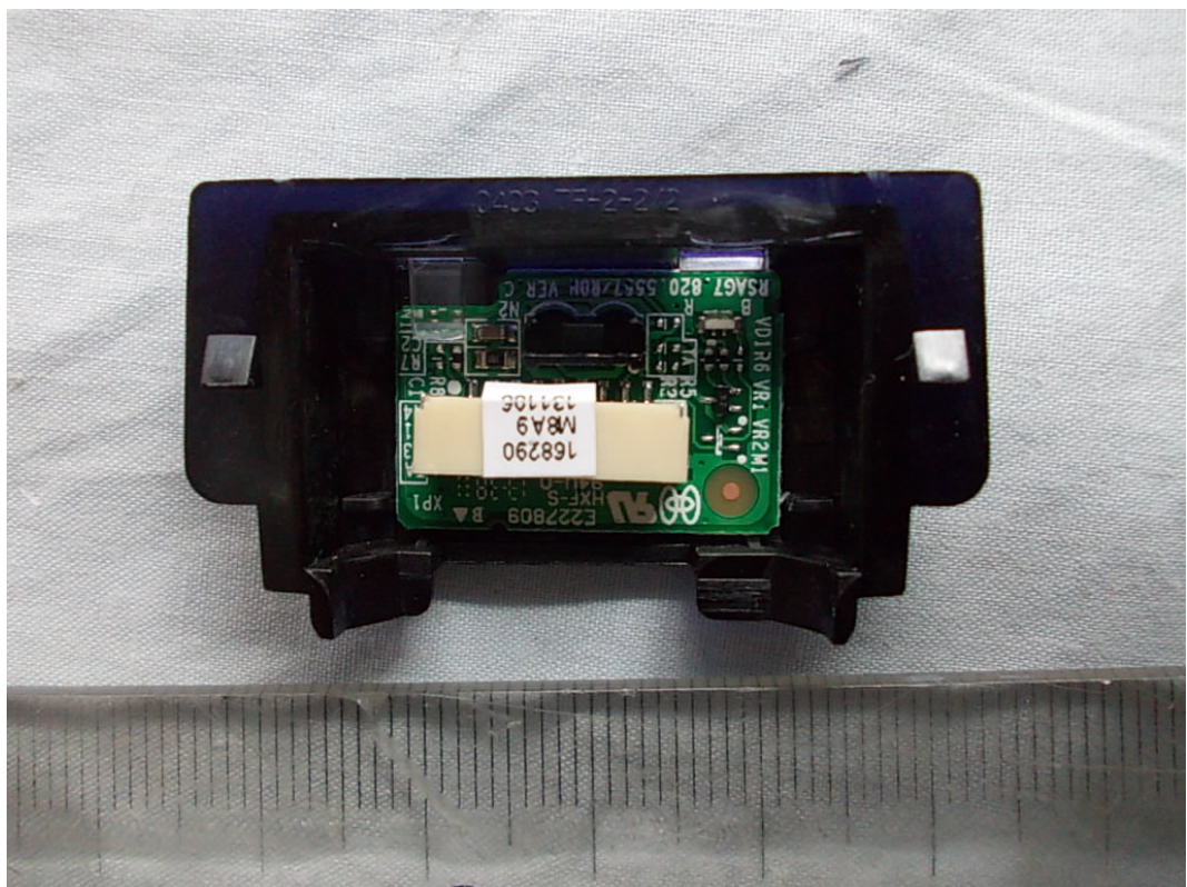
FIGURE 10 LED LCD TV (M/N: 32K20D) IR BOARD
